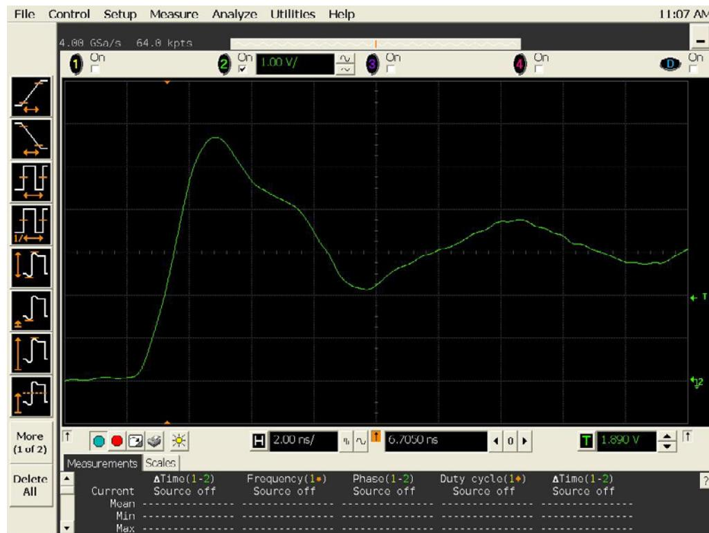
Figure 11a DUT 19742 Pre-Radiation Rising Edge
