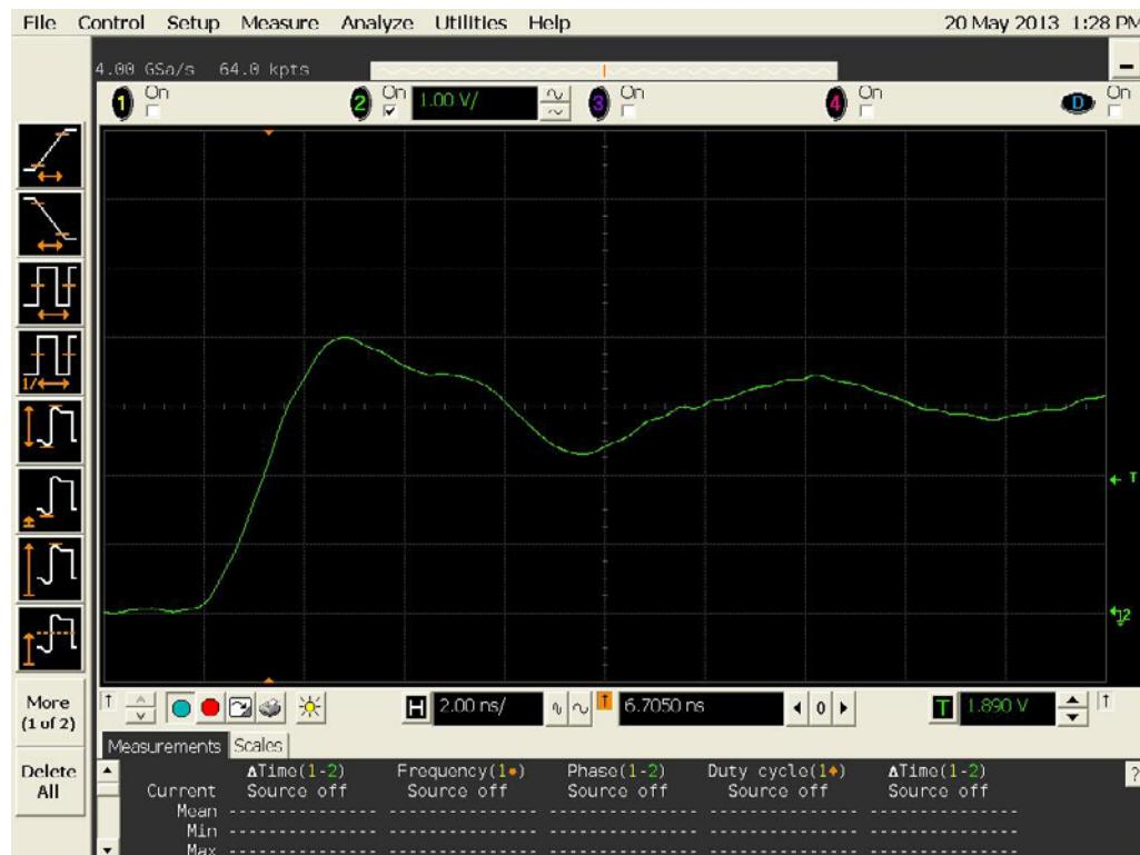
Figure 11b DUT 19742 Post-Annealing Rising edge
