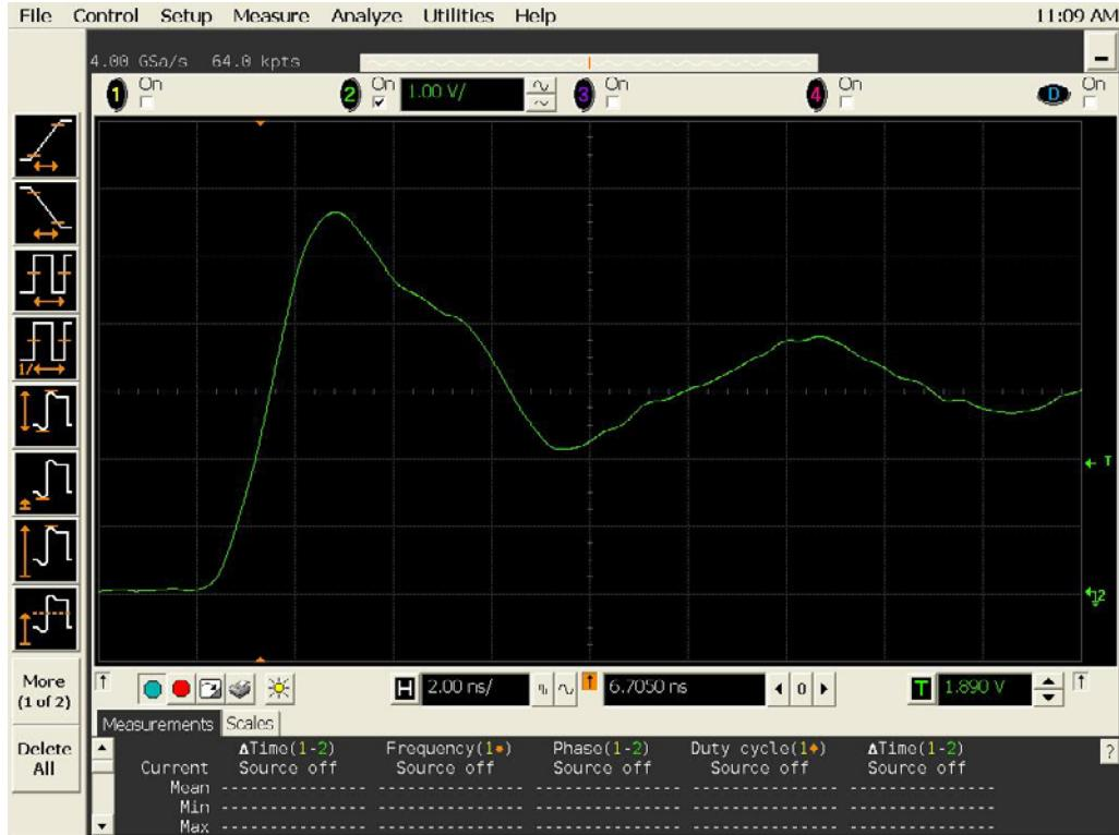
Figure 10a DUT 19740 Pre-Irradiation Rising Edge
