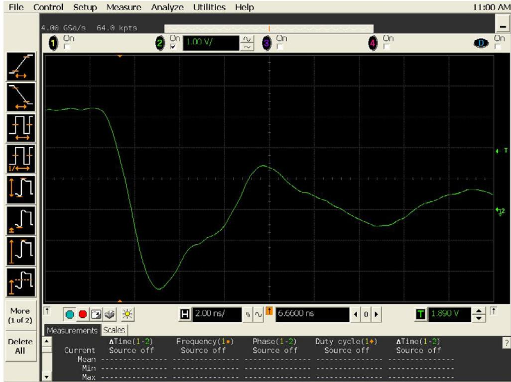
Figure 15a DUT 19739 Pre-Radiation Falling Edge
