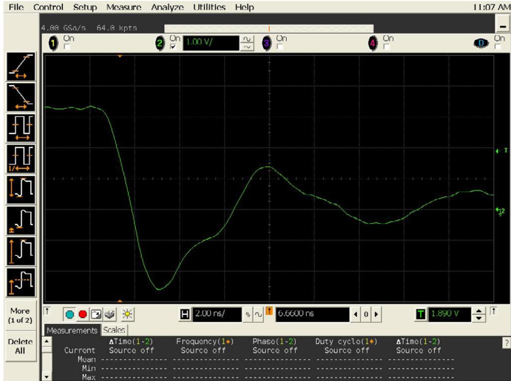
Figure 17a DUT 19742 Pre-Irradiation Falling Edge
