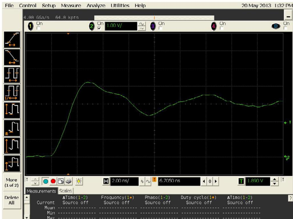
Figure 12b DUT 19743 Post-Annealing Rising Edge
