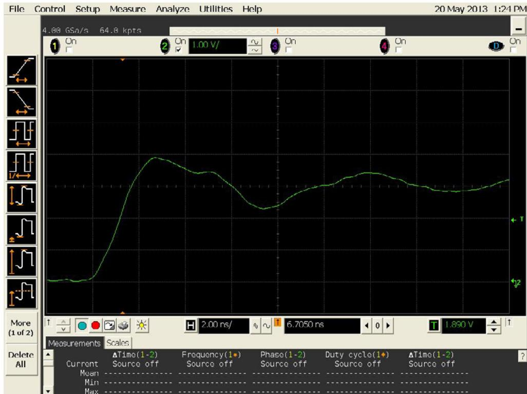
Figure 10b DUT 19740 Post-Annealing Rising Edge
