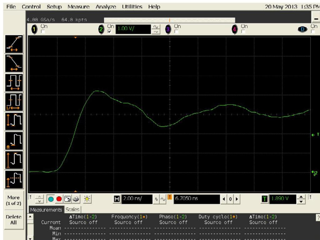
Figure 13b DUT 19759 Post-Annealing Rising Edge
