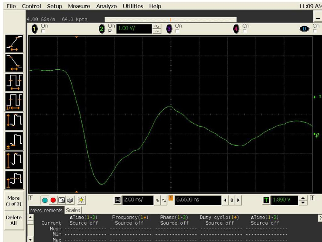
Figure 16a DUT 19740 Pre-Irradiation Falling Edge
