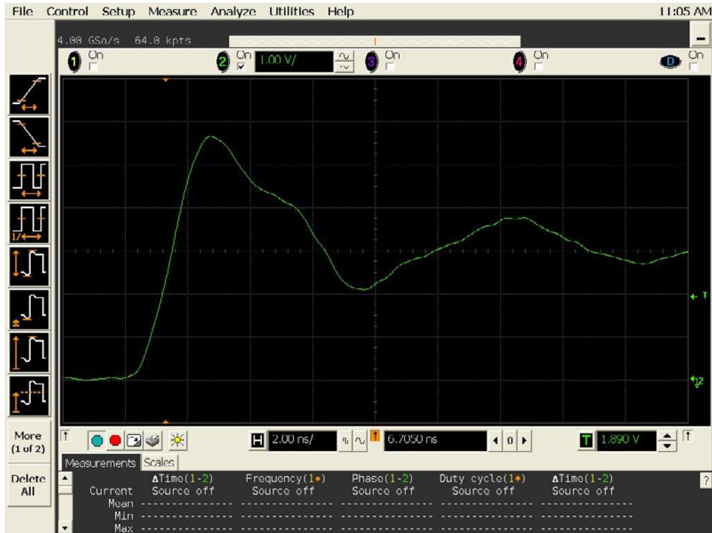
Figure 12a DUT 19743 Pre-Irradiation Rising Edge
