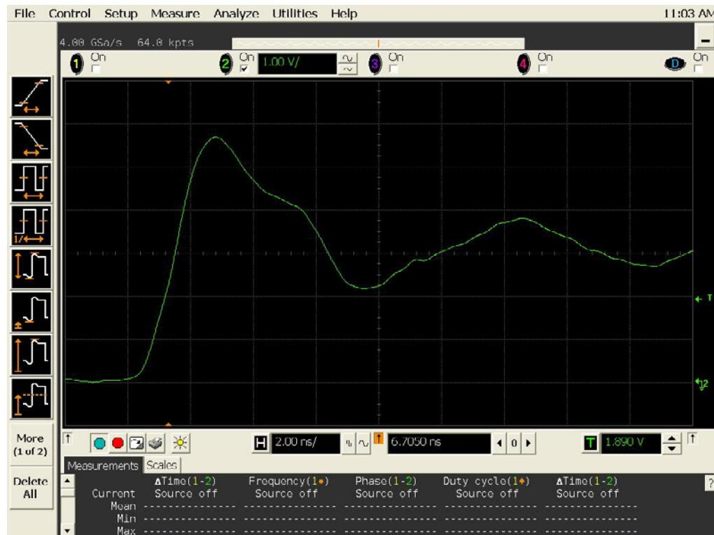
Figure 13a DUT 19759 Pre-Irradiation Rising Edge
