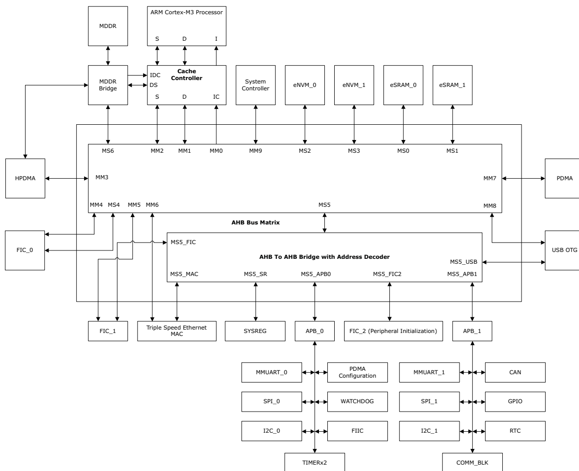
Figure 1 • SmartFusion2 - System Controller Interfacing with AHB Bus Matrix
