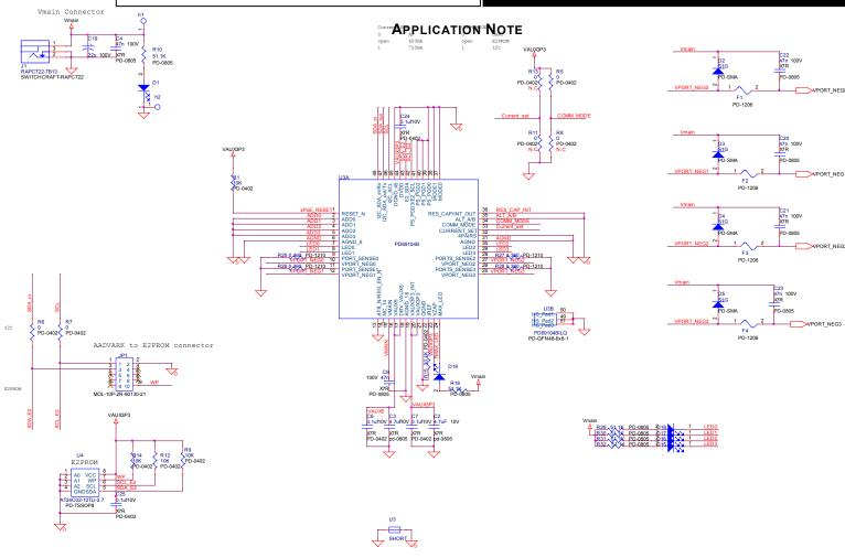
Figure 1: 4 Ports Auto Mode Circuit
