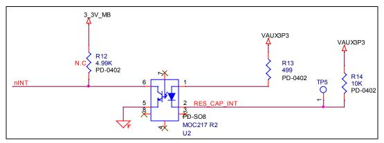
Figure 3: Interrupt Isolation Circuitry
