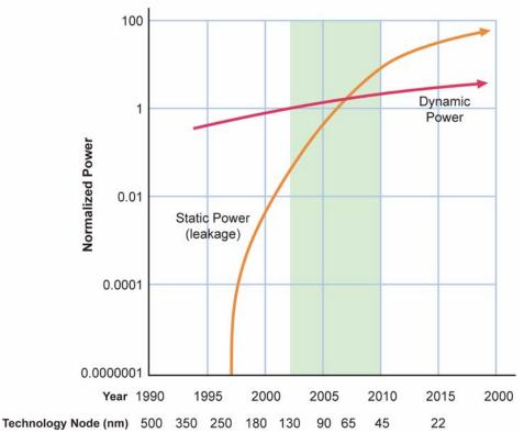
Figure 1: Static Power Significant at 90 nm
