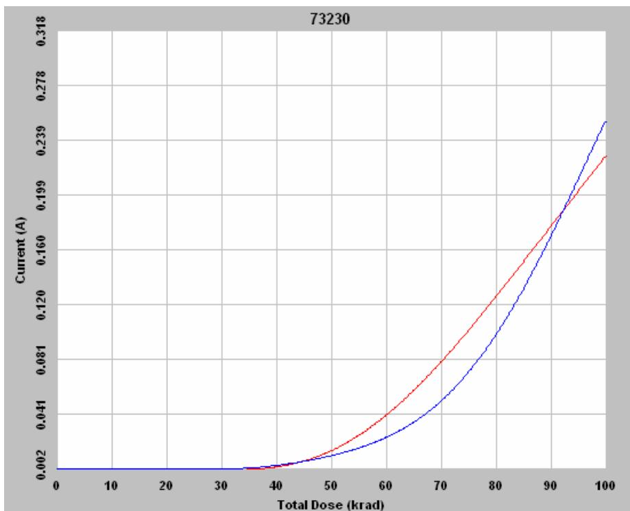
Figure 2 DUT 73230 in-flux  $I_{CCA}$  and  $I_{CCI}$ ; blue line is  $I_{CCA}$ , and red line  $I_{CCI}$ .
