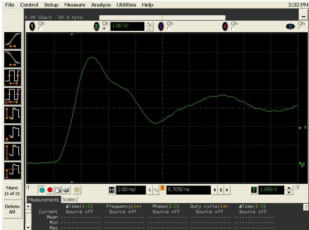
Figure 12a DUT 19712 Pre-Irradiation Rising Edge
