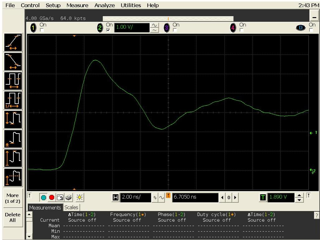
Figure 10a DUT 19683 Pre-Irradiation Rising Edge
