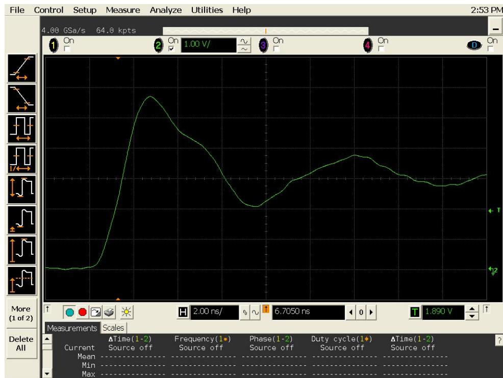
Figure 9a DUT 19665 Pre-Irradiation Rising Edge
