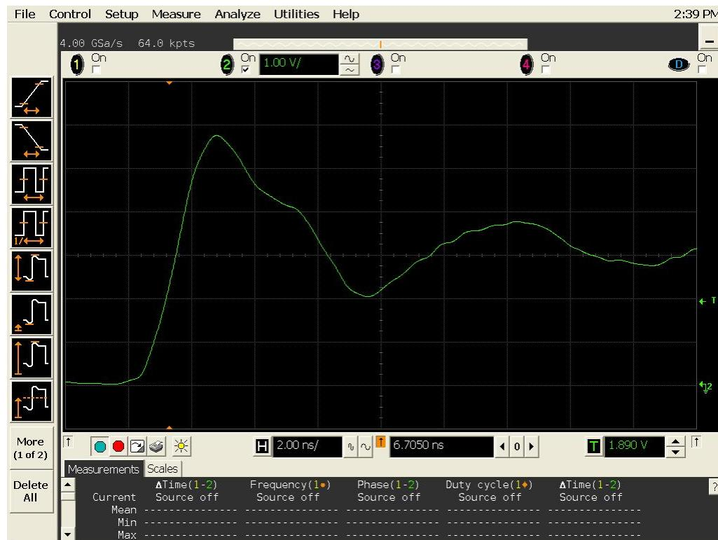
Figure 11a DUT 19701 Pre-Radiation Rising Edge
