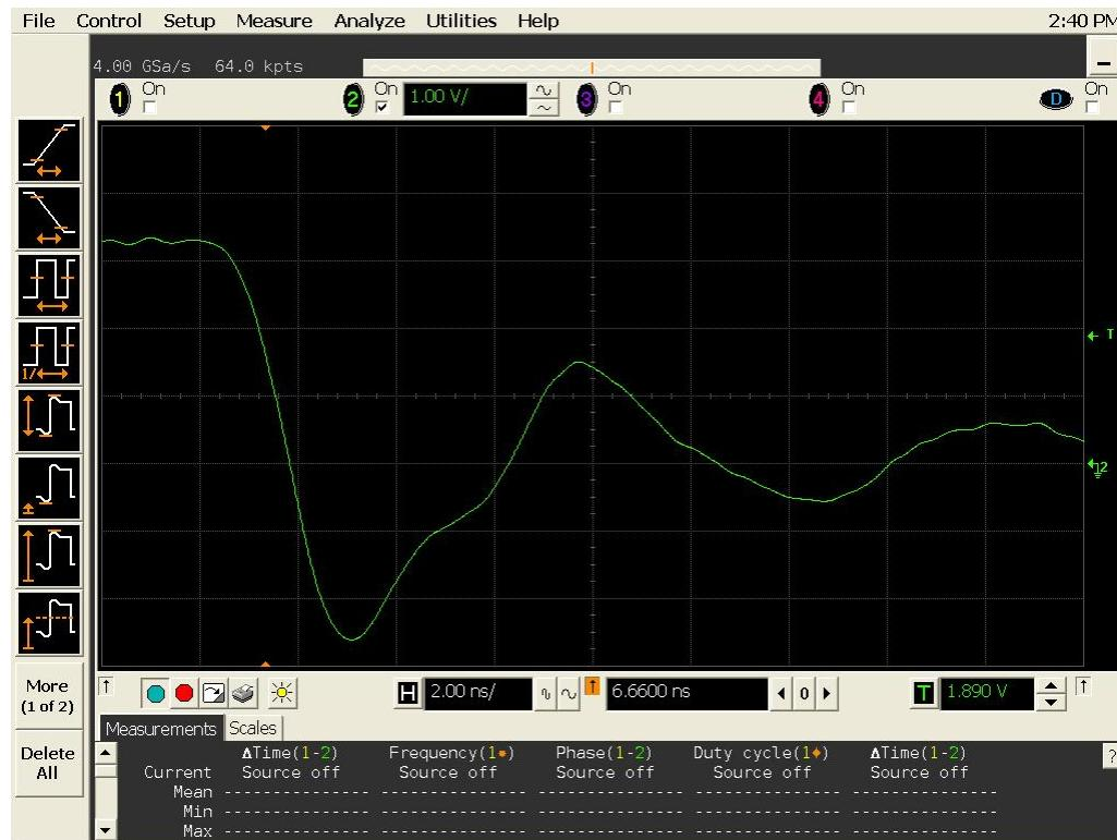
Figure 17a DUT 19701 Pre-Irradiation Falling Edge
