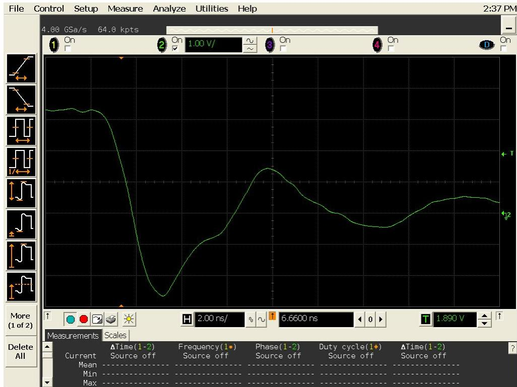
Figure 20a DUT 19723 Pre-Irradiation Falling Edge
