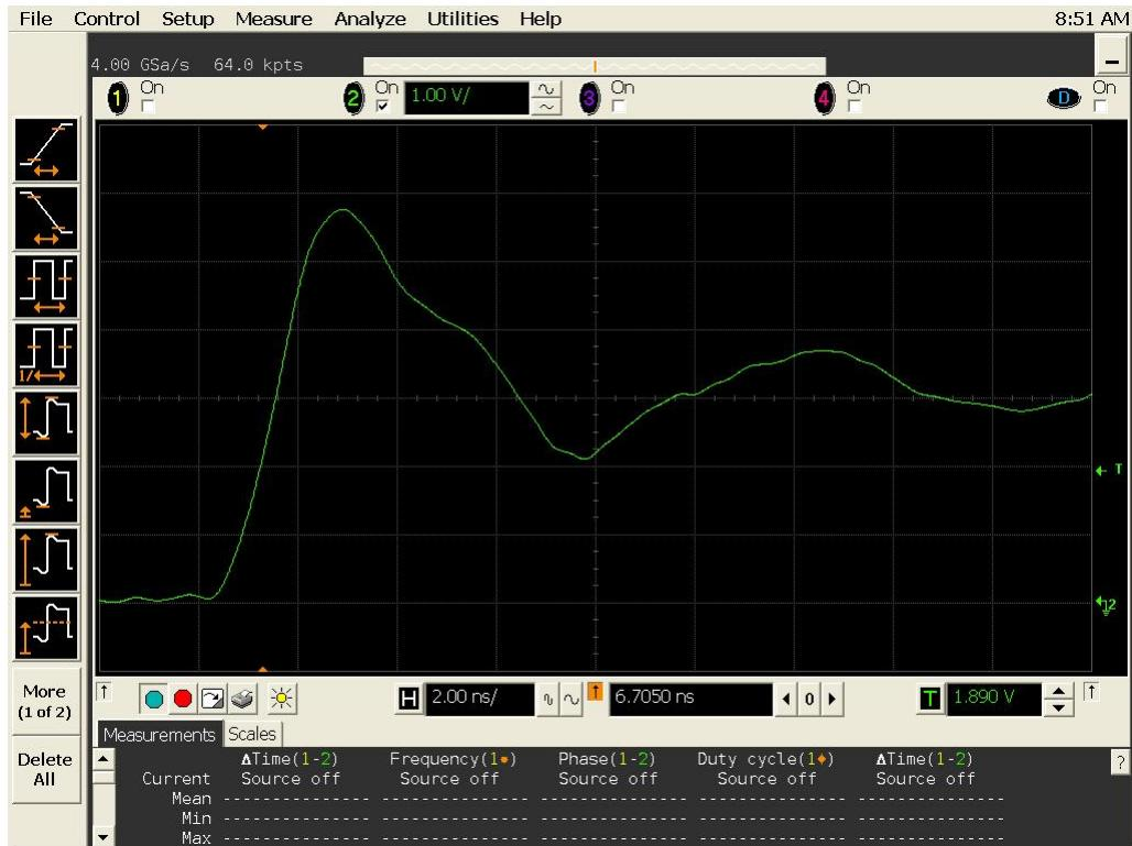
Figure 10b DUT 19683 Post-Annealing Rising Edge
