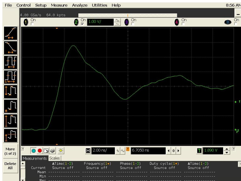
Figure 11b DUT 19701 Post-Annealing Rising edge
