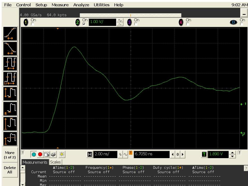
Figure 14b DUT 19723 Post-Annealing Rising Edge
