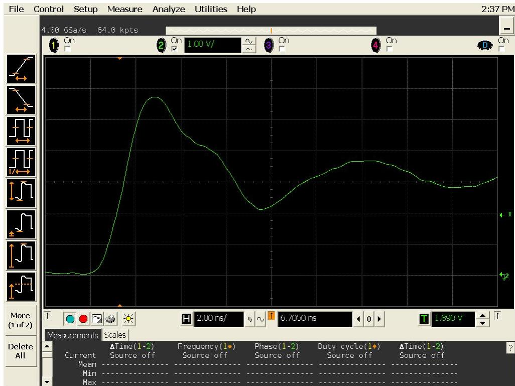
Figure 14a DUT 19723 Pre-Irradiation Rising Edge
