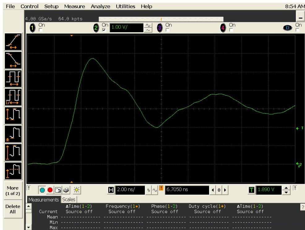
Figure 9b DUT 19665 Post-Annealing Rising Edge
