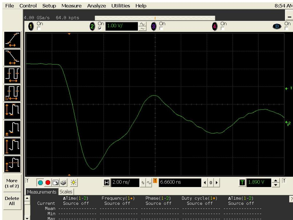
Figure 15b DUT 19665 Post-Annealing Falling Edge
