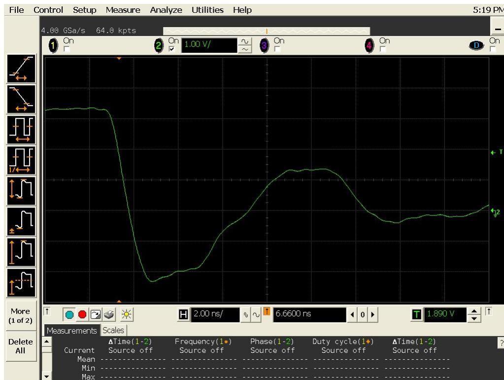
Figure 19b DUT 702 Post-Annealing Falling Edge
