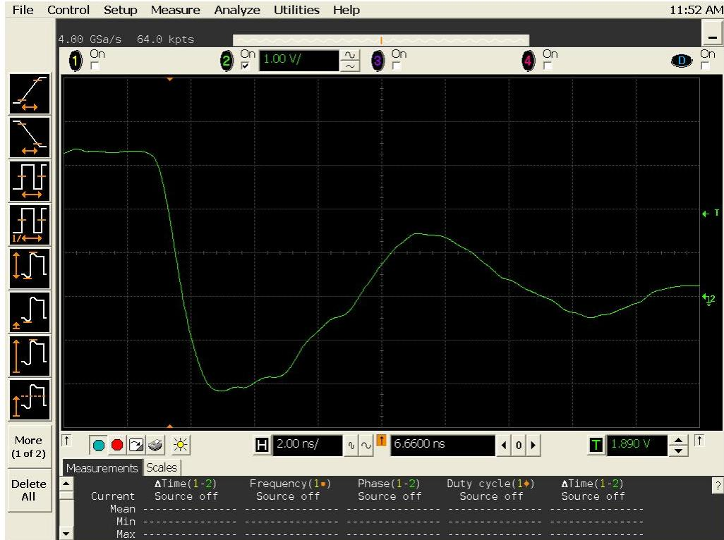
Figure 18a DUT 701 Pre-Irradiation Falling Edge
