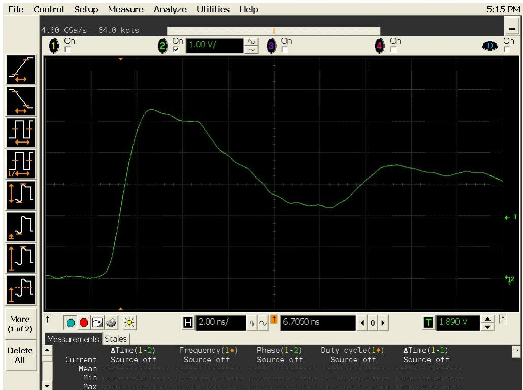
Figure 12b DUT 701 Post-Annealing Rising Edge
