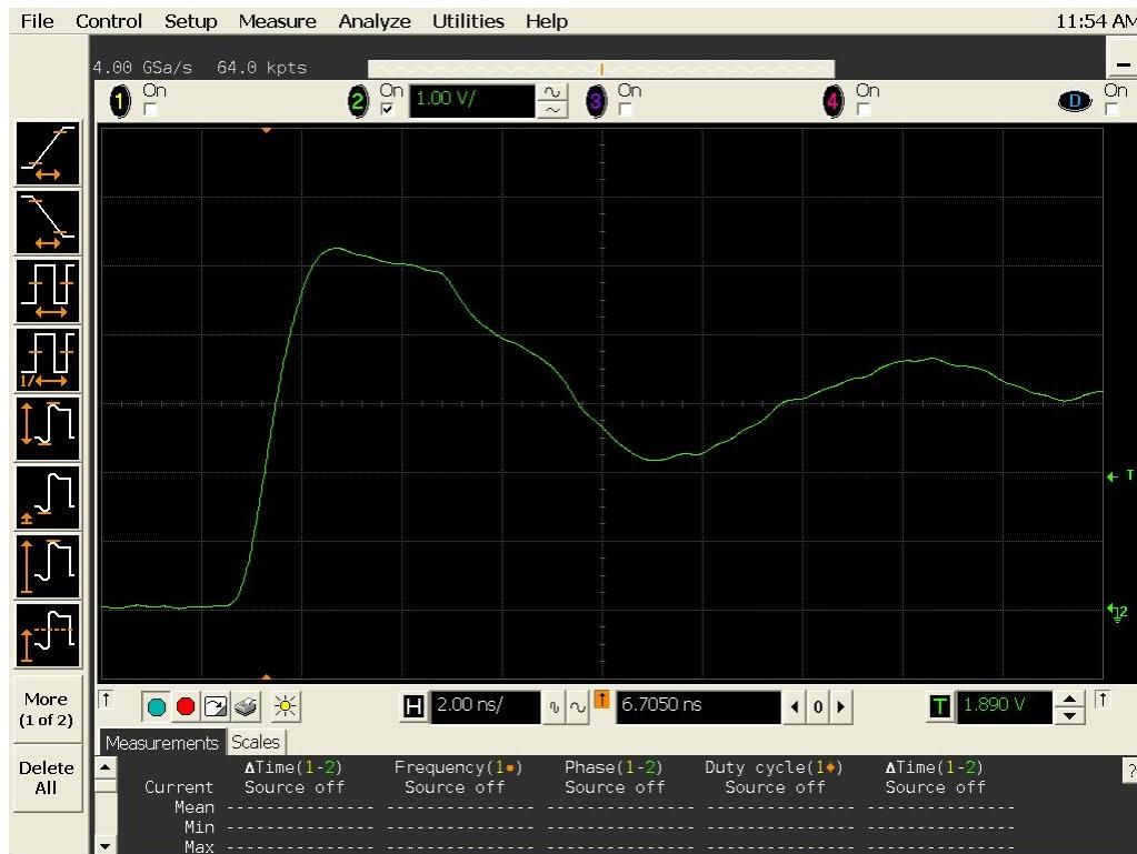
Figure 13a DUT 702 Pre-Irradiation Rising Edge
