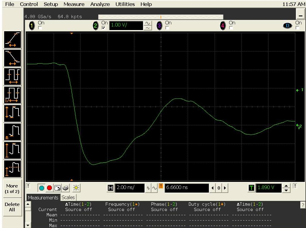
Figure 20a DUT 706 Pre-Irradiation Falling Edge
