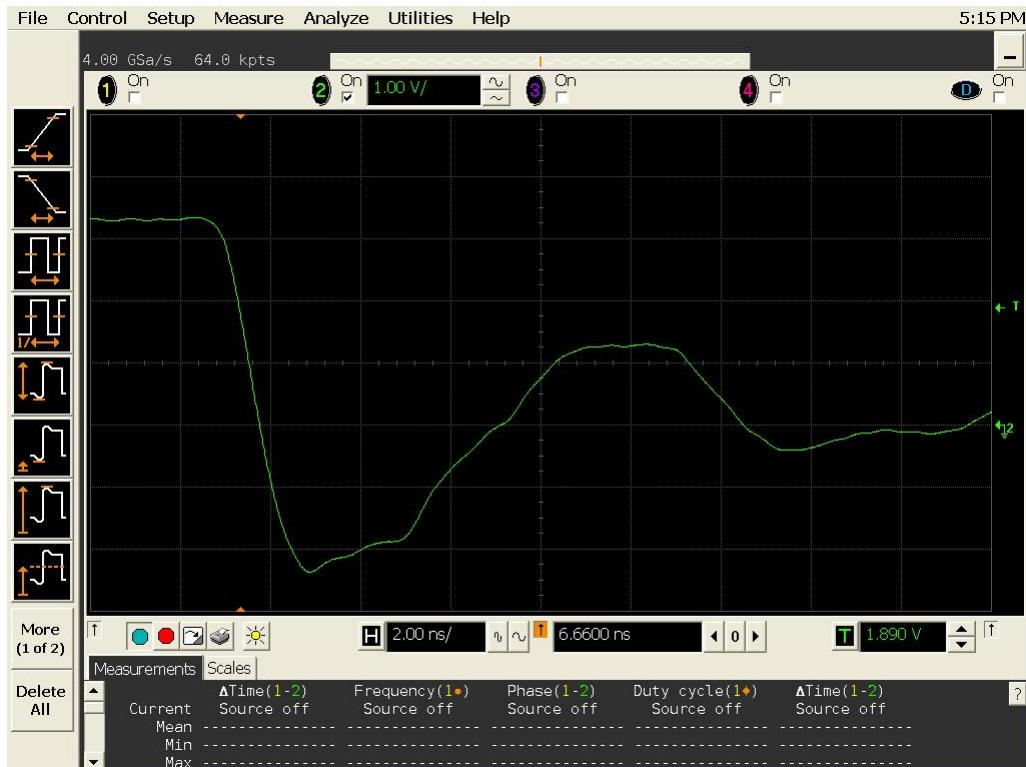
Figure 18b DUT 701 Post-Annealing Falling Edge
