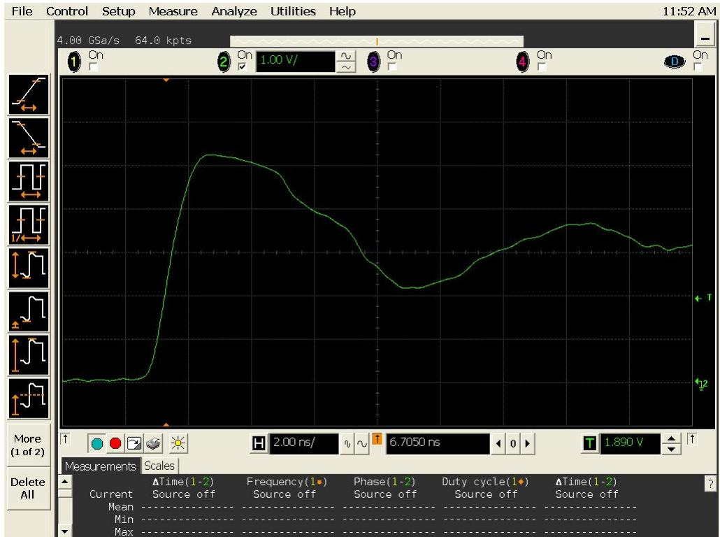
Figure 12a DUT 701 Pre-Irradiation Rising Edge
