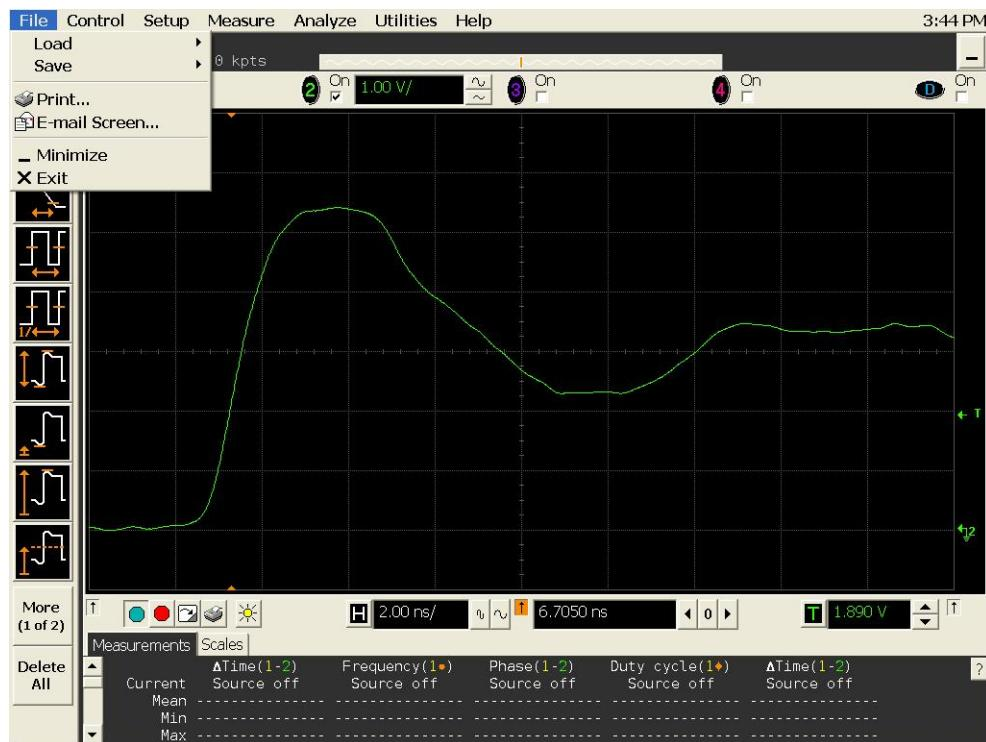
Figure 9b DUT 680 Post-Annealing Rising Edge
