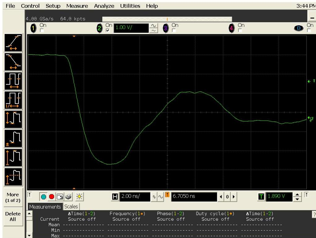
Figure 15b DUT 680 Post-Annealing Falling Edge
