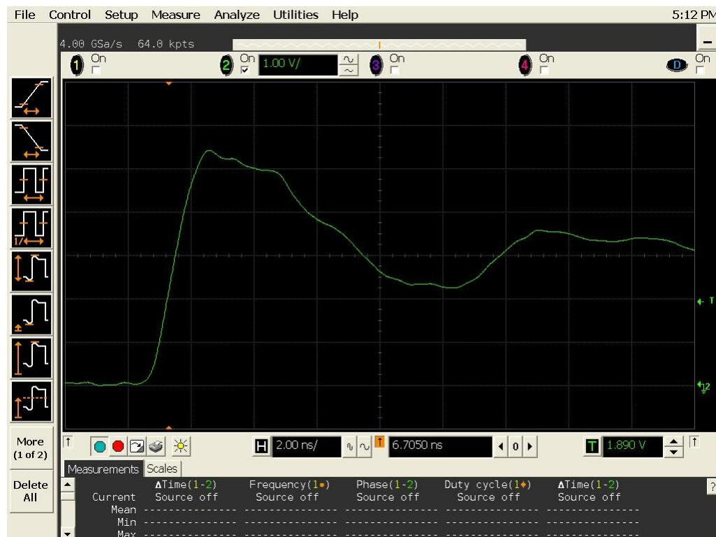
**Figure 11b DUT 694 Post-Annealing Rising edge**
