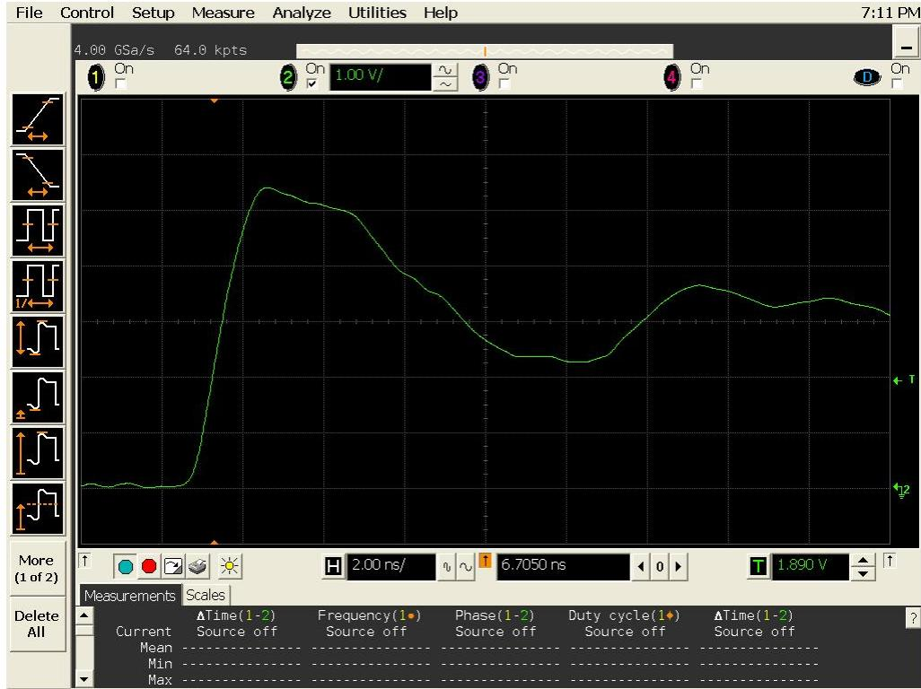
Figure 10a DUT 691 Pre-Irradiation Rising Edge
