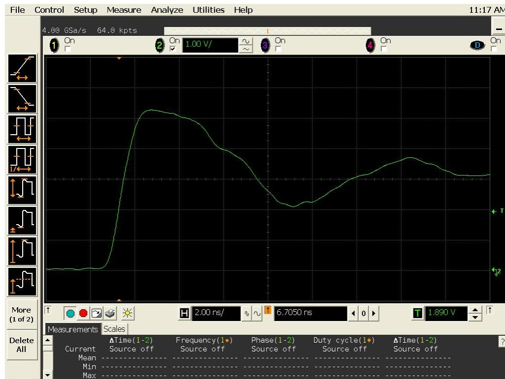
**Figure 11a DUT 694 Pre-Radiation Rising Edge**
