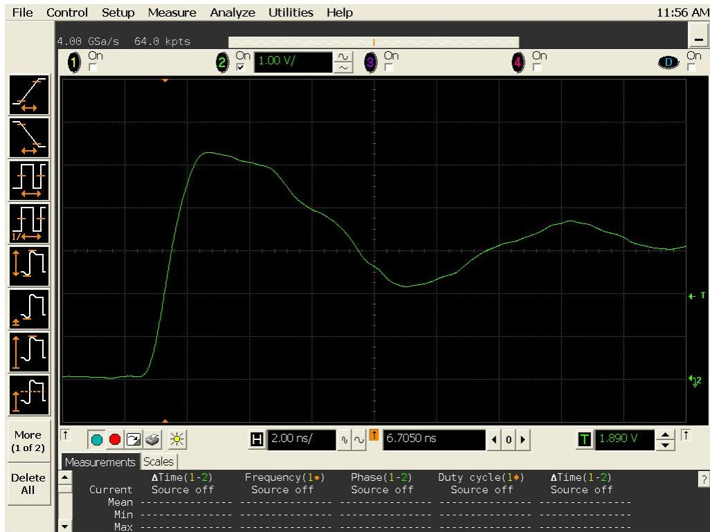
Figure 14a DUT 706 Pre-Irradiation Rising Edge
