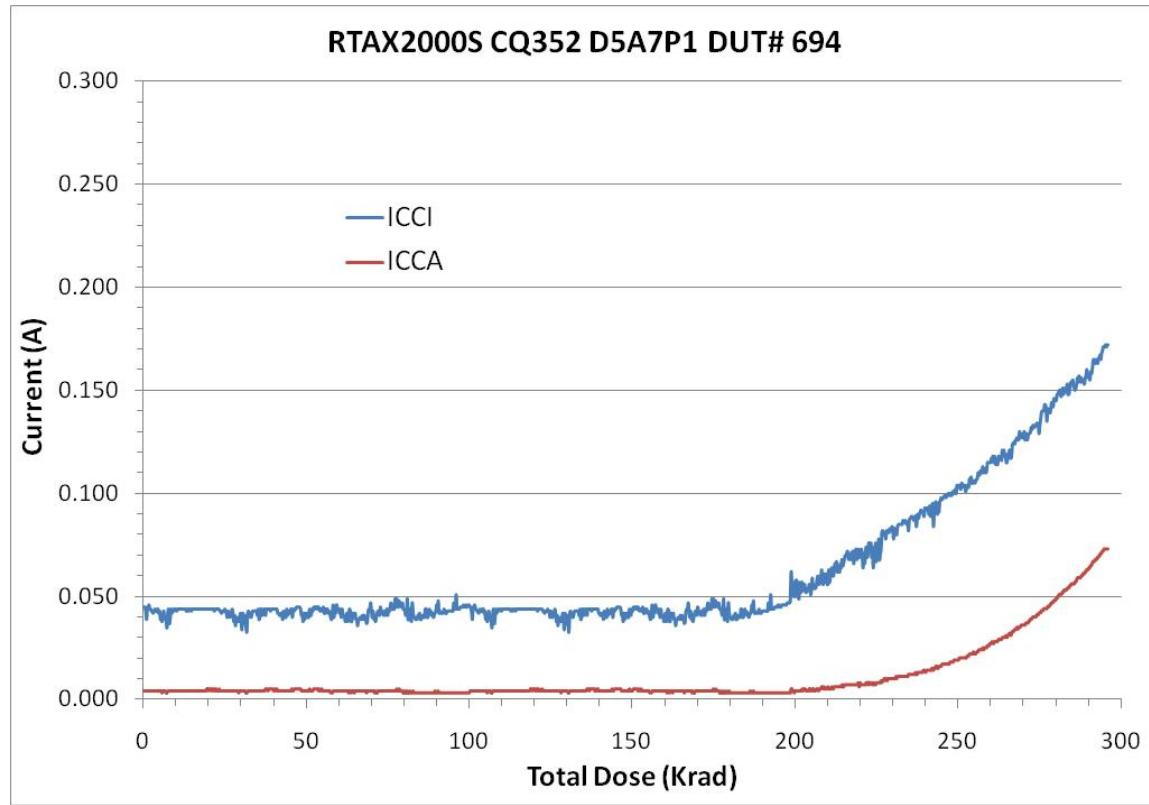
Figure 4 DUT 694 Influx ICCA and ICCI (some measurement noises are present)
