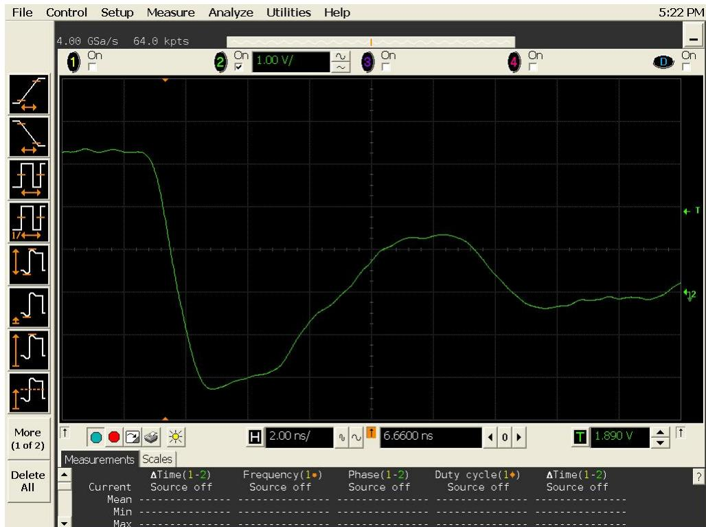
Figure 20b DUT 706 Post-Annealing Falling Edge
