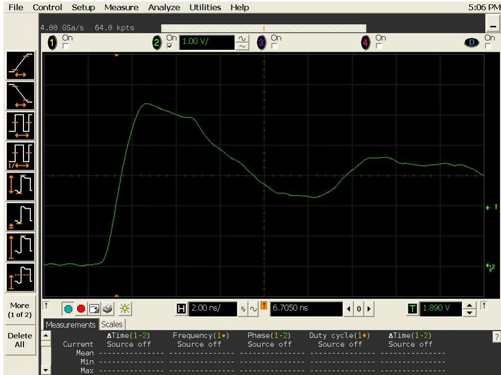
Figure 10b DUT 691 Post-Annealing Rising Edge
