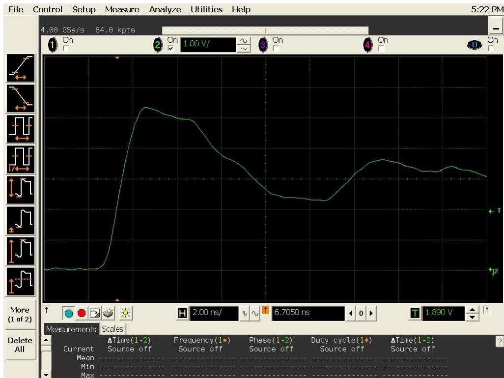
Figure 14b DUT 706 Post-Annealing Rising Edge
