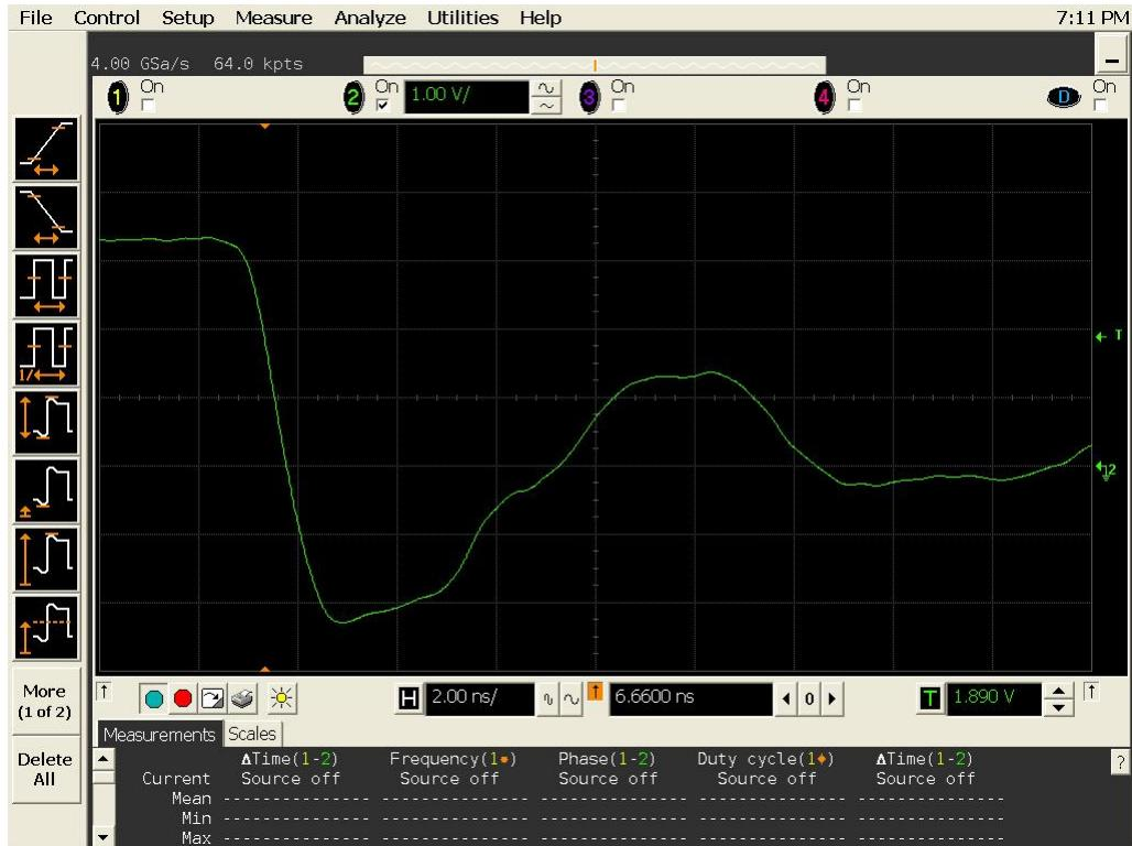
Figure 16a DUT 691 Pre-Irradiation Falling Edge
