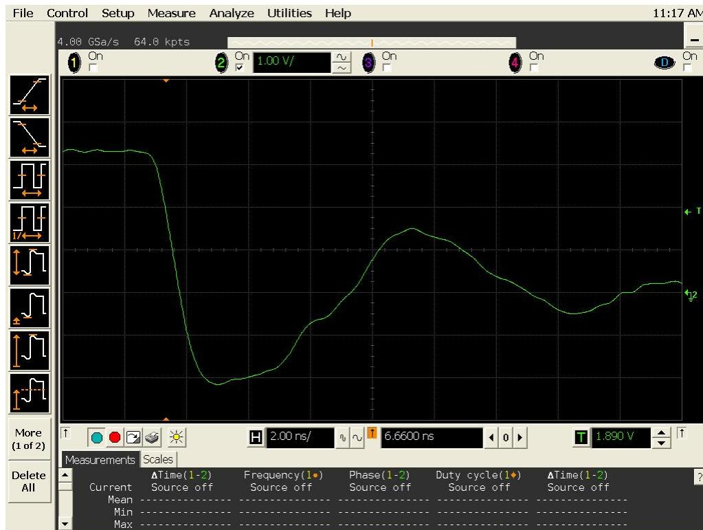
Figure 17a DUT 694 Pre-Irradiation Falling Edge
