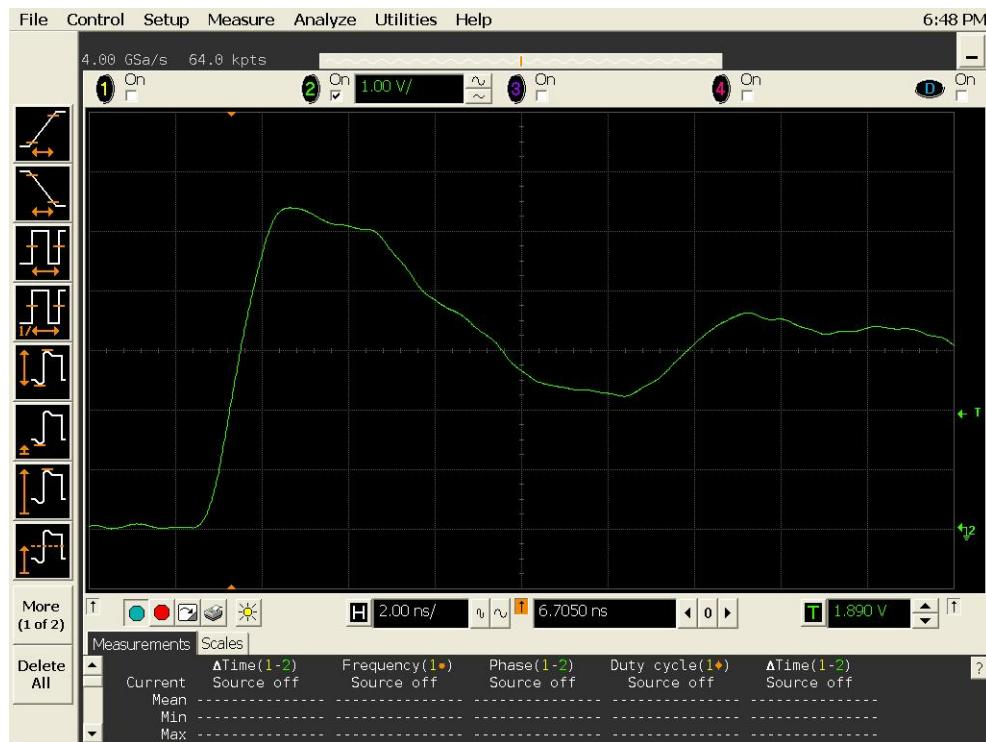
Figure 9a DUT 680 Pre-Irradiation Rising Edge
