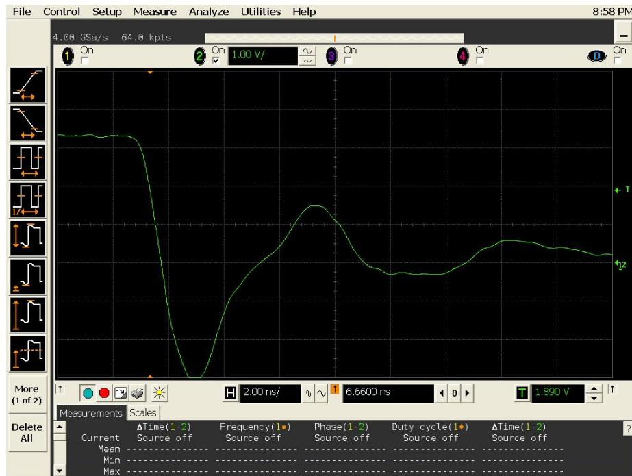
Figure 17a DUT 3023 Pre-Irradiation Falling Edge
