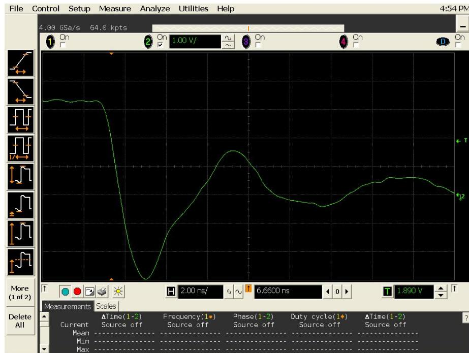
Figure 13a DUT 3000 Pre-Radiation Falling Edge
