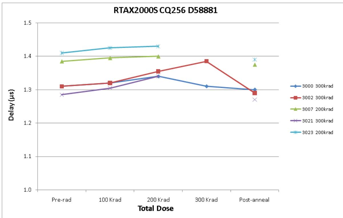
**Figure 7 In-Situ Propagation Delay versus Total Dose**
