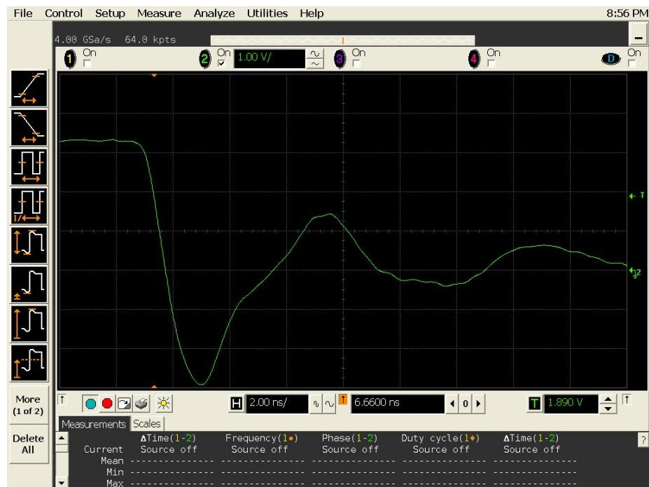
Figure 16a DUT 3021 Pre-Irradiation Falling Edge
