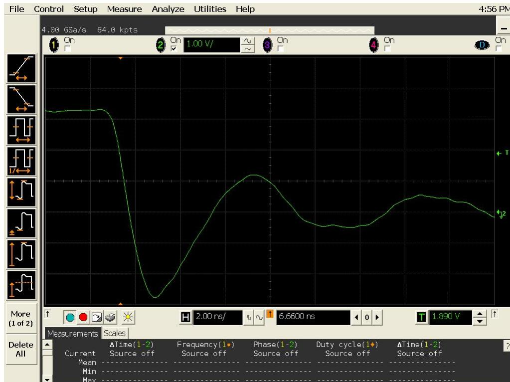
Figure 16b DUT 5319 Post-Annealing Falling Edge
