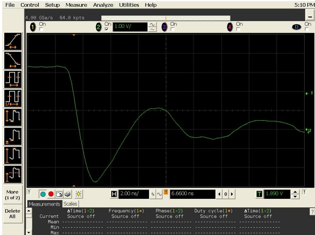
Figure 19b DUT 5355 Post-Annealing Falling Edge
