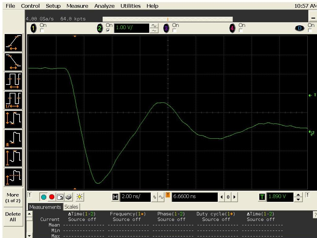
Figure 16a DUT 5319 Pre-Irradiation Falling Edge
