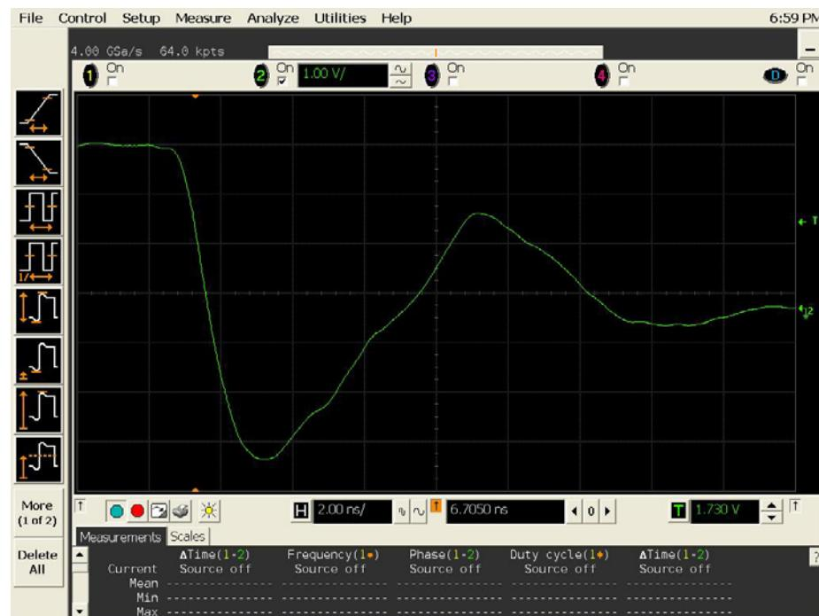
Figure 17b DUT 13932 Post-Annealing Falling Edge
