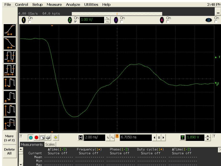
Figure 18a DUT 2532 Pre-Irradiation Falling Edge
