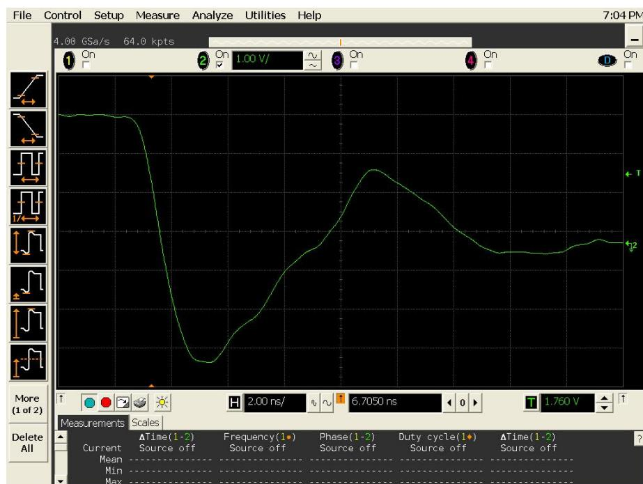
Figure 18b DUT 2532 Post-Annealing Falling Edge
