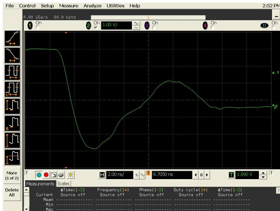
Figure 20a DUT 2550 Pre-Irradiation Falling Edge
