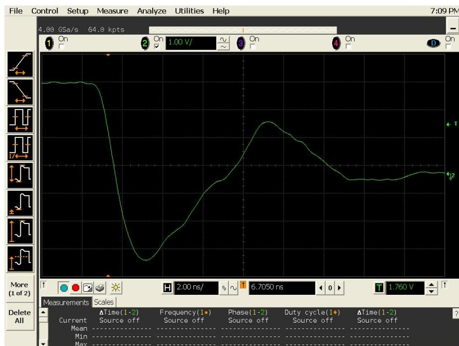
Figure 20b DUT 2550 Post-Annealing Falling Edge
