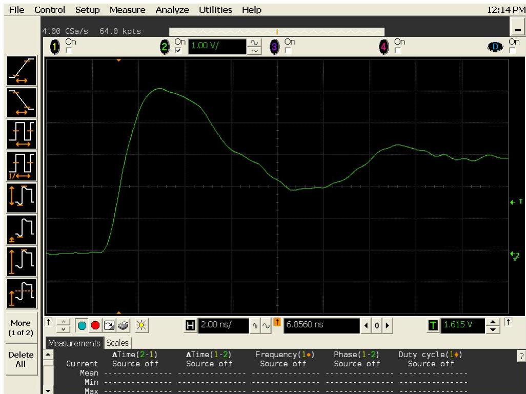
Figure 11b DUT 684 Post-Annealing Rising edge
