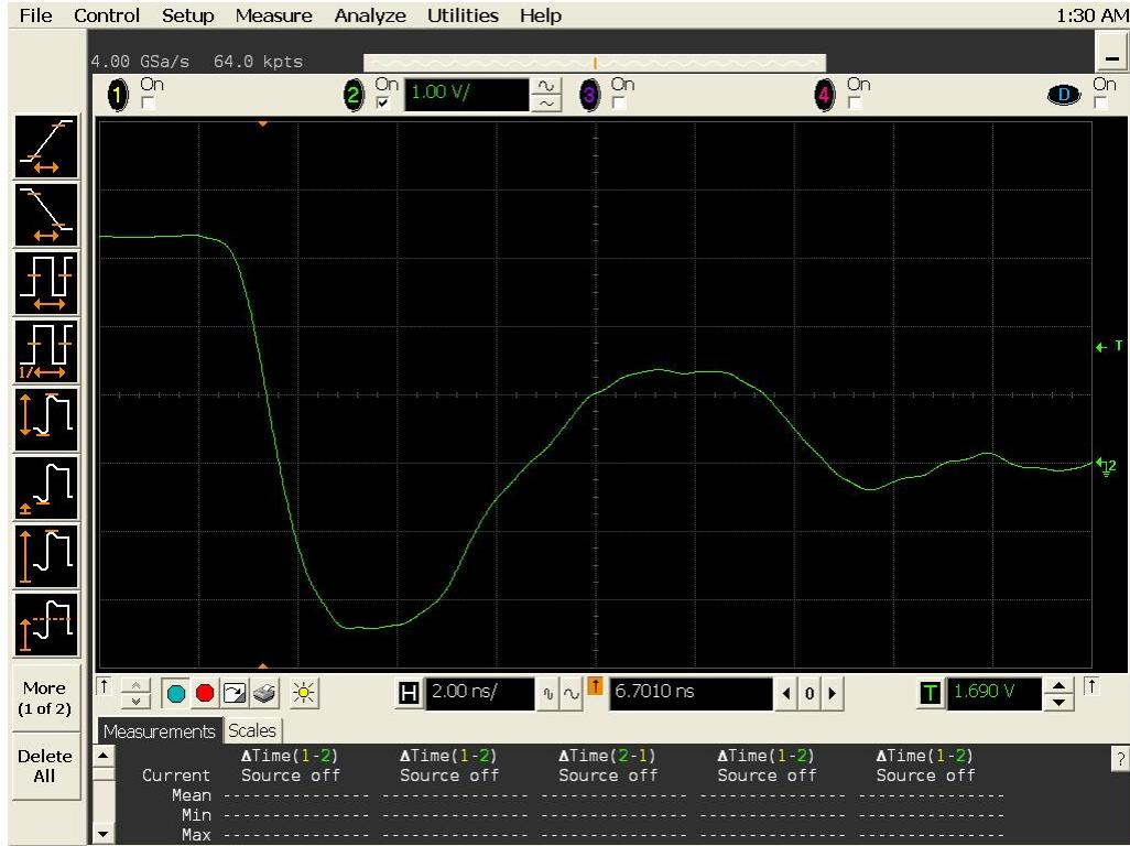
Figure 17a DUT 684 Pre-Irradiation Falling Edge
