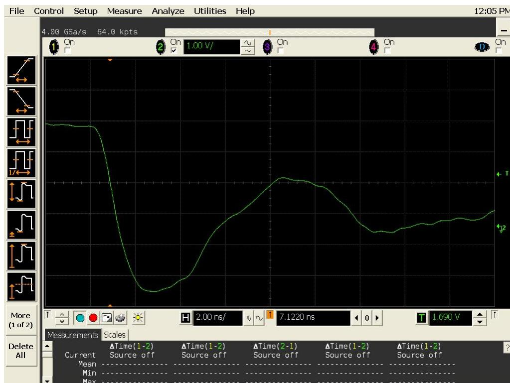
Figure 18b DUT 685 Post-Annealing Falling Edge
