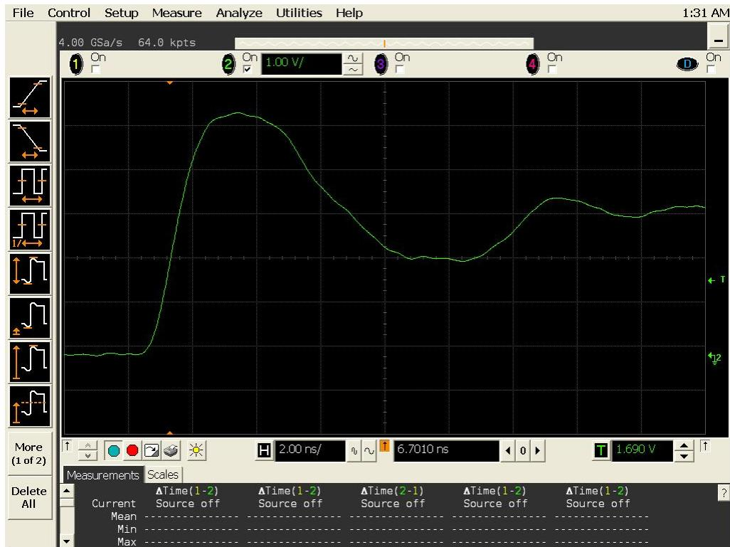
Figure 11a DUT 684 Pre-Radiation Rising Edge
