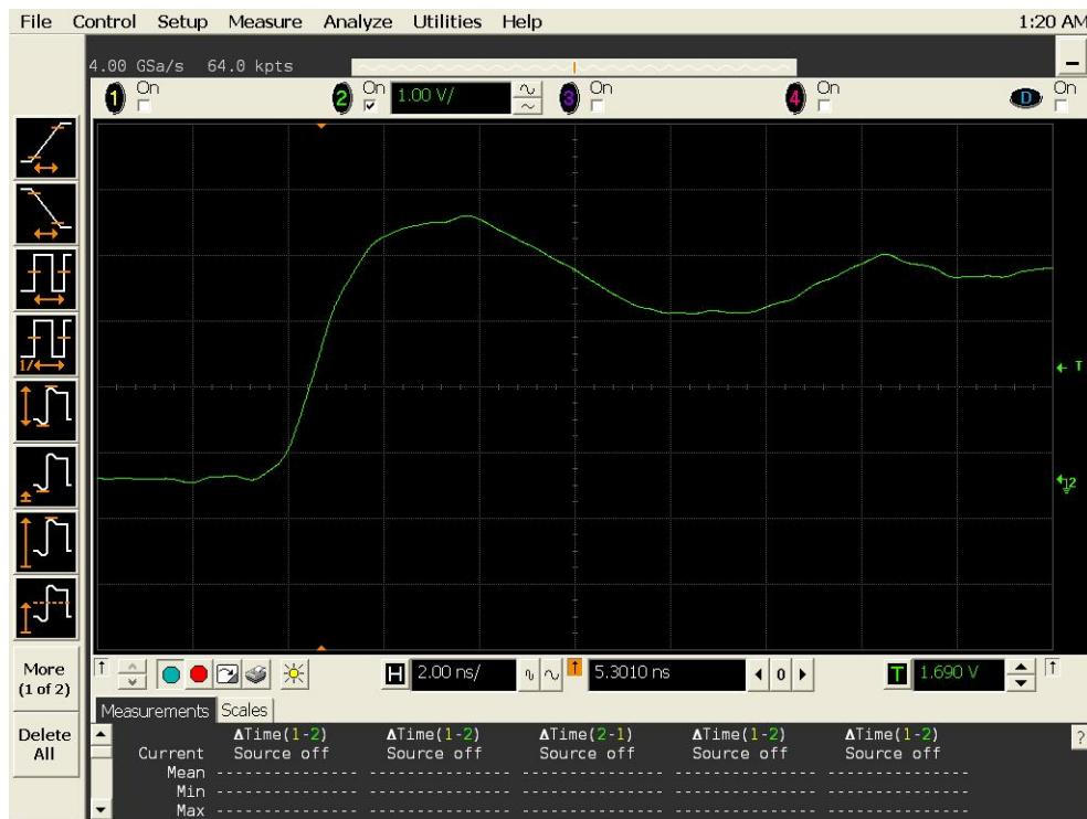
Figure 9a DUT 682 Pre-Irradiation Rising Edge
