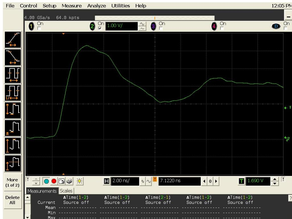
Figure 12b DUT 685 Post-Annealing Rising Edge
