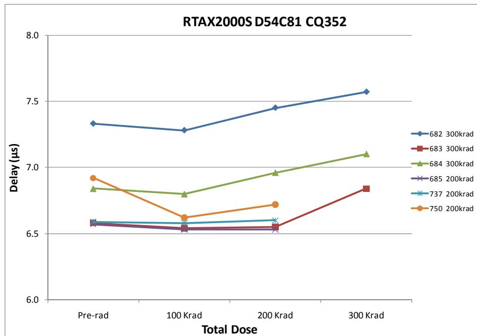
**Figure 8 In-Situ Propagation Delay versus Total Dose**
