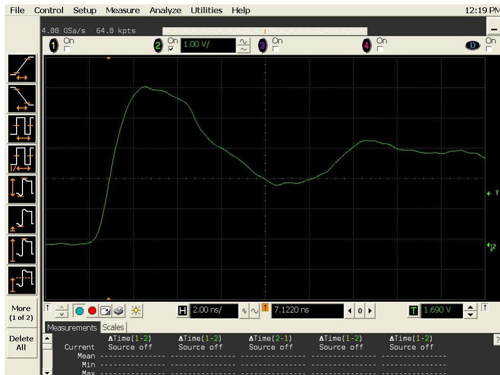
Figure 14b DUT 750 Post-Annealing Rising Edge
