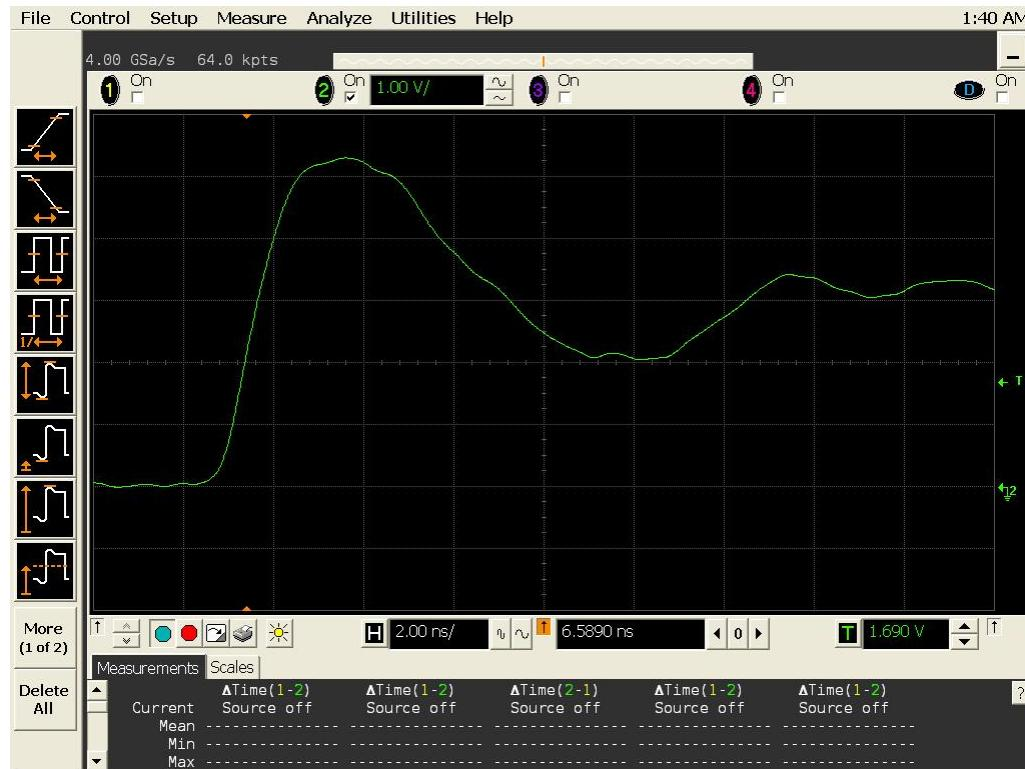
Figure 14a DUT 750 Pre-Irradiation Rising Edge
