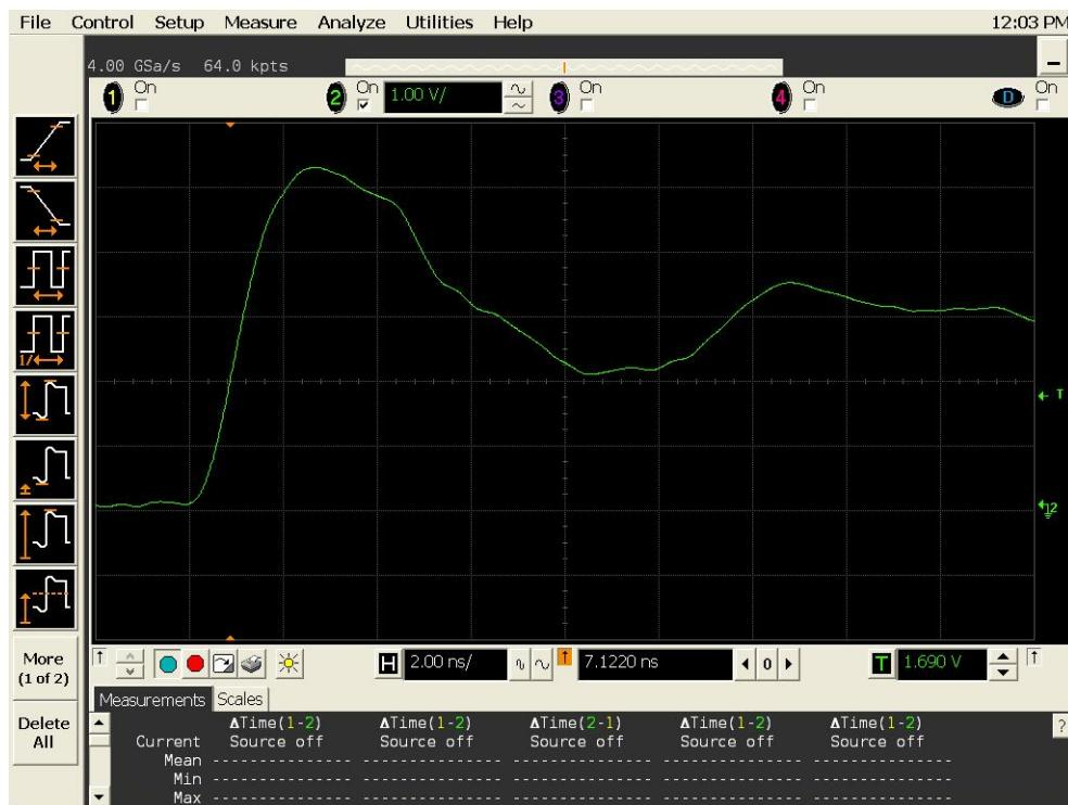
Figure 9b DUT 682 Post-Annealing Rising Edge
