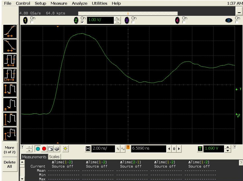
Figure 13a DUT 737 Pre-Irradiation Rising Edge
