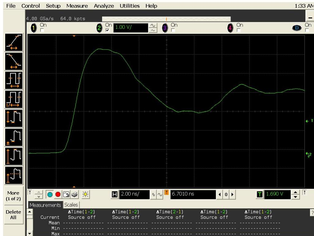
Figure 12a DUT 685 Pre-Irradiation Rising Edge
