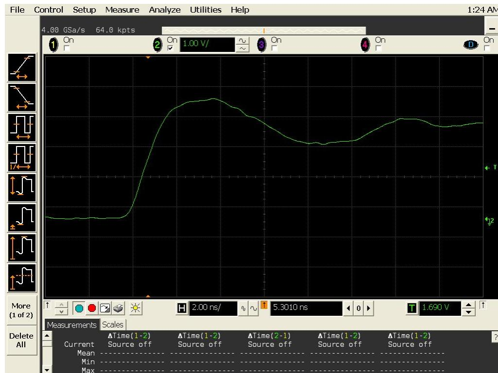
Figure 10a DUT 683 Pre-Irradiation Rising Edge
