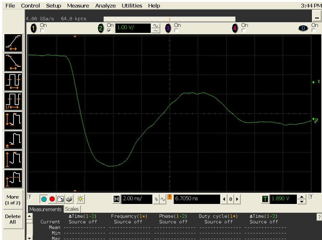
Figure 16b DUT 9659 Post-Annealing Falling Edge
