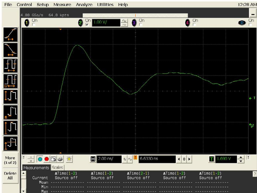
Figure 14a DUT 15746 Pre-Irradiation Rising Edge
