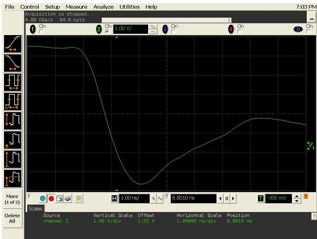
Figure 8(b) DUT 8318 post-annealing falling edge, abscissa scale is 1 ns/div and ordinate scale is 1 V/div.
