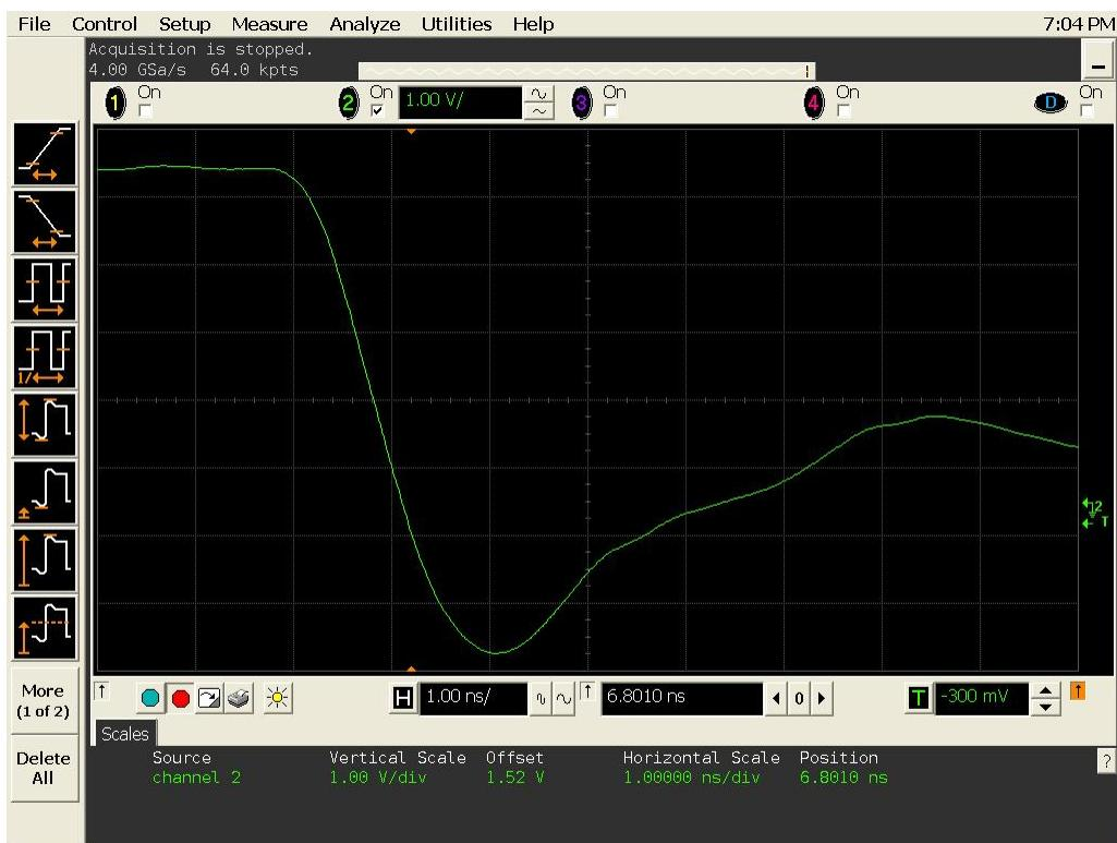
Figure 7(b) DUT 8292 post-annealing falling edge, abscissa scale is 1 ns/div and ordinate scale is 1 V/div.
