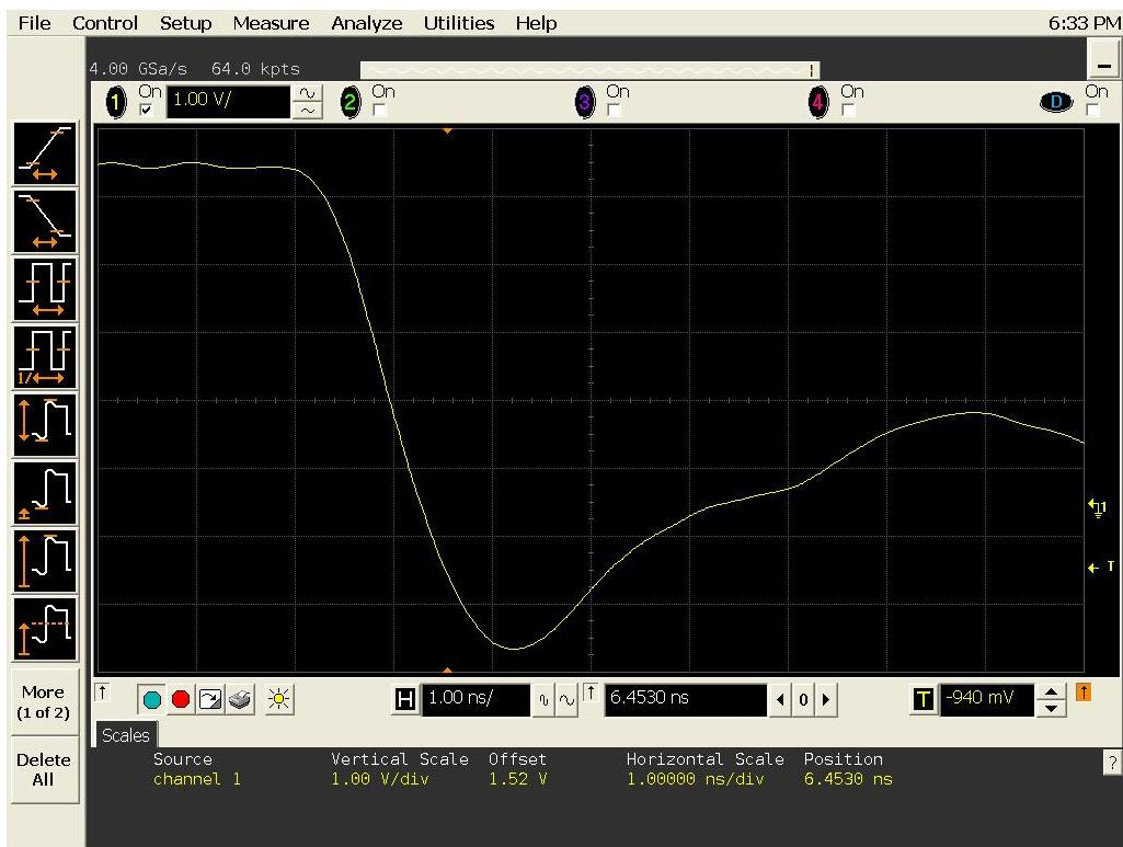
Figure 7(a) DUT 8292 pre-irradiation falling edge, abscissa scale is 1 ns/div and ordinate scale is 1 V/div.
