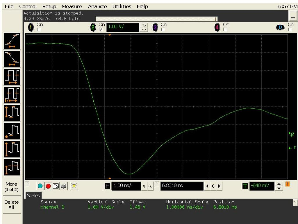
Figure 9(b) DUT 8321 post-annealing falling edge, abscissa scale is 1 ns/div and ordinate scale is 1 V/div.
