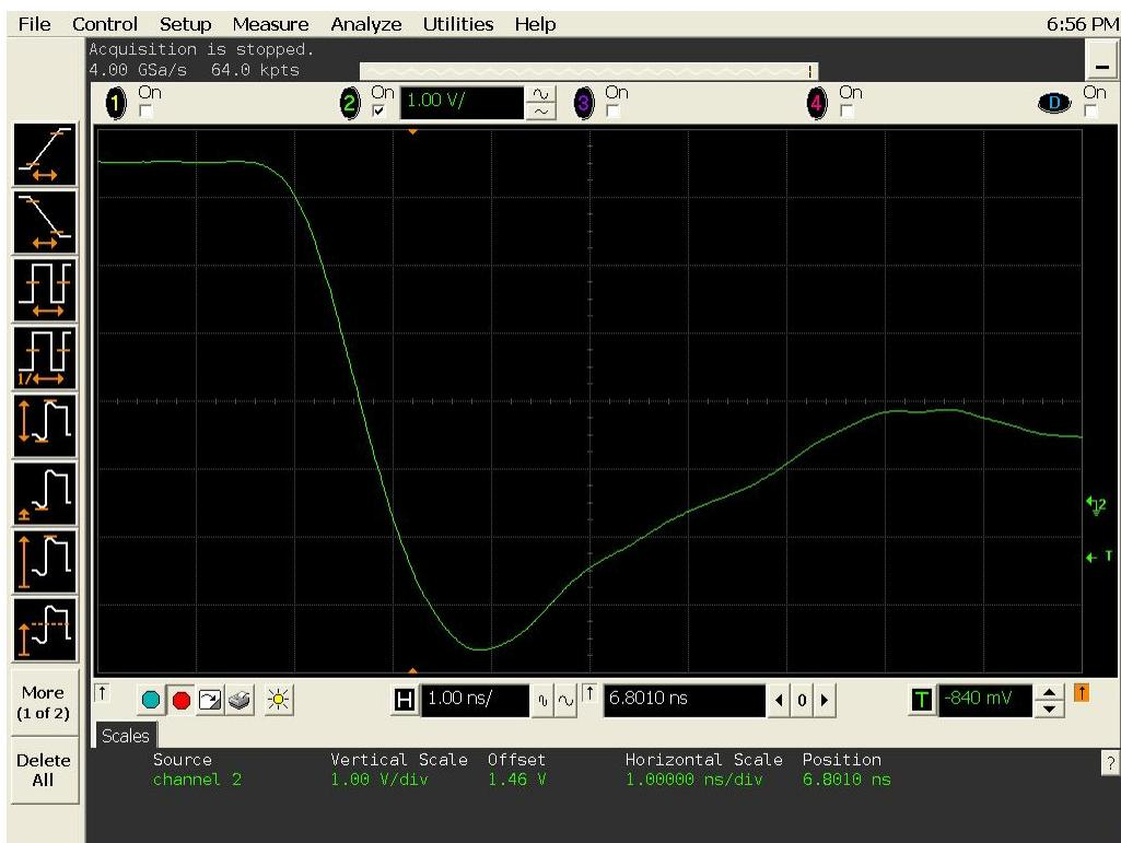
Figure 10(b) DUT 8352 post-irradiation falling edge, abscissa scale is 1 V/div and ordinate scale is 1 ns/div.
