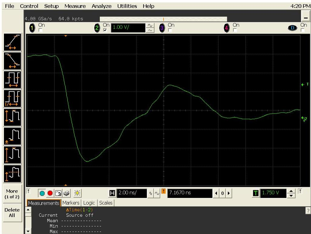
Figure 14(a) DUT 5743 pre-radiation falling edge.
