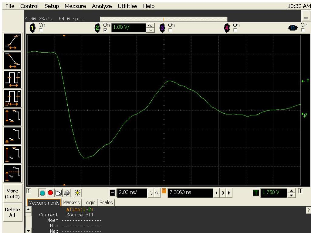
Figure 18(a) DUT 5870 pre-irradiation falling edge.
