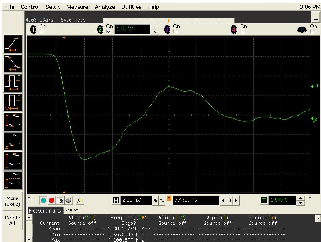
Figure 14(b) DUT 5743 post-annealing falling edge.
