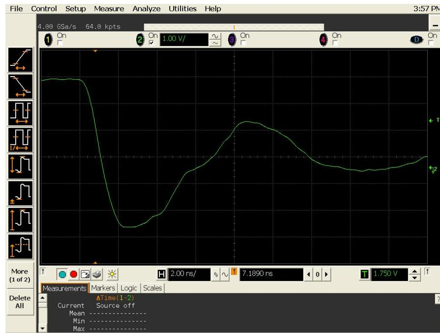
Figure 16(b) DUT 2457 post-annealing falling edge.
