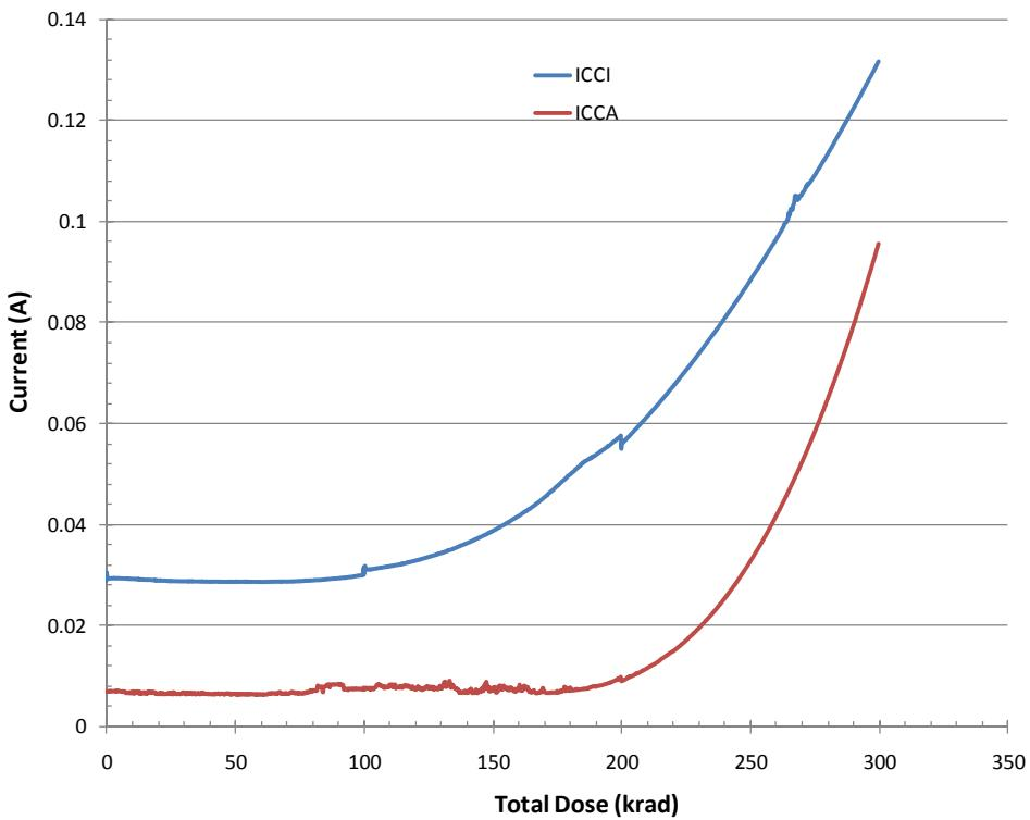
Figure 4 DUT 2460 in-flux  $I_{CCA}$  and  $I_{CCI}$ . If there is any curve-kink occurring at 100 krad or 200 krad, it is due to stopping irradiation for propagation-delay measurement.
