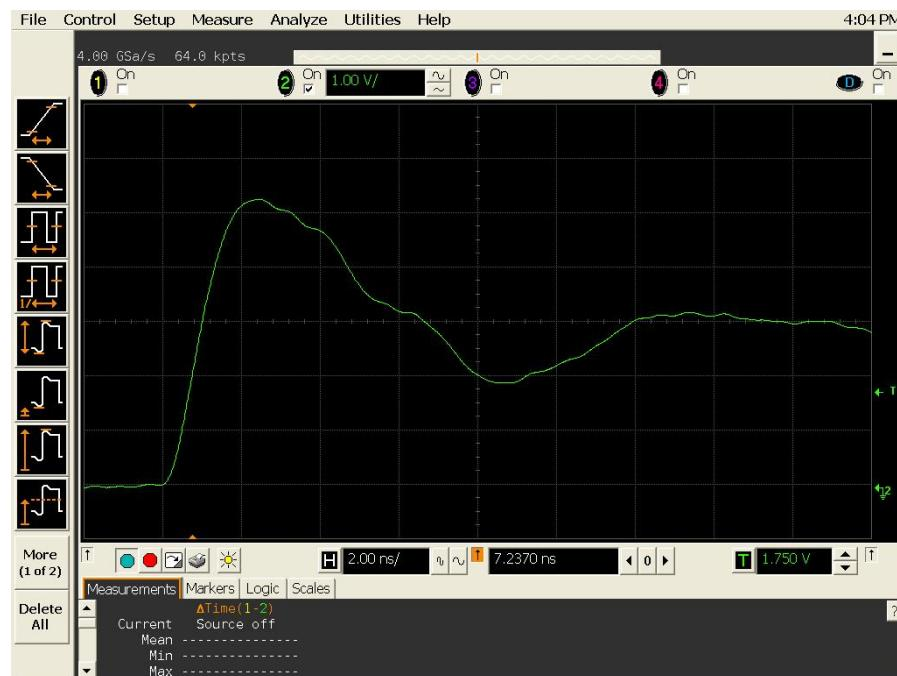
Figure 12(b) DUT 2516 post-annealing rising edge.
