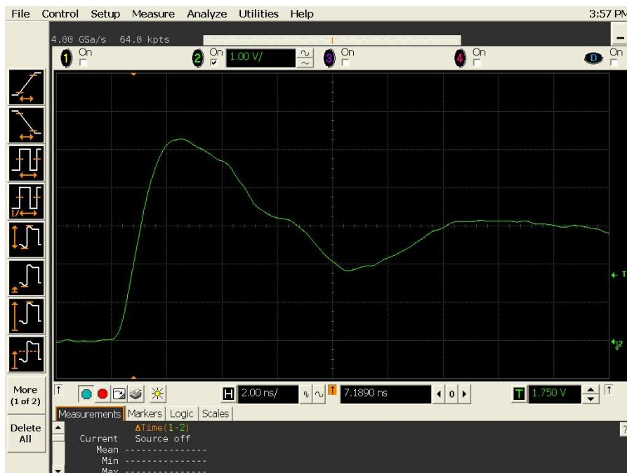
Figure 10(b) DUT 2457 post-annealing rising edge.
