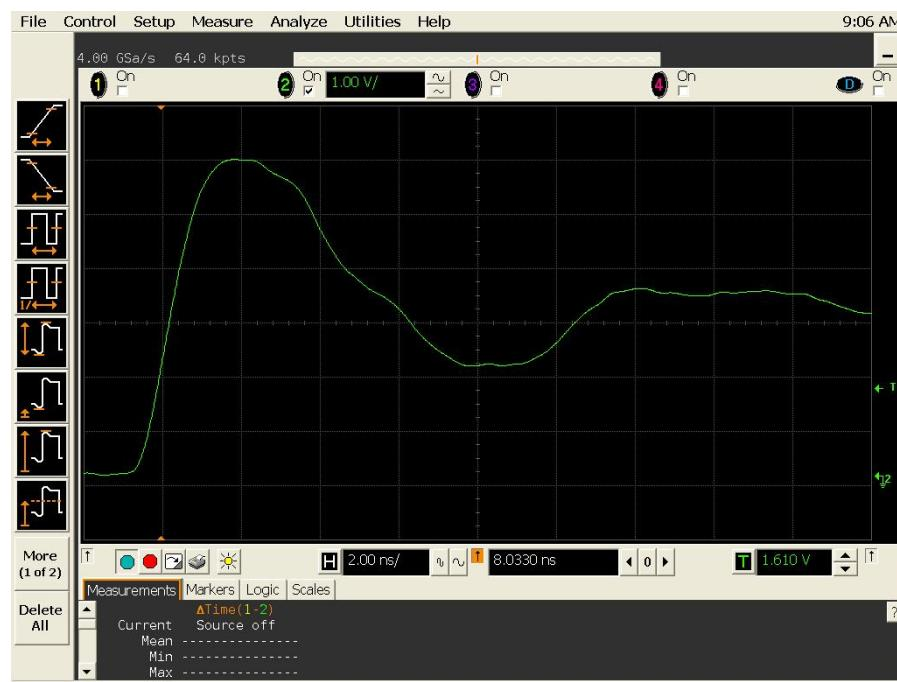
Figure 13(a) DUT 2517 pre-irradiation rising edge.
