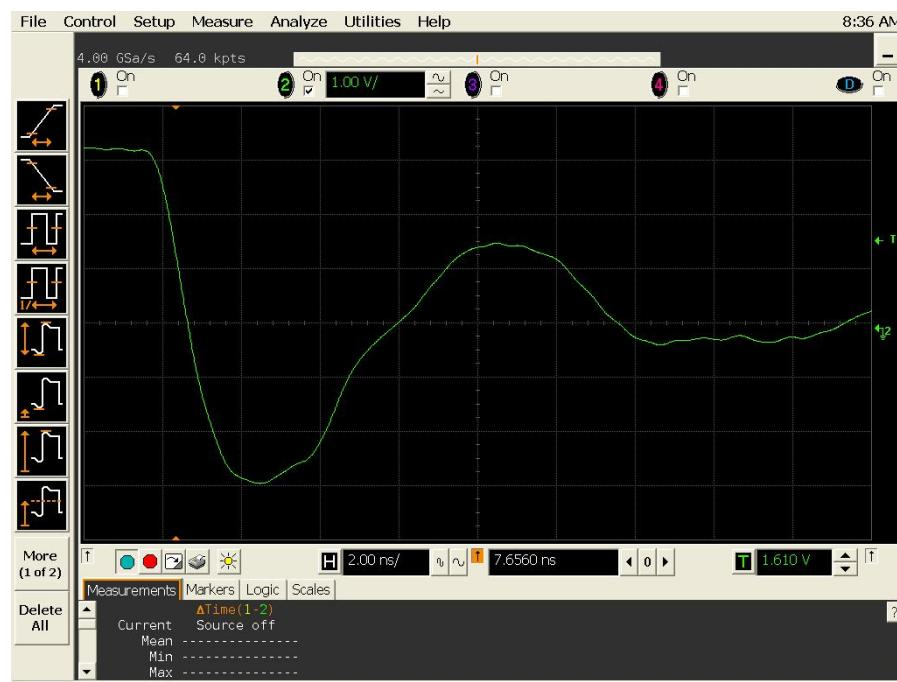
Figure 16(a) DUT 2457 pre-irradiation falling edge.
