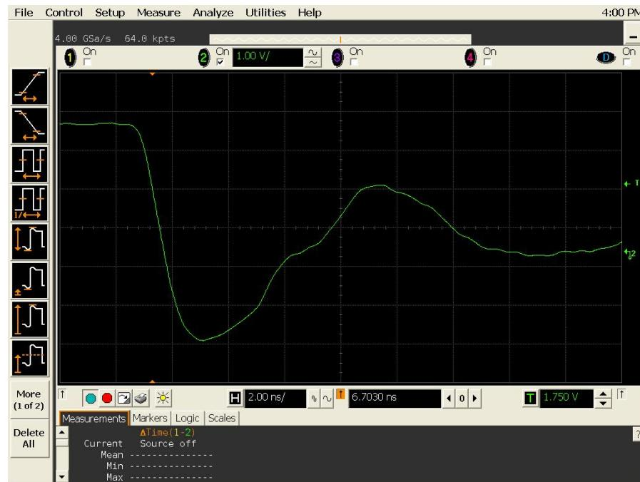
Figure 17(b) DUT 2460 post-annealing falling edge.
