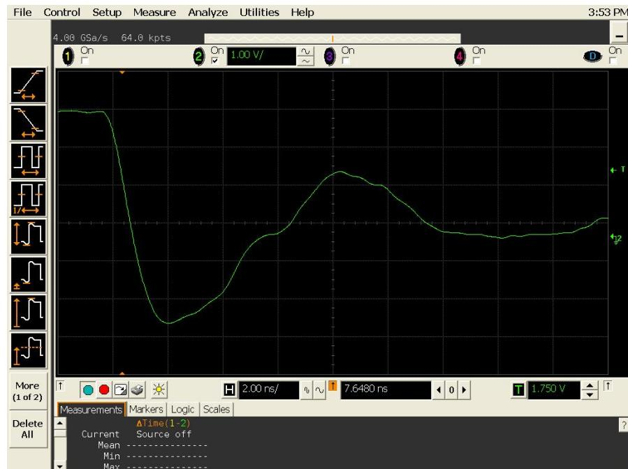
Figure 21(b) DUT 2519 post-annealing falling edge.
