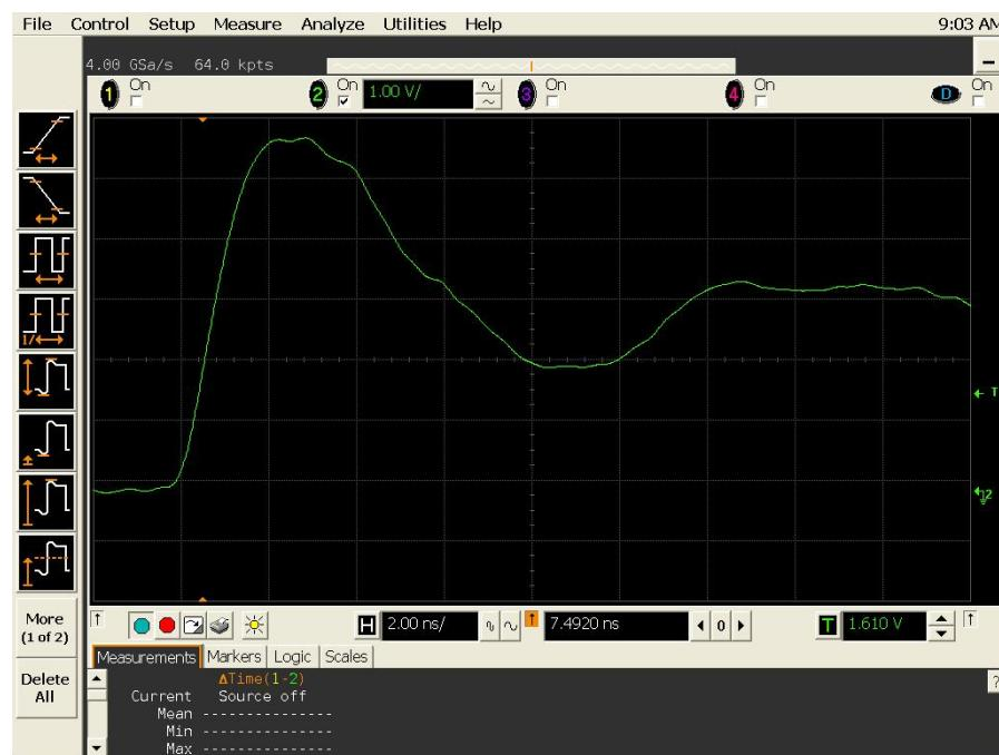
Figure 12(a) DUT 2516 pre-radiation rising edge.
