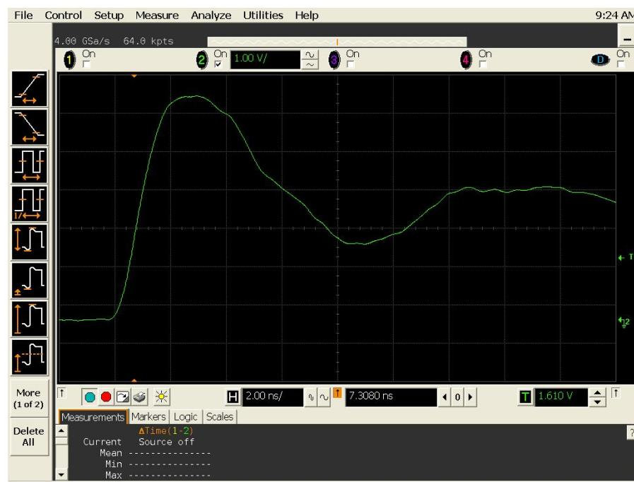
Figure 14(a) DUT 2518 pre-irradiation rising edge.
