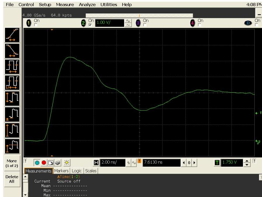
Figure 13(b) DUT 2517 post-annealing rising edge.
