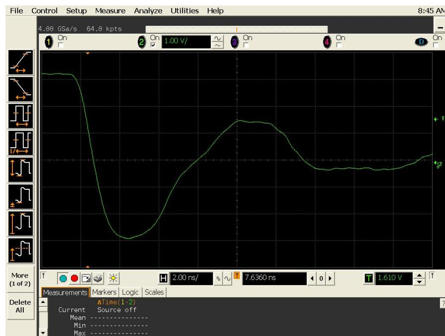
Figure 17(a) DUT 2460 pre-irradiation falling edge.
