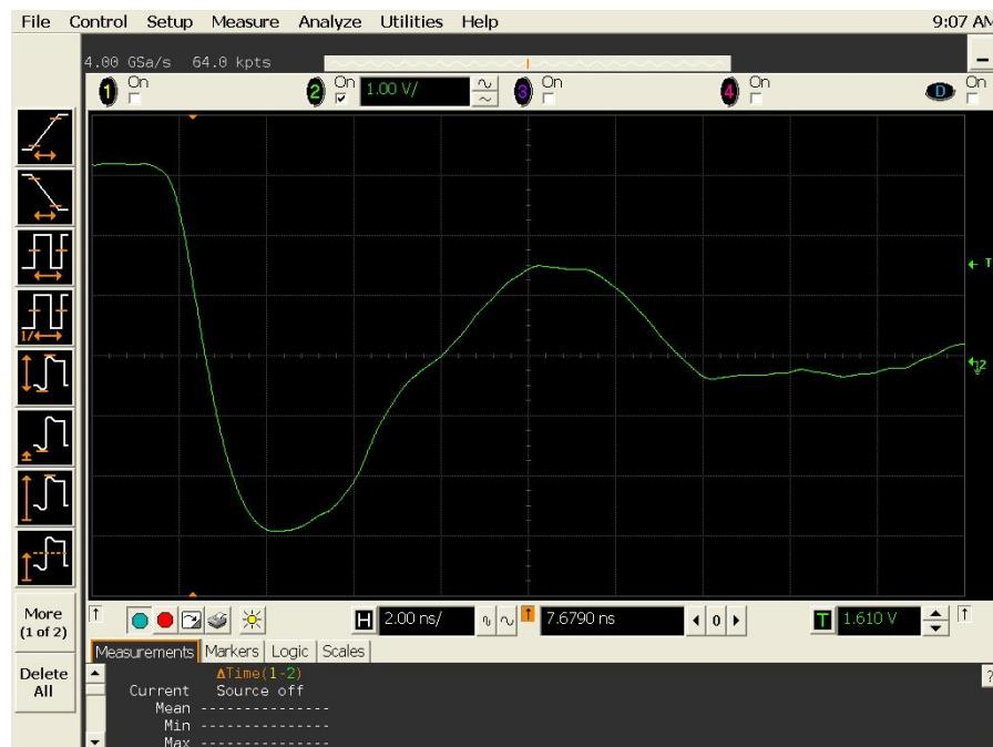
Figure 19(a) DUT 2517 pre-irradiation falling edge.
