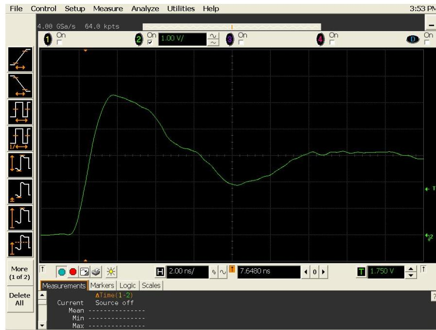
Figure 15(b) DUT 2519 post-annealing rising edge.
