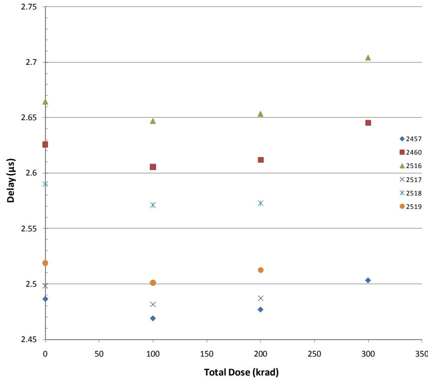
Figure 9 In-situ propagation delay versus total dose. The measurement was performed when irradiation was temporarily stopped.
