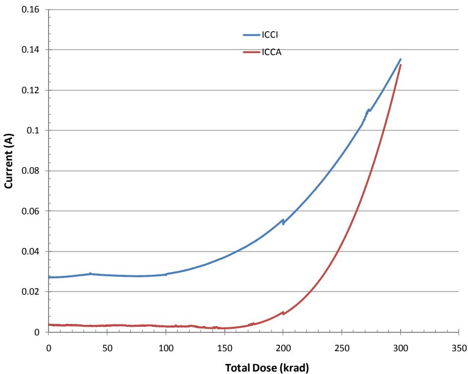
Figure 5 DUT 2516 in-flux  $I_{CCA}$  and  $I_{CCI}$ . If there is any curve-kink occurring at 100 krad or 200 krad, it is due to stopping irradiation for propagation-delay measurement.
