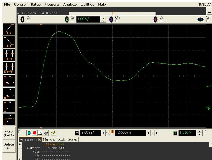
Figure 10(a) DUT 2457 pre-irradiation rising edge.
