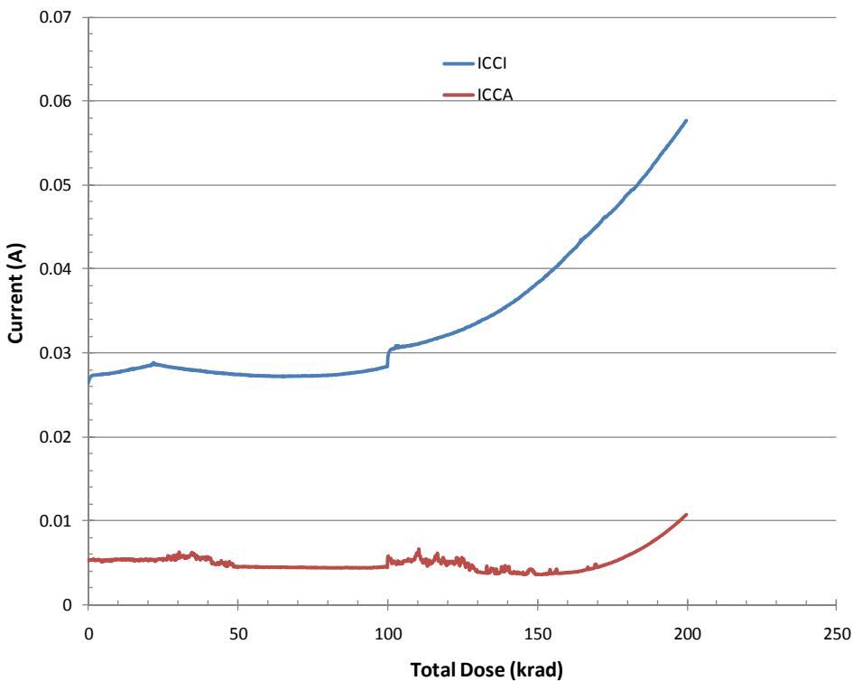
Figure 6 DUT 2517 in-flux  $I_{CCA}$  and  $I_{CCI}$ . If there is any curve-kink occurring at 100 krad, it is due to stopping irradiation for propagation-delay measurement.
