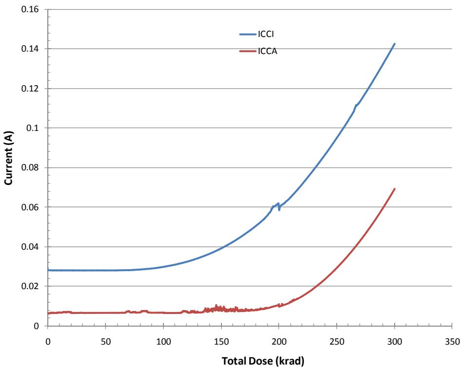
Figure 3 DUT 2457 in-flux  $I_{CCA}$  and  $I_{CCI}$ . If there is any curve-kink occurring at 100 krad or 200 krad, it is due to stopping irradiation for propagation-delay measurement.
