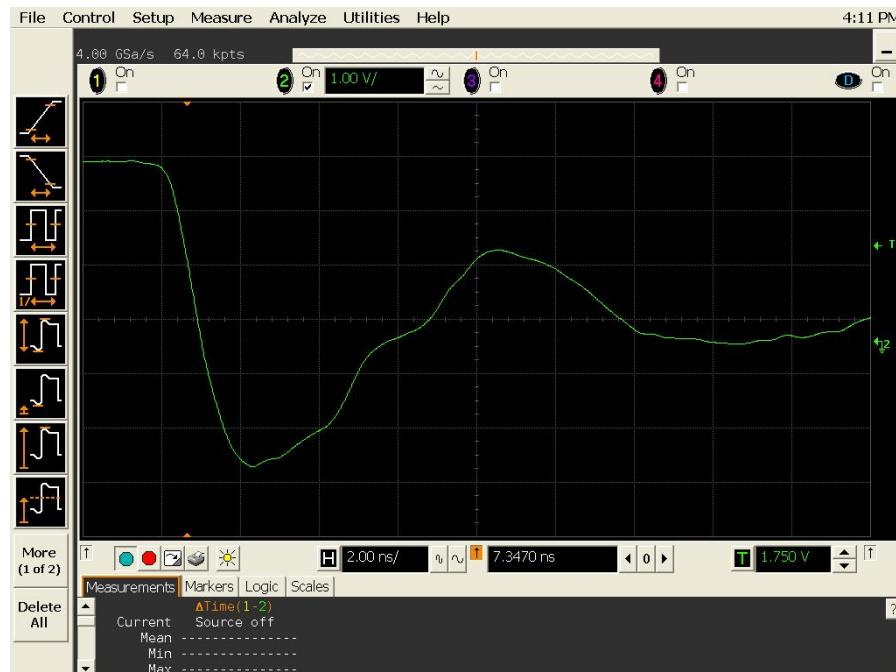
Figure 20(b) DUT 2518 post-annealing falling edge.
