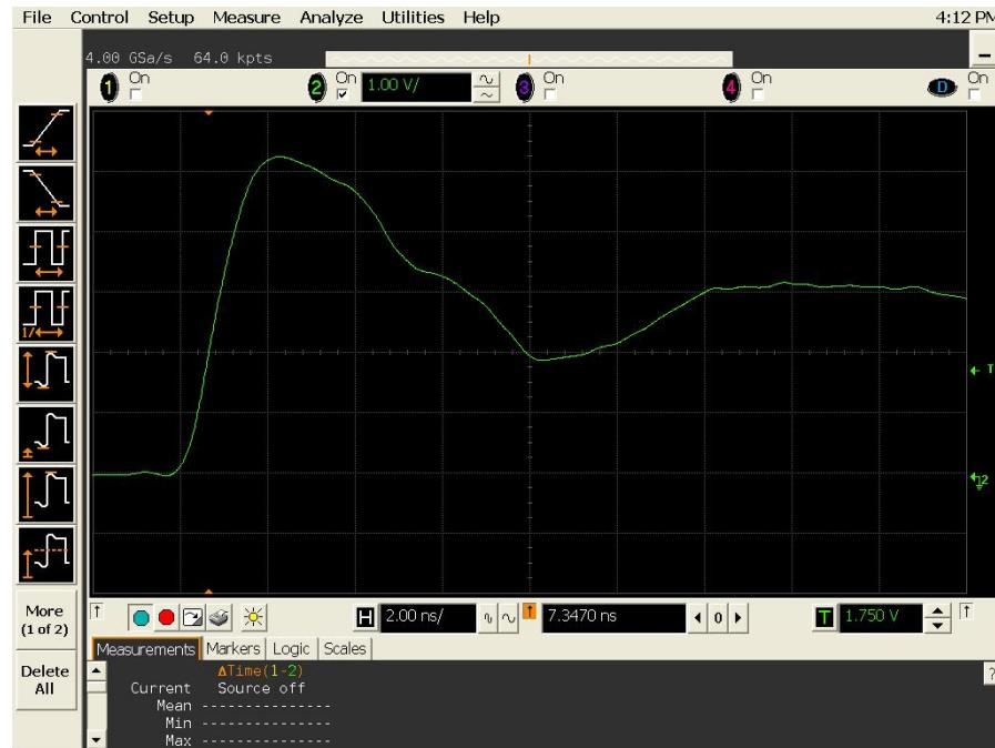
Figure 14(b) DUT 2518 post-annealing rising edge.
