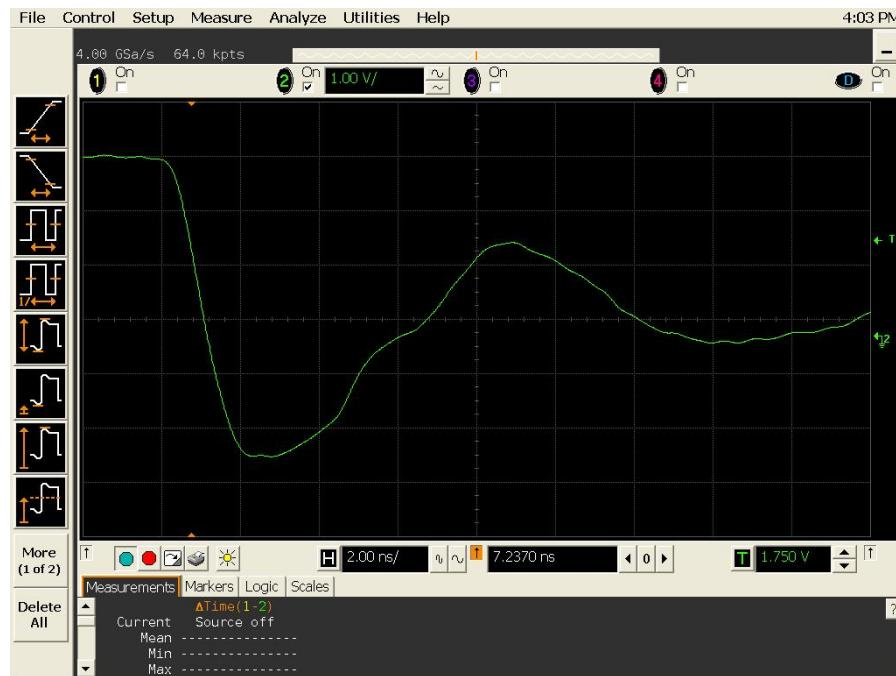
Figure 18(b) DUT 2516 post-annealing falling edge.
