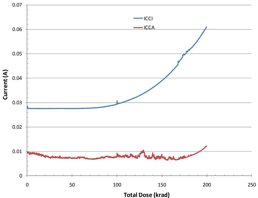
Figure 8 DUT 2519 in-flux  $I_{CCA}$  and  $I_{CCI}$ . If there is any curve-kink occurring at 100 krad, it is due to stopping irradiation for propagation-delay measurement.
