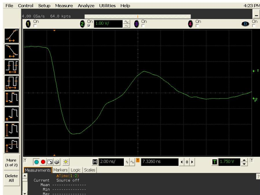
Figure 21(a) DUT 2519 pre-irradiation falling edge.
