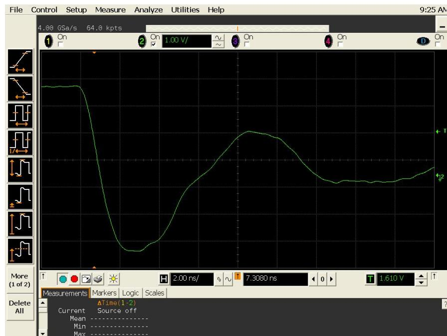
Figure 20(a) DUT 2518 pre-irradiation falling edge.
