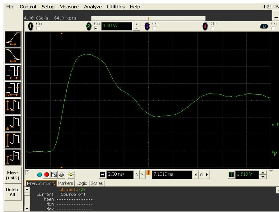
Figure 15(a) DUT 2519 pre-irradiation rising edge.
