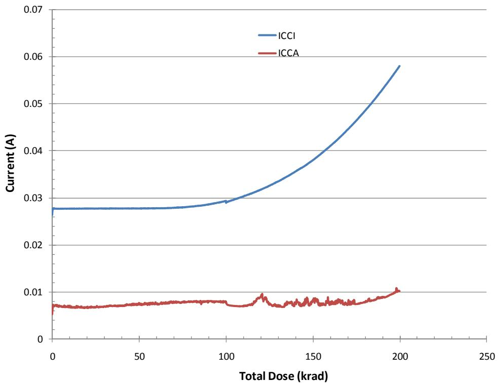
Figure 7 DUT 2518 in-flux  $I_{CCA}$  and  $I_{CCI}$ . If there is any curve-kink occurring at 100 krad, it is due to stopping irradiation for propagation-delay measurement.
