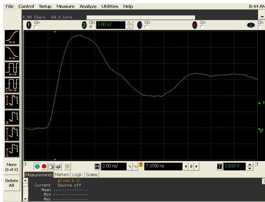
Figure 11(a) DUT 2460 pre-irradiation rising edge.
