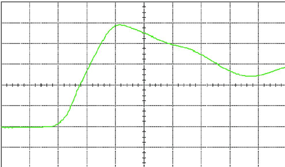
Figure 10(b) DUT 3931 post-annealing rising edge, abscissa scale is 1 V/div and ordinate scale is 1 ns/div.
