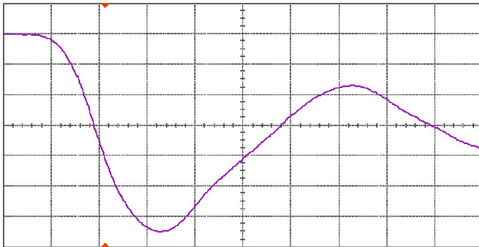
Figure 12(a) DUT 3859 pre-irradiation falling edge, abscissa scale is 1 V/div and ordinate scale is 1 ns/div.
