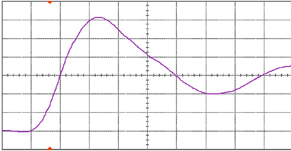
Figure 8(a) DUT 3859 pre-irradiation rising edge, abscissa scale is 1 V/div and ordinate scale is 1 ns/div .
