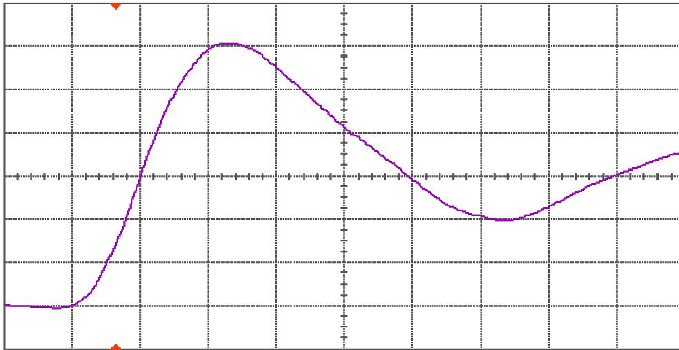
Figure 7(a) DUT 3853 pre-irradiation rising edge, abscissa scale is 1 V/div and ordinate scale is 1 ns/div .
