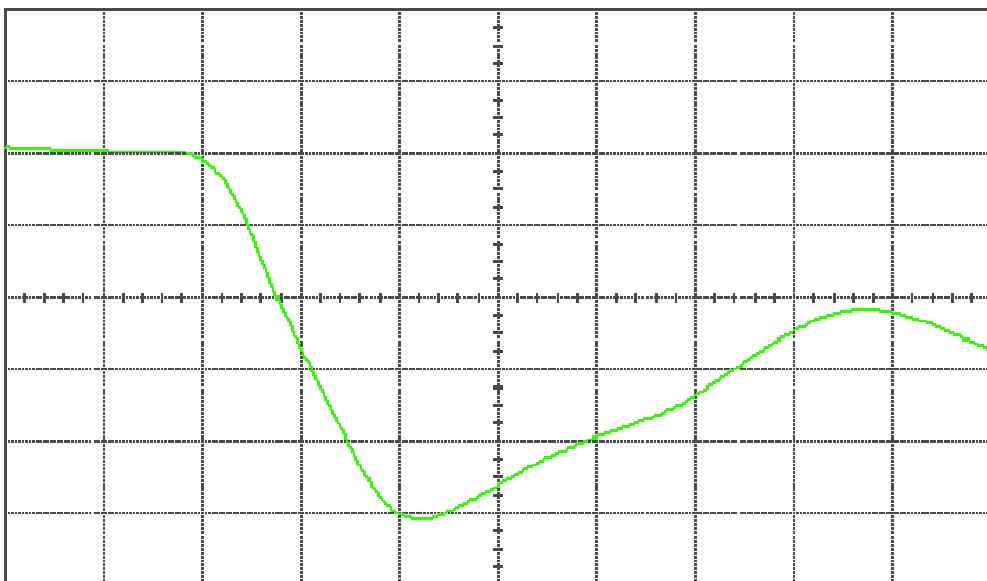
Figure 11(b) DUT 3853 post-annealing falling edge, abscissa scale is 1 V/div and ordinate scale is 1 ns/div.
