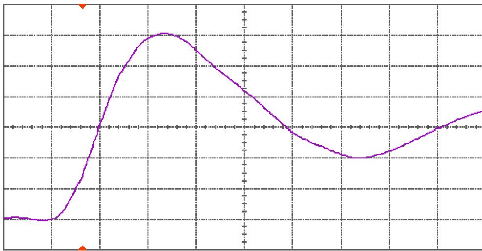
Figure 9(a) DUT 3916 pre-irradiation rising edge, abscissa scale is 1 V/div and ordinate scale is 1 ns/div .
