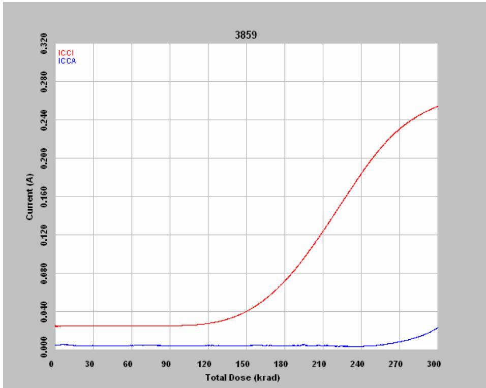
Figure 4 DUT 3859 in-flux  $I_{CCA}$  and  $I_{CCl}$
