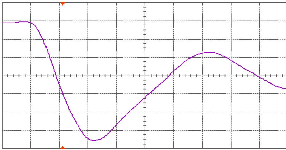
Figure 11(a) DUT 3853 pre-irradiation falling edge, abscissa scale is 1 V/div and ordinate scale is 1 ns/div.
