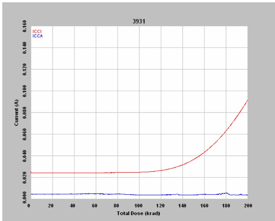
Figure 6 DUT 3931 in-flux  $I_{CCA}$  and  $I_{CCI}$
