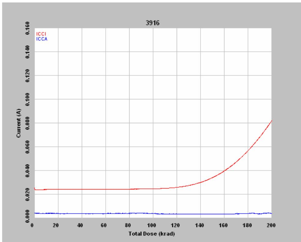
Figure 5 DUT 3916 in-flux  $I_{CCA}$  and  $I_{CCI}$
