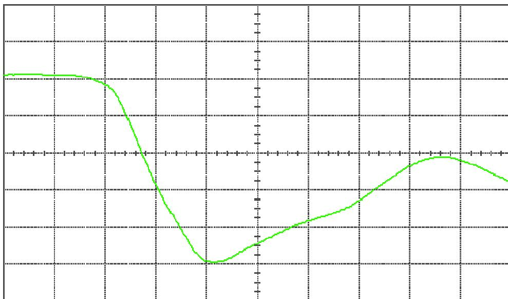
Figure 14(b) DUT 3931 post-annealing falling edge, abscissa scale is 1 V/div and ordinate scale is 1 ns/div.
