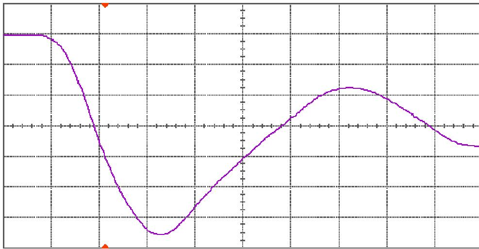
Figure 13(a) DUT 3916 pre-irradiation falling edge, abscissa scale is 1 V/div and ordinate scale is 1 ns/div.
