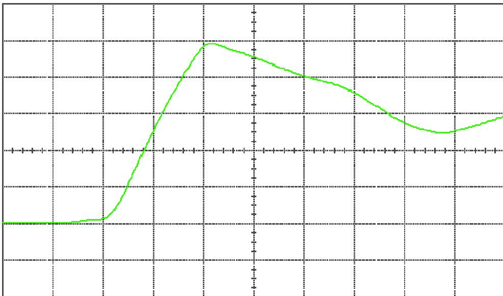
Figure 9(b) DUT 3916 post-annealing rising edge, abscissa scale is 1 V/div and ordinate scale is 1 ns/div
