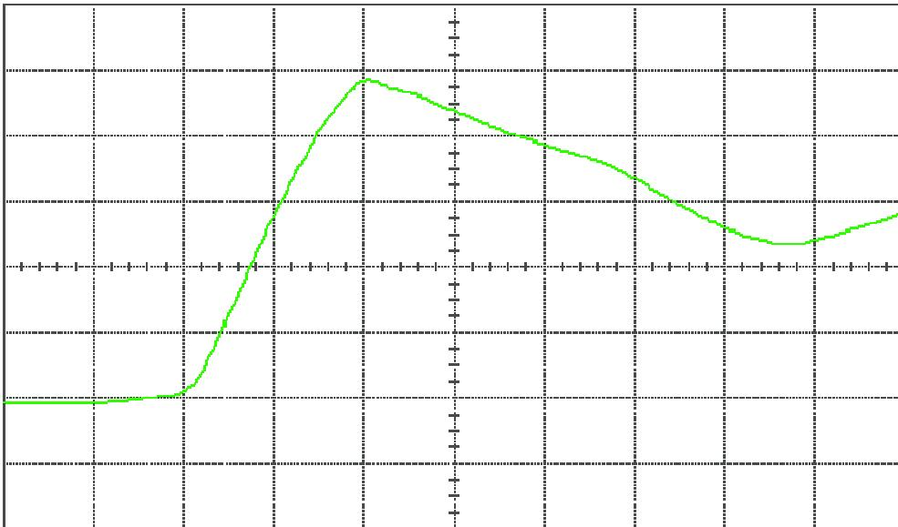
Figure 7(b) DUT 3853 post-annealing rising edge, abscissa scale is 1 V/div and ordinate scale is 1 ns/div.
