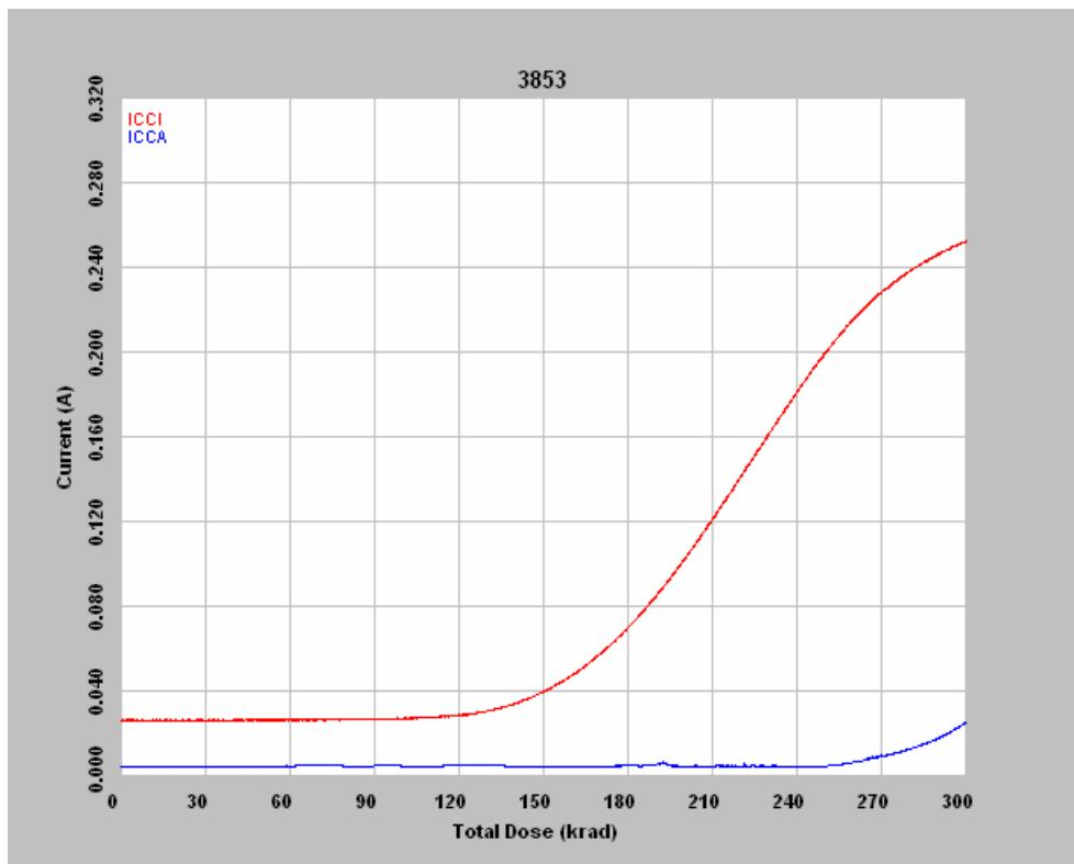
Figure 3 DUT 3853 in-flux  $I_{CCA}$  and  $I_{CCl}$ . The spikes are due to bad contacts.
