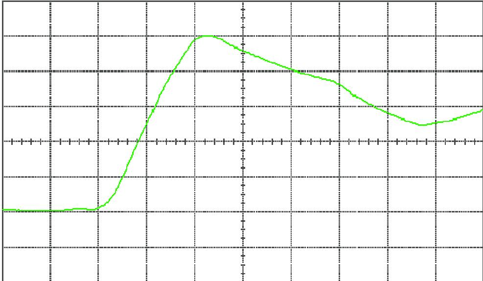
Figure 8(b) DUT 3859 post-annealing rising edge, abscissa scale is 1 V/div and ordinate scale is 1 ns/div.
