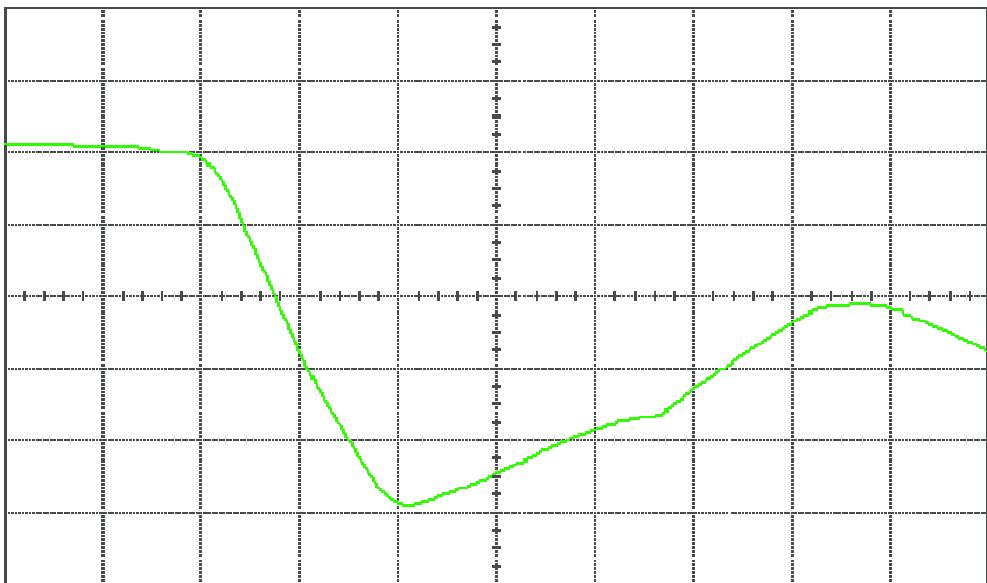
Figure 13(b) DUT 3916 post-annealing falling edge, abscissa scale is 1 V/div and ordinate scale is 1 ns/div.
