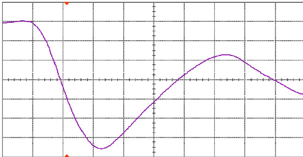
Figure 14(a) DUT 3931 pre-irradiation falling edge, abscissa scale is 1 V/div and ordinate scale is 1 ns/div.
