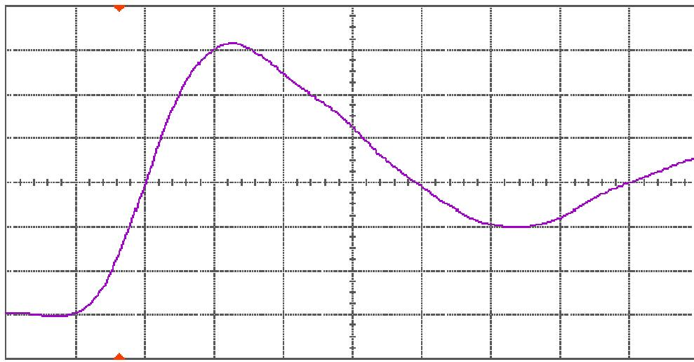
Figure 10(a) DUT 3931 pre-irradiation rising edge, abscissa scale is 1 V/div and ordinate scale is 1 ns/div .
