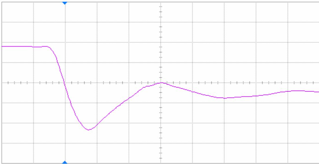
Figure 15(a) DUT 84539 pre-irradiation falling edge, abscissa scale is 2 V/div and ordinate scale is 2 ns/div.
