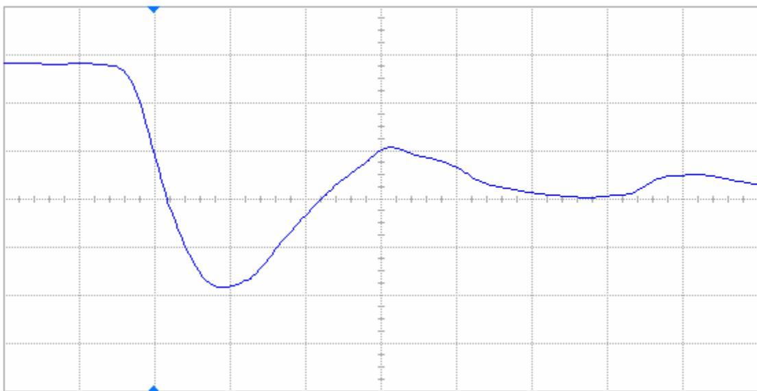
Figure 16(b) DUT 84543 post-annealing falling edge, abscissa scale is 2 V/div and ordinate scale is 2 ns/div.
