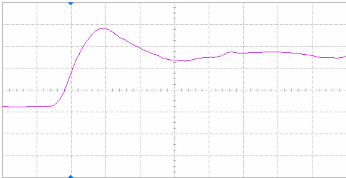
Figure 9(a) DUT 84539 pre-irradiation rising edge, abscissa scale is 2 V/div and ordinate scale is 2 ns/div.
