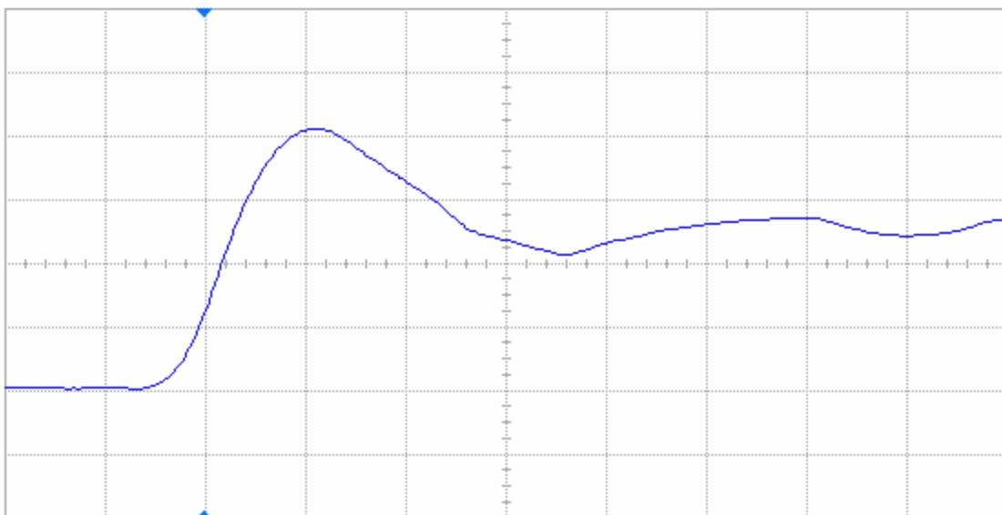
Figure 8(b) DUT 84531 post-annealing rising edge, abscissa scale is 2 V/div and ordinate scale is 2 ns/div.
