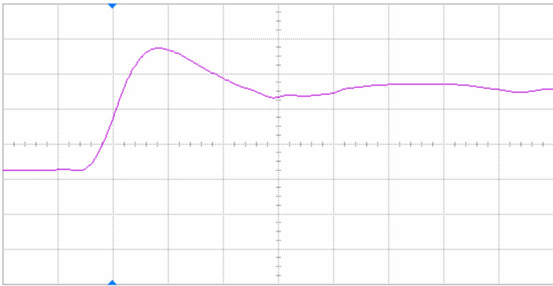
Figure 10(a) DUT 84543 pre-irradiation rising edge, abscissa scale is 2 V/div and ordinate scale is 2 ns/div.
