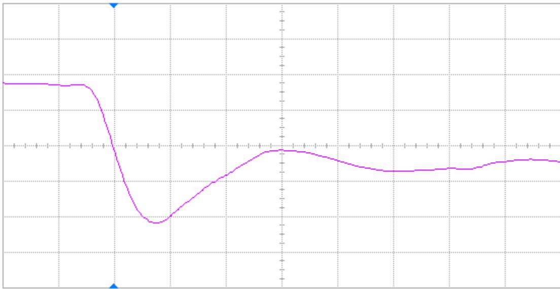
Figure 14(a) DUT 84531 pre-irradiation falling edge, abscissa scale is 2 V/div and ordinate scale is 2 ns/div.
