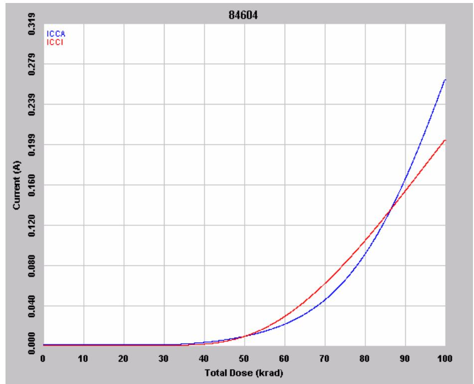
Figure 7 DUT 84604 in-flux  $I_{CCA}$  and  $I_{CCI}$
