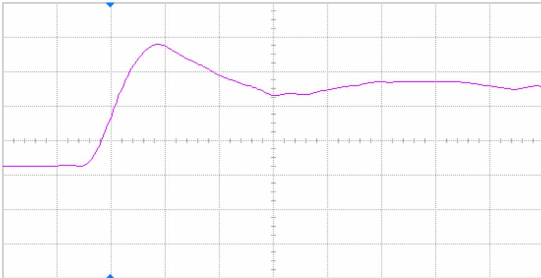
Figure 8(a) DUT 84531 pre-irradiation rising edge, abscissa scale is 2 V/div and ordinate scale is 2 ns/div.
