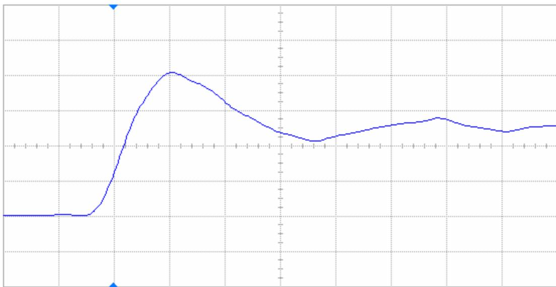
Figure 11(b) DUT 84588 post-annealing rising edge, abscissa scale is 2 V/div and ordinate scale is 2 ns/div.
