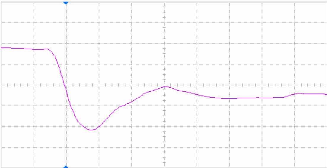
Figure 17(a) DUT 84588 pre-irradiation falling edge, abscissa scale is 2 V/div and ordinate scale is 2 ns/div.
