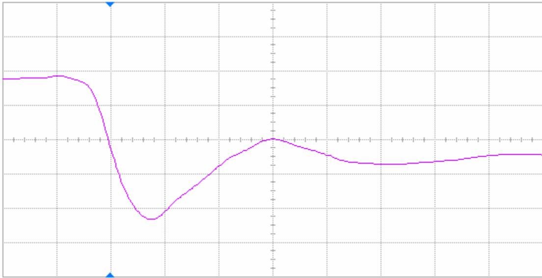
Figure 16(a) DUT 84543 pre-irradiation falling edge, abscissa scale is 2 V/div and ordinate scale is 2 ns/div.
