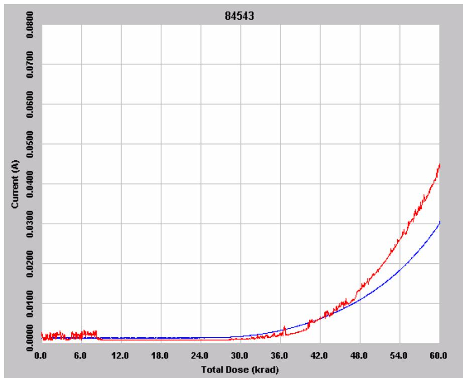
Figure 4 DUT 84543 in-flux  $I_{CCA}$  and  $I_{CCI}$
