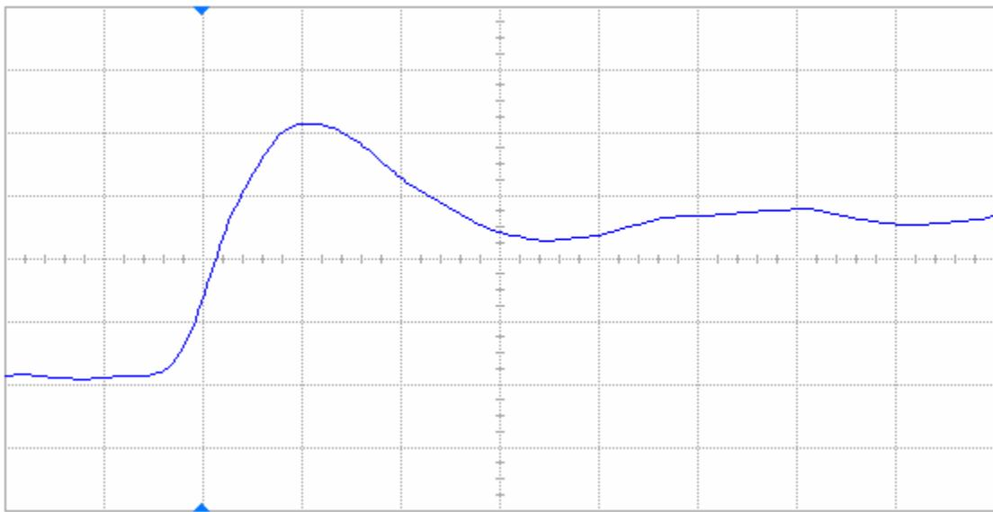
Figure 10(b) DUT 84543 post-annealing rising edge, abscissa scale is 2 V/div and ordinate scale is 2 ns/div.
