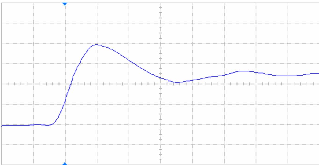
Figure 12(b) DUT 84601 post-irradiation rising edge, abscissa scale is 2 V/div and ordinate scale is 2 ns/div.
