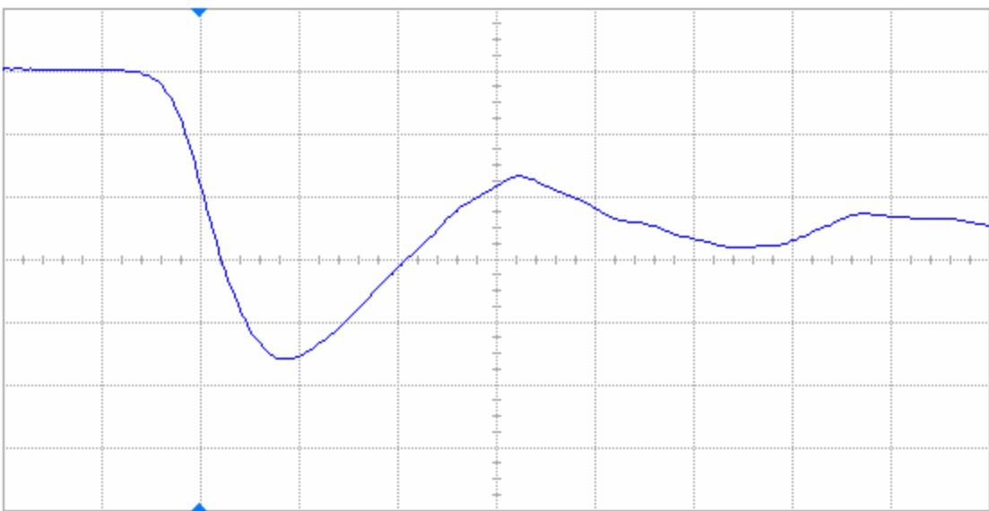
Figure 17(b) DUT 84588 post-irradiation falling edge, abscissa scale is 2 V/div and ordinate scale is 2 ns/div.
