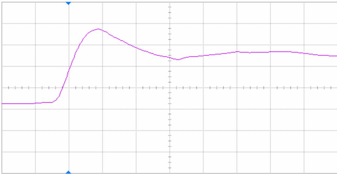
Figure 11(a) DUT 84588 pre-irradiation rising edge, abscissa scale is 2 V/div and ordinate scale is 2 ns/div.
