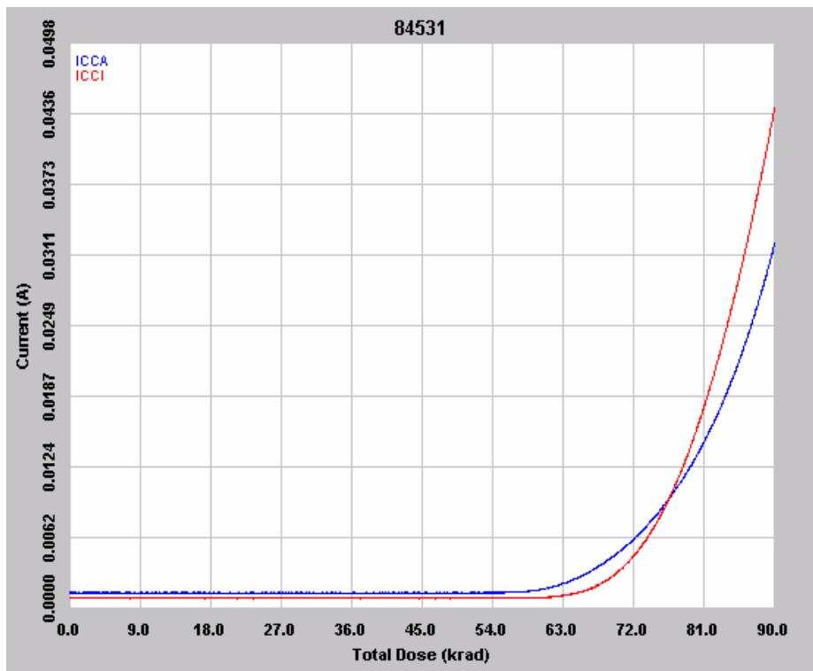
Figure 2 DUT 84531 in-flux I<sub>CCA</sub> and I<sub>CCI</sub>
