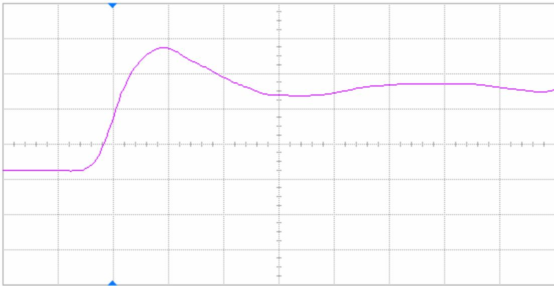
Figure 12(a) DUT 84601 pre-irradiation rising edge, abscissa scale is 2 V/div and ordinate scale is 2 ns/div.
