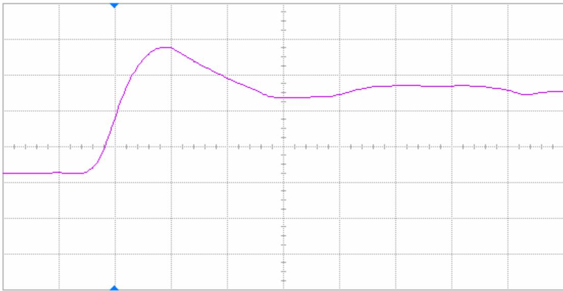
Figure 13(a) DUT 84604 pre-irradiation rising edge, abscissa scale is 2 V/div and ordinate scale is 2 ns/div.
