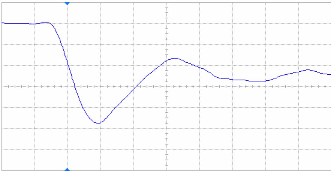
Figure 15(b) DUT 84539 post-annealing falling edge, abscissa scale is 2 V/div and ordinate scale is 2 ns/div.
