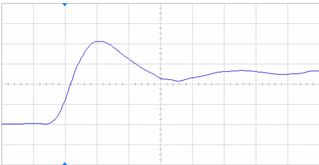
Figure 13(b) DUT 84604 post-irradiation rising edge, abscissa scale is 2 V/div and ordinate scale is 2 ns/div.
