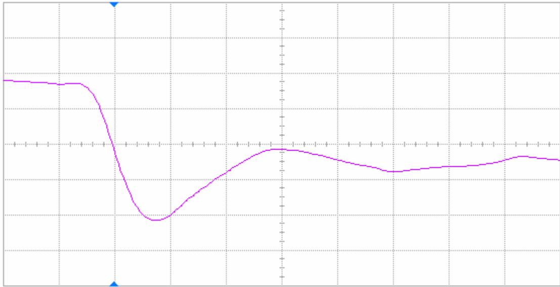
Figure 18(a) DUT 84601 pre-irradiation falling edge, abscissa scale is 2 V/div and ordinate scale is 2 ns/div.
