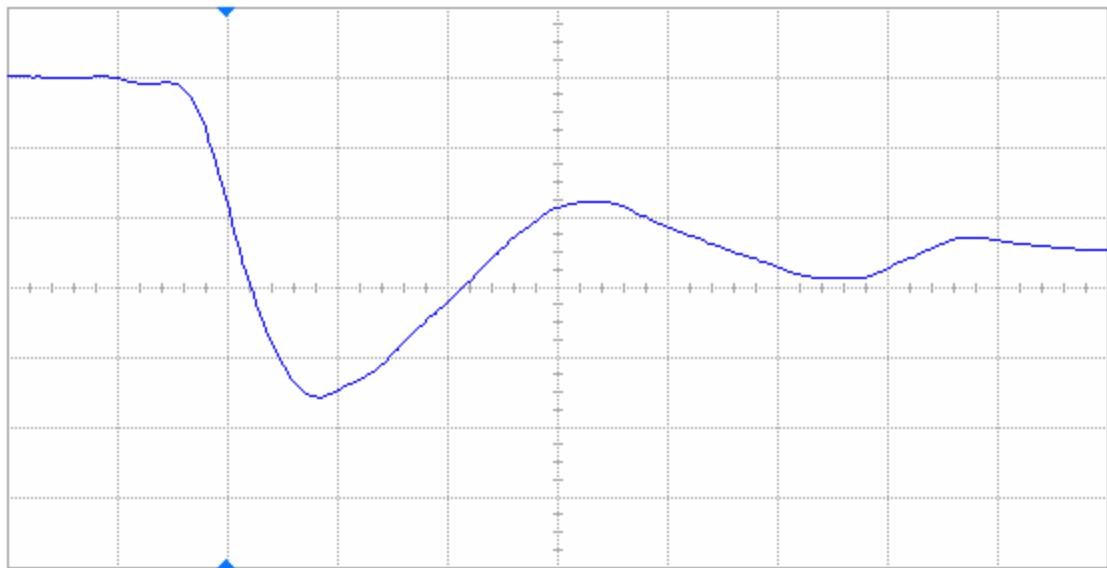
Figure 18(b) DUT 84601 post-irradiation falling edge, abscissa scale is 2 V/div and ordinate scale is 2 ns/div.
