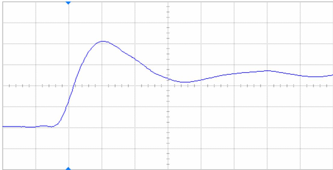
Figure 9(b) DUT 84539 post-annealing rising edge, abscissa scale is 2 V/div and ordinate scale is 2 ns/div.
