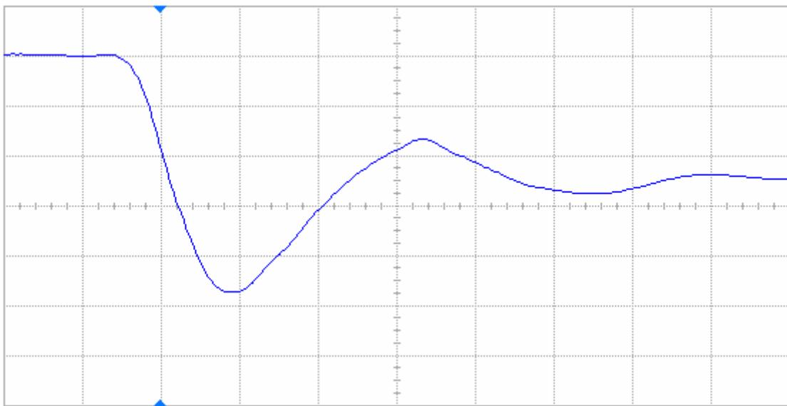
Figure 19(b) DUT 84604 post-irradiation falling edge, abscissa scale is 2 V/div and ordinate scale is 2 ns/div.
