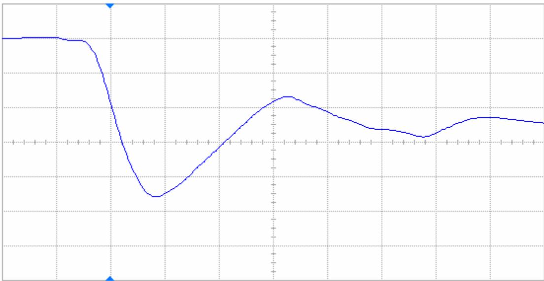
Figure 14(b) DUT 84531 post-annealing falling edge, abscissa scale is 2 V/div and ordinate scale is 2 ns/div.
