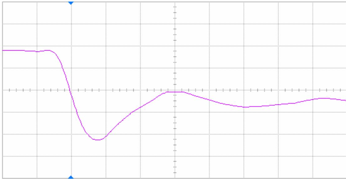
Figure 19(a) DUT 84604 pre-irradiation falling edge, abscissa scale is 2 V/div and ordinate scale is 2 ns/div.
