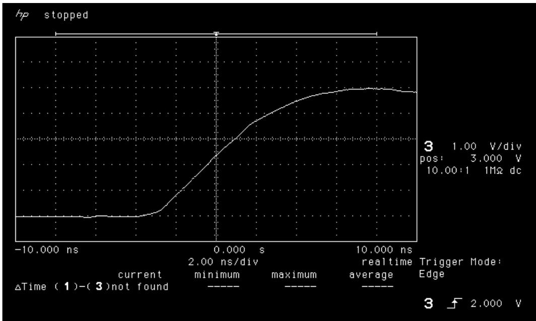
Figure 11b. Rising edge of LAN4706 post-annealing
