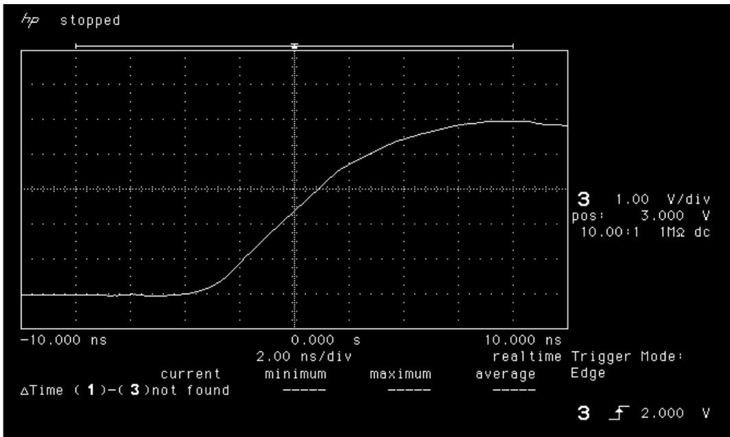
Figure 8b. Rising edge of LAN4703 post-annealing.
