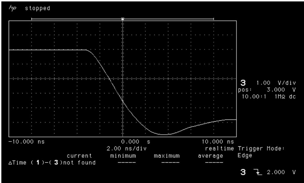
Figure 15a. Falling edge of LAN4706 pre-irradiation
