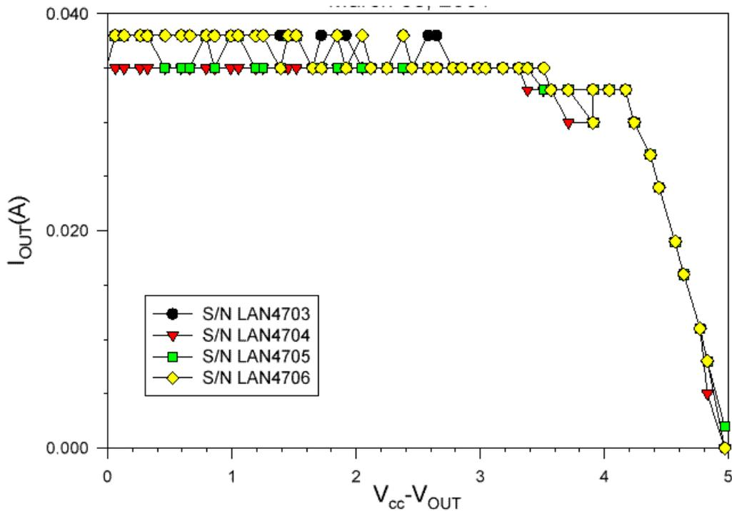
Figure 6b. Post-annealing  $V_{OL}$  characteristic curves.
