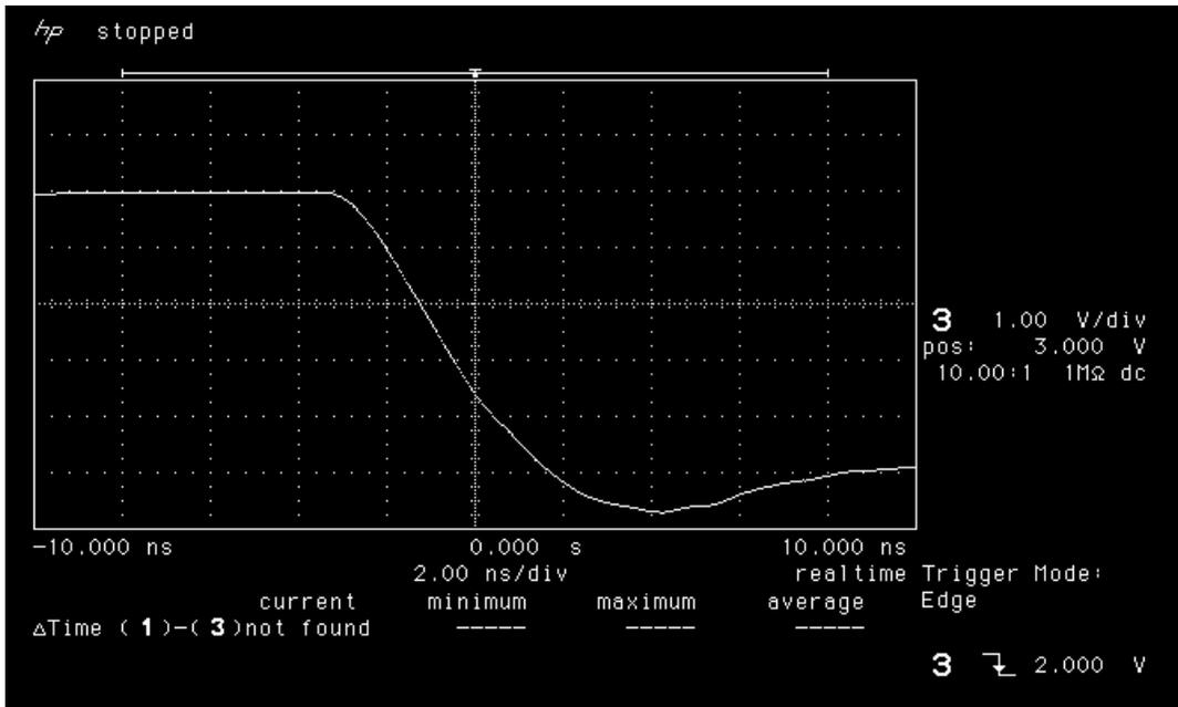
Figure 12a. Falling edge of LAN4703 pre-irradiation
