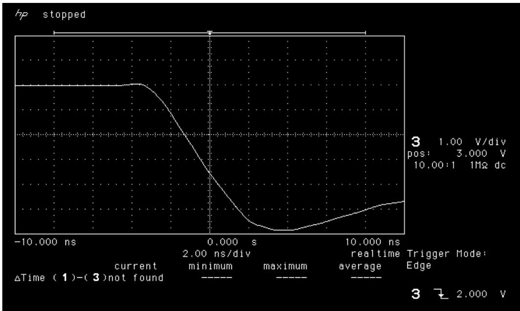
Figure 15b. Falling edge of LAN4706 post-annealing
