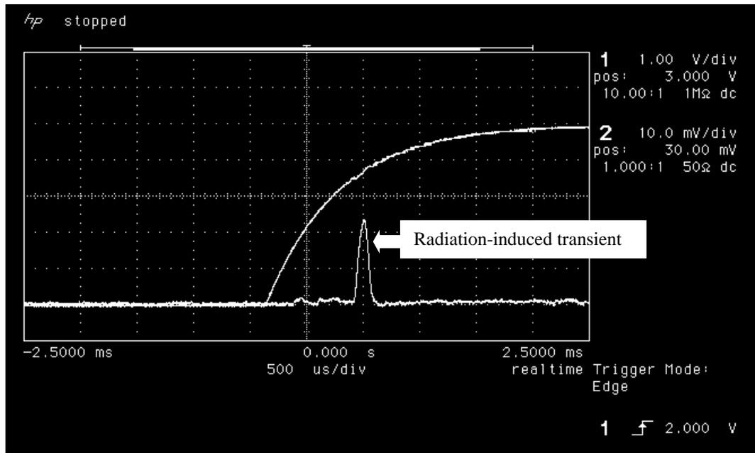
Figure 16b. Power-up transient of LAN4703 post-annealing.
