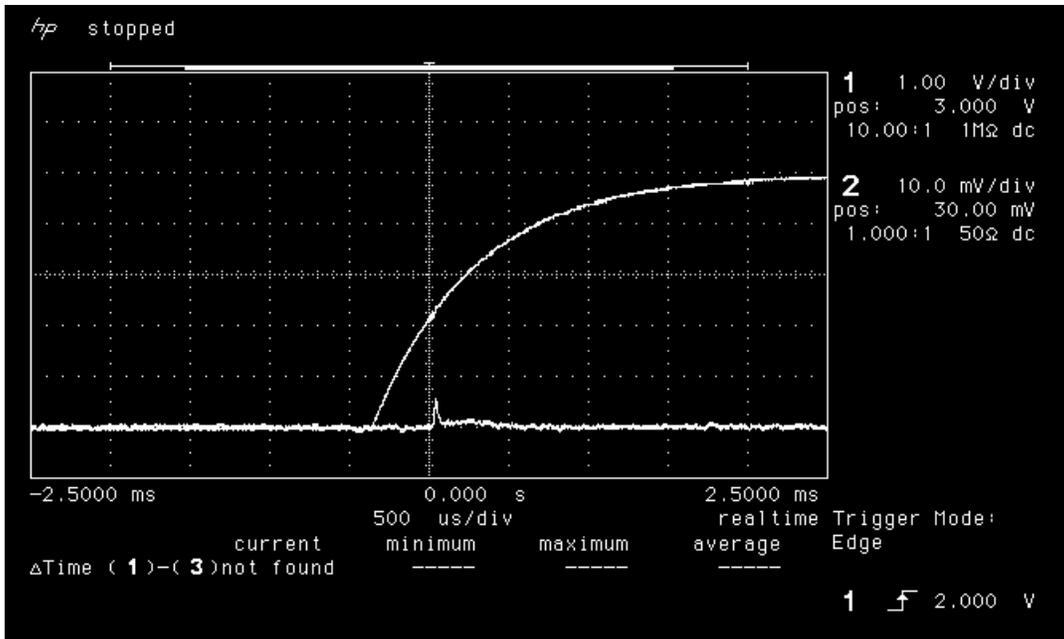
Figure 17a. Power-up transient of LAN4704 pre-irradiation.
