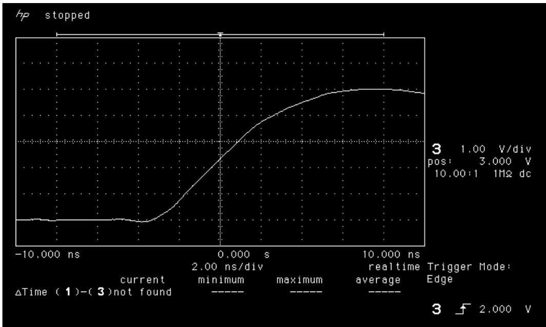
Figure 10b. Rising edge of LAN4705 post-annealing.
