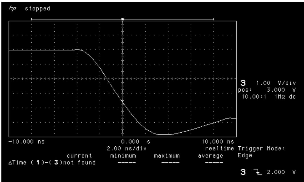
Figure 12b. Falling edge of LAN4703 post-annealing.
