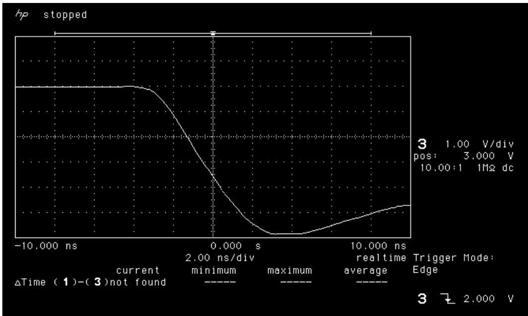
Figure 14b. Falling edge of LAN4705 post-annealing.
