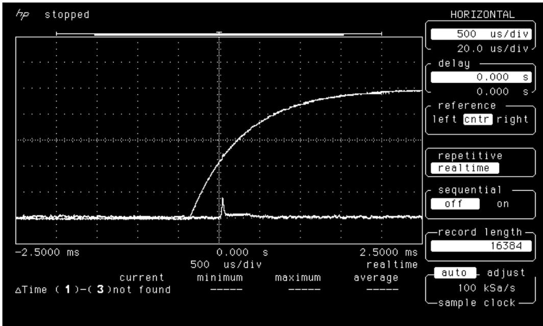
Figure 19a. Power-up transient of LAN4706 pre-irradiation
