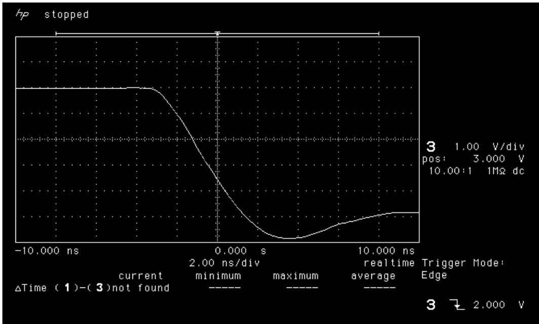
Figure 14a. Falling edge of LAN4705 pre-irradiation.
