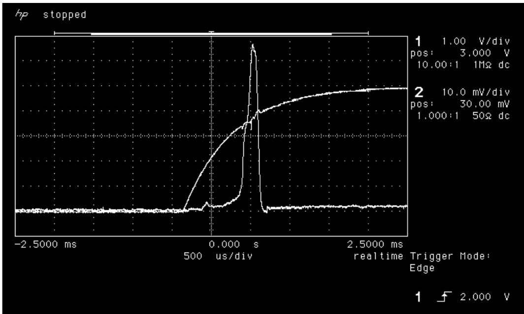
Figure 19b. Power-up transient of LAN4706 post-annealing
