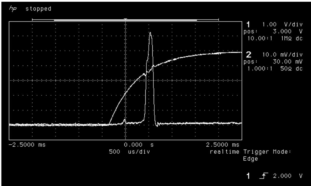
Figure 18b. Power-up transient of LAN4705 post-annealing.
