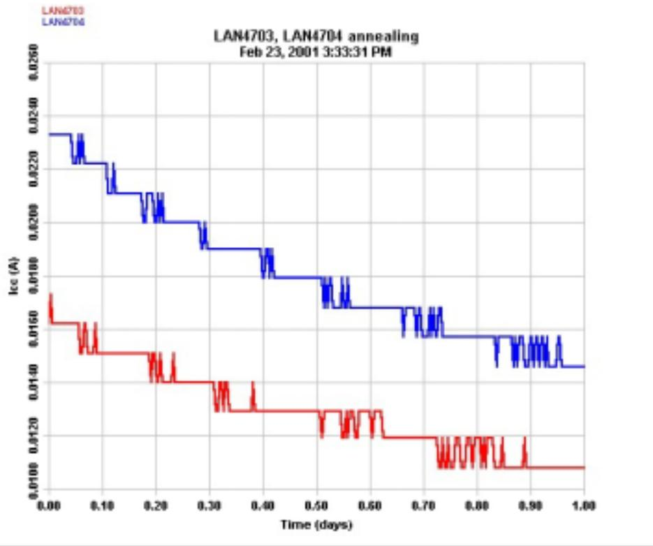
Figure 4. Post-irradiation room temperature biased annealing effects on  $I_{DDSTDY}$  of LAN4703 and LAN4704.
