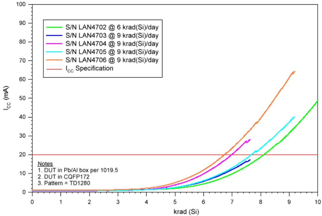
Figure 3. Radiation-induced Delta  $I_{DDstandby}$  ( $I_{CC}$ ) versus total dose for LAN4703, LAN4704, LAN4705 and LAN4706, in-situ monitoring.
