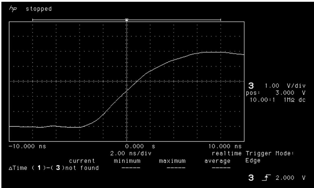
Figure 9b. Rising edge of LAN4704 post-annealing.
