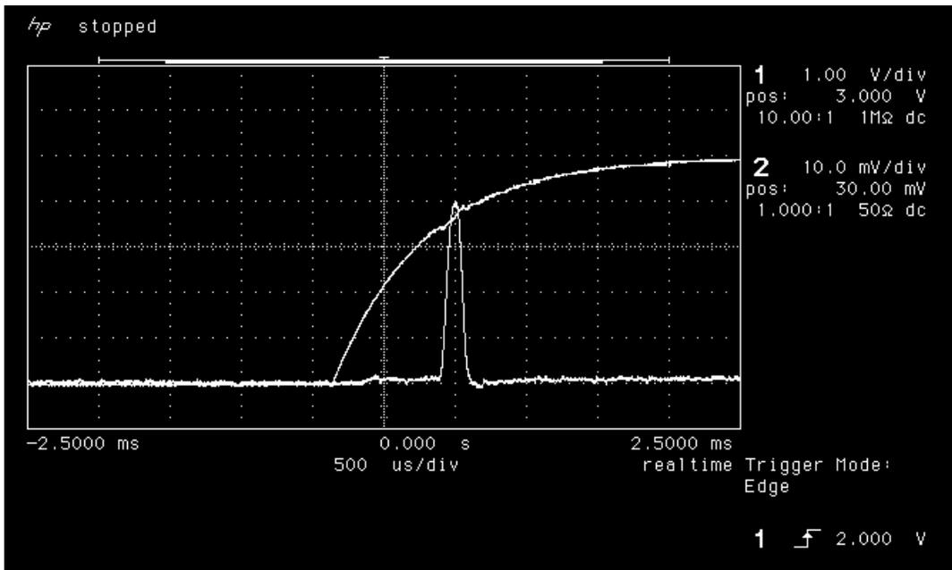
Figure 17b. Power-up transient of LAN4704 post-annealing.
