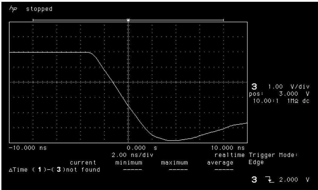
Figure 13b. Falling edge of LAN4704 post-annealing.
