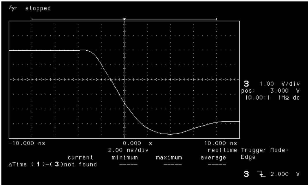
Figure 13a. Falling edge of LAN4704 pre-irradiation.
