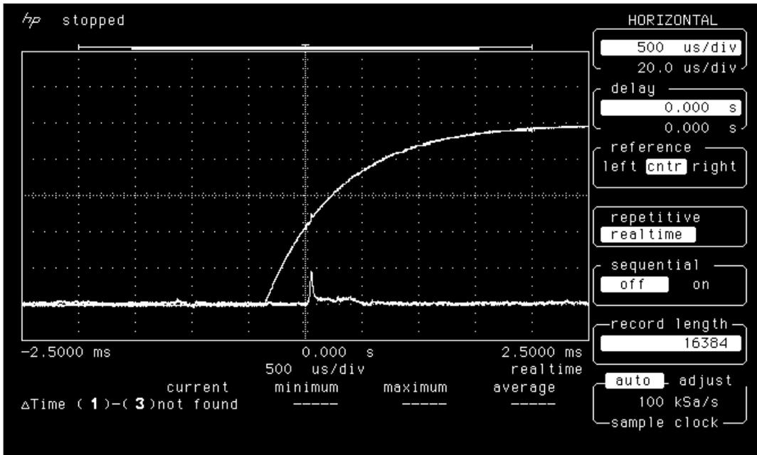
Figure 18a. Power-up transient of LAN4705 pre-irradiation.
