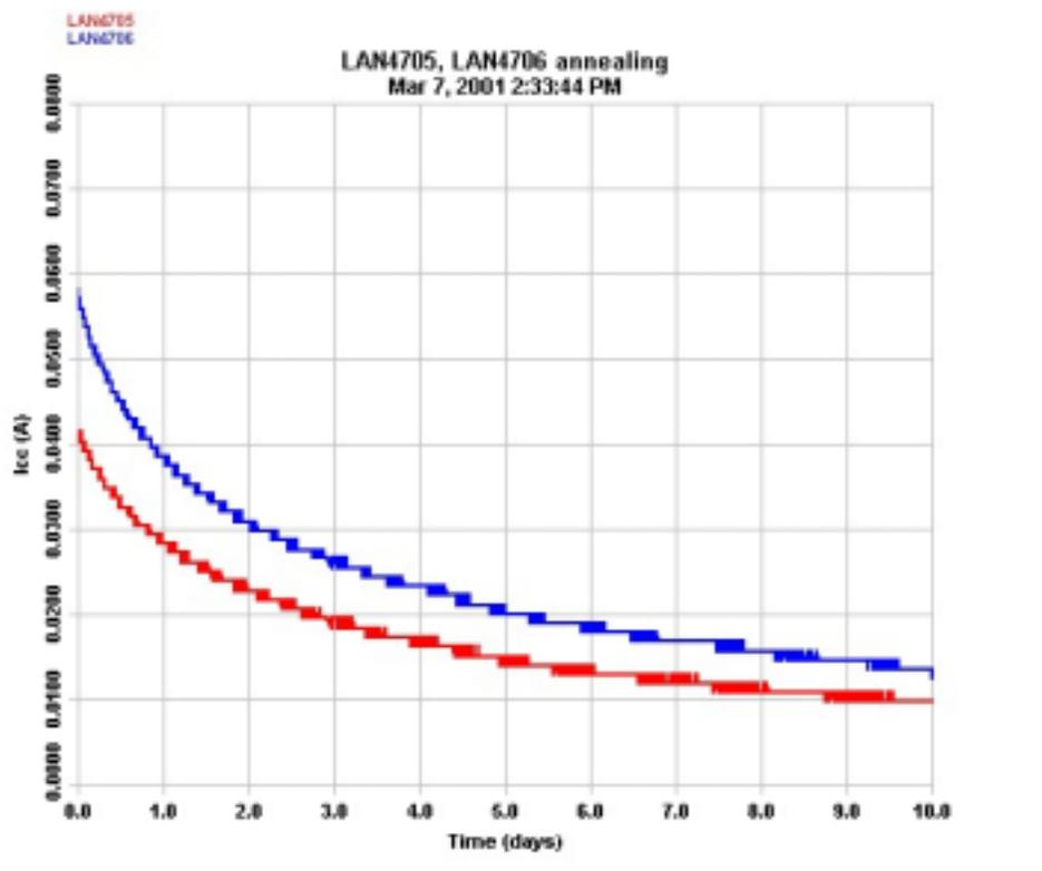
Figure 5. Post-irradiation room temperature biased annealing effects on  $I_{DDSTDY}$  of LAN4705 and LAN4706.
