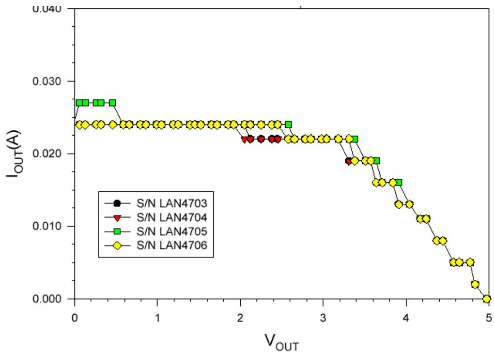
Figure 7b. Post-annealing  $V_{OH}$  characteristic curves.
