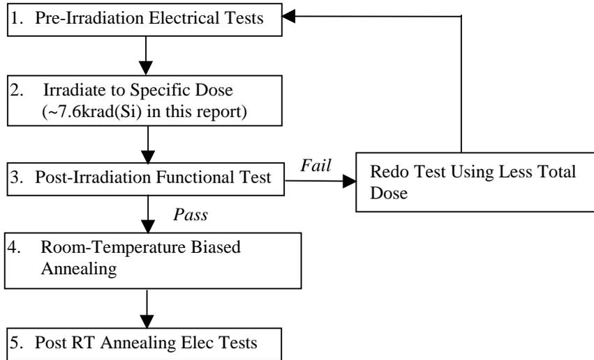
Figure 1. Parametric test flow chart.
