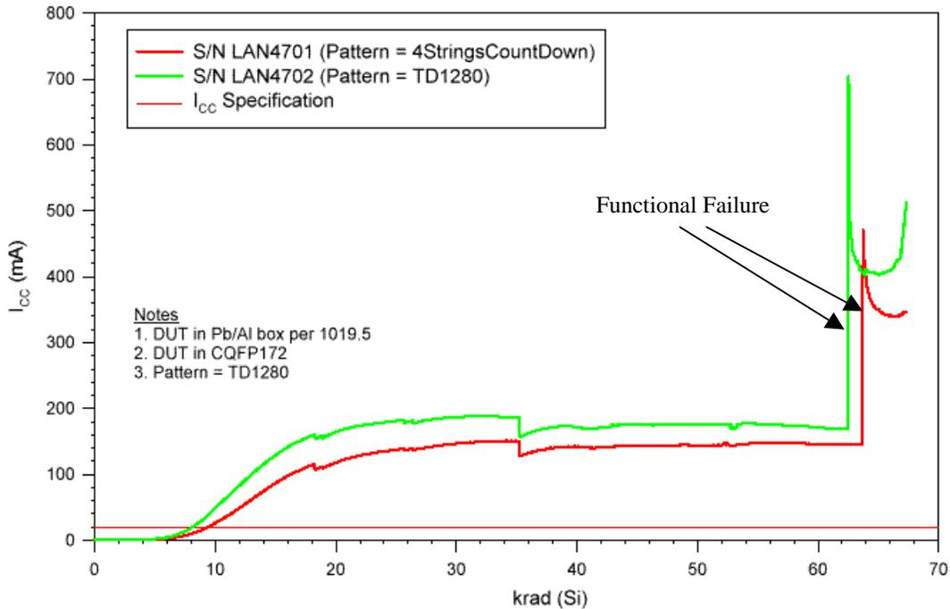
Figure 2. Radiation-induced  $I_{CC}$  (Delta  $I_{CC}$ ) versus total dose for two DUT (LAN4701 and LAN4702).
