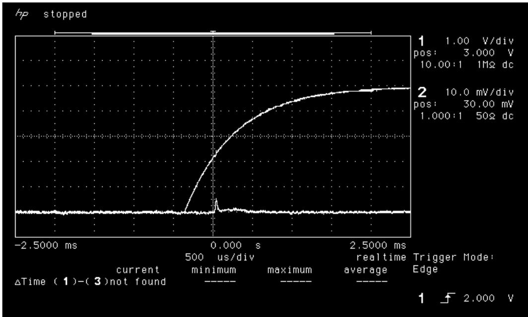
Figure 16a. Power-up transient of LAN4703 pre-irradiation.
