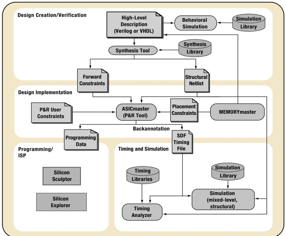
Figure 2: ASICmaster Design Flow
