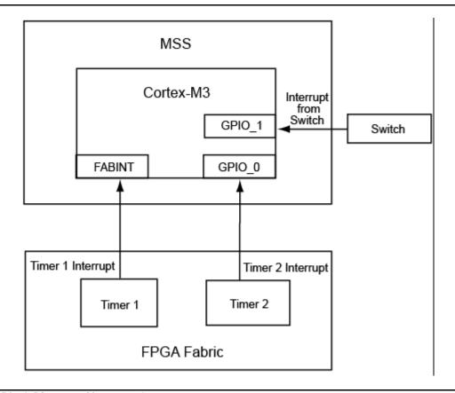
Figure 2 • Block Diagram of Interrupt Generator
