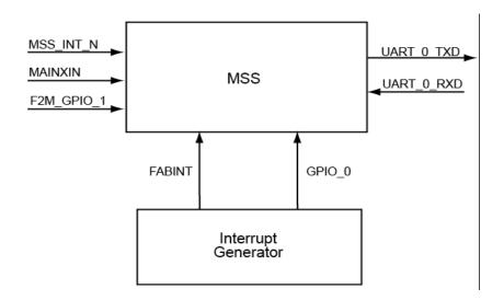
Figure 1 • Interfaces of Interrupt Generator Block with MSS
