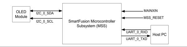
Figure 1 • Top Level Interface Signals
