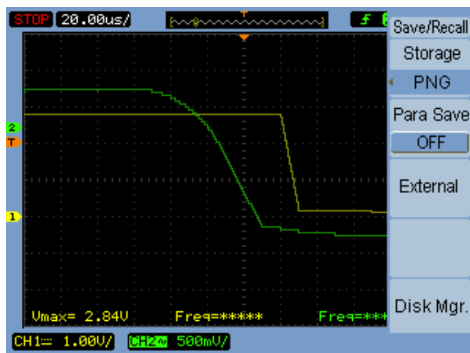
Figure 10 • Falling Edge of Raw Tacho and Filtered Tacho
