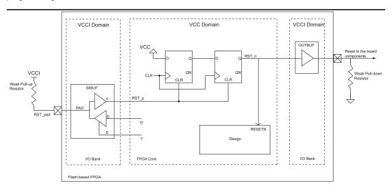
Figure 3 • POR/PPR Signal to Board Components
