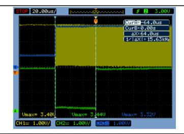
Figure 2 • Pulse Generated Due to Reset from the POR or PPR Circuit
