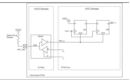
Figure 1 • POR/PPR Circuit Using the BIBUF and External Pull-up Resistor
