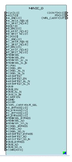
All signals of the MACC block, except CDIN and CDOUT, have optional registers. All registers must use the same clock. Each of the registers has enables and resets that can differ from each other. For a complete list of all the block options and their configurations, refer to the Microsemi documentation.
