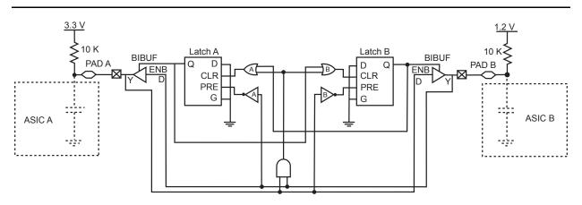
Figure 2 • Bidirectional Level Shifter Circuit Diagram
