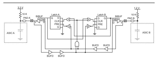
Figure 4 • Bidirectional Level Shifter with Input Path Delay
