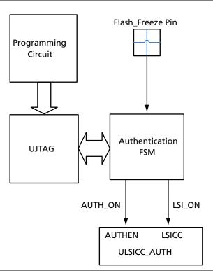
Figure 1 • ULSICC\_AUTH Macro Block Diagram
