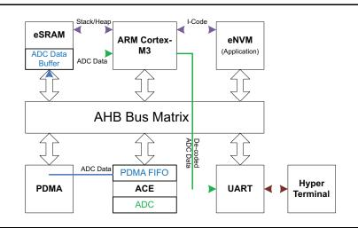
Figure 1 • ACE PDMA Data Flow with MSS eSRAM
