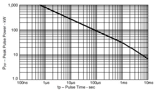
Figure 1 • Figure 1: Peak Pulse Power vs Pulse Time
