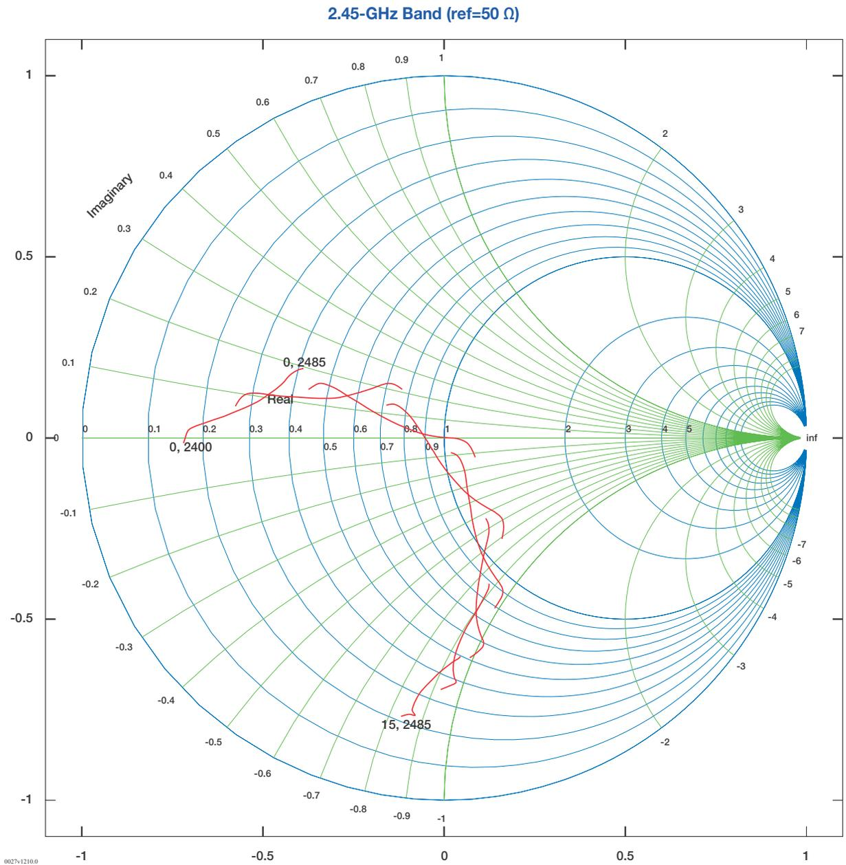
**Figure 2-2 • Combined Port Impedance (2400 to 2485GHz)**
