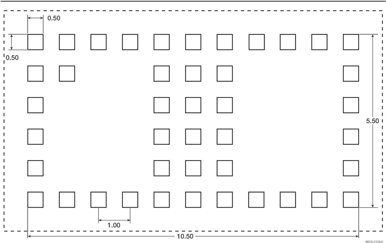
Figure 4-3 • Recommended PCB Layout
