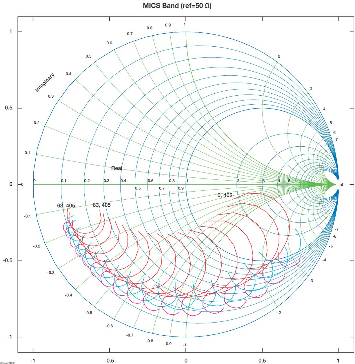
Figure 2-1 • Combined Port Impedance (402 to 405 MHz)
