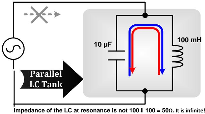
At 159 Hz, the impedances are the same ( $100 \Omega$ ), leading to equal and opposite currents ( $180^\circ$  out of phase with respect to each other), so energy just sloshes back and forth indefinitely. Also no current is drawn from input source (not required), so the source sees in effect, a very high impedance across it.
