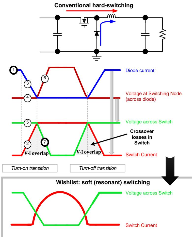
Figure 1: Hard switching compared to resonant (soft) switching
