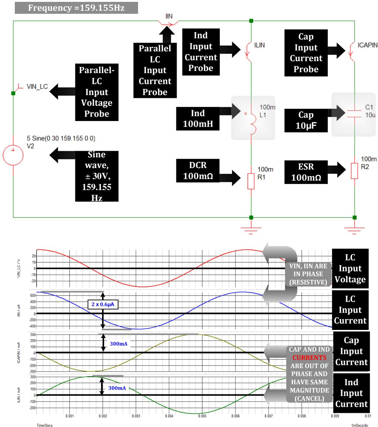
Figure 6: The (almost unloaded) parallel LC at resonance, showing the high circulating currents in L and C
