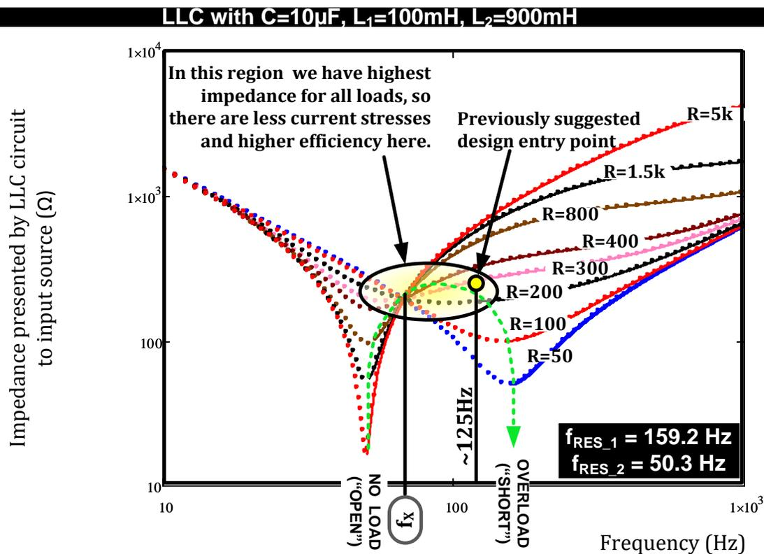
**CAUTION:** Note that these curves only tell us the input impedance for a given load and frequency, so that we can check whether the network appears inductive (for ZVS) or not. They do *not* provide the frequency variation as we change the load or help pick a good design entry point! That is discussed later.
