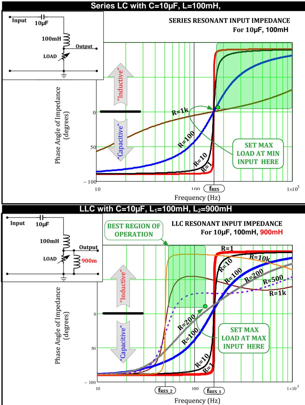
$$f_{RES} = f_{RES_1} = \frac{1}{2\pi\sqrt{LC}} = \frac{1}{2\pi\sqrt{100\text{mH} \times 10\mu\text{F}}} = 159.2\text{Hz}; f_{RES_2} = \frac{1}{2\pi\sqrt{(L_1+L_2)C}} = \frac{1}{2\pi\sqrt{(100+900)\text{mH} \times 10\mu\text{F}}} = 50.3\text{Hz}$$
