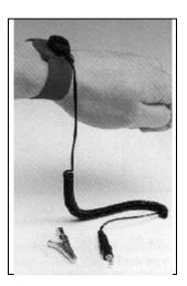
Wrist straps may be selected from a number of approved commercial designs that are acceptable if they provide a path to ground of less than 1 Megaohm from the operator's free hand exclusive of the limiting resistor. Detachable connections are employed by Zarlink with a breakaway force of 5lb (2.3kg).
