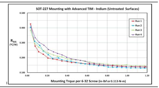
Figure 5 · Thermal resistance vs. mounting torque with advanced TIM - Indium and untreated surfaces.
