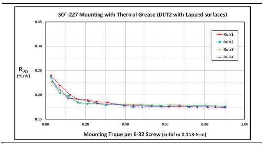
Figure 4 · Thermal resistance vs. mounting torque with Thermal Grease TIM and treated surfaces (DUT 2).
