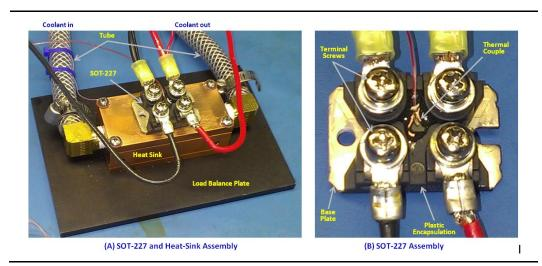
Figure 7 · Heat sink and SOT-227 assemblies of the thermal resistance vs. mounting pressure measurement.
