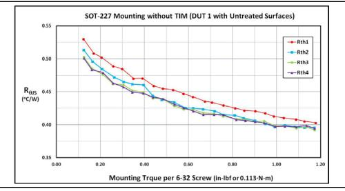
Figure 8 · Thermal resistance vs. mounting torque without TIM and untreated surfaces.
