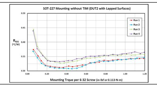
Figure 9 · Thermal resistance vs. mounting torque without TIM and treated surfaces.
