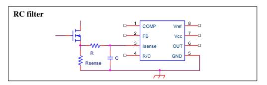
Figure 5. Filtering of Rsense signal
