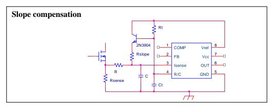
Figure 6. Adding Slope Compensation
