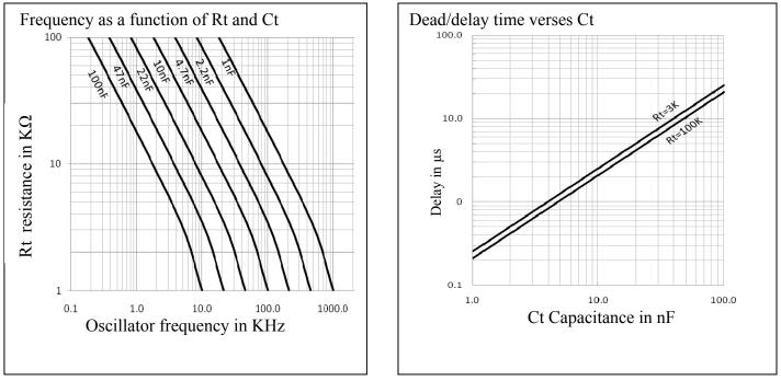
Figure 3. Oscillator Frequency verse Rt and Ct
