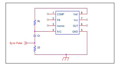
Figure 8. Synchronization of oscillators.
