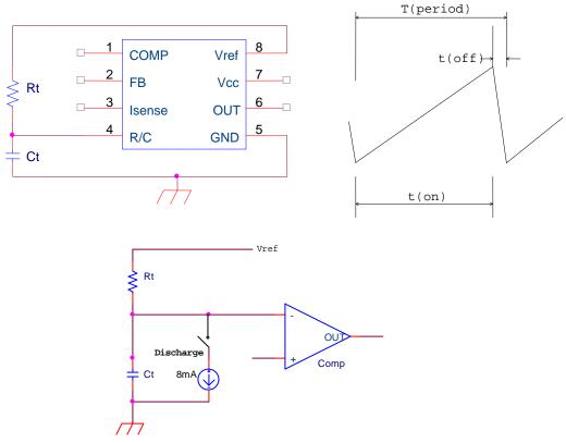
Figure 2. Oscillator Operation
