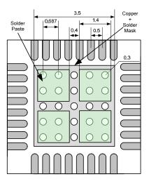
Figure 10: PD70201ILQ Recommended PCB Layout for Thermal Pad Array (mm)
