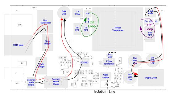
Figure 2: PD70201EVB60F12 EVB power loops and power flow
