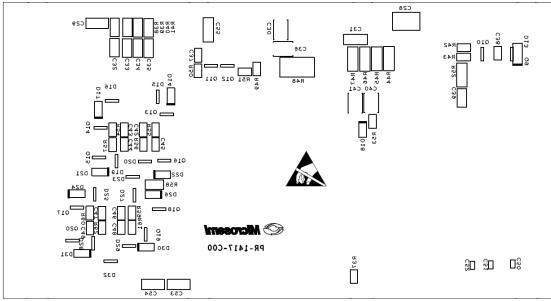
Figure 18: PD70201EVB60F12 EVB PCB Silk Bottom (Mirror)
