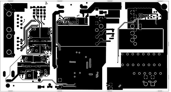
Figure 17: PD70201EVB60F12 EVB PCB Bottom (Layer 4)
