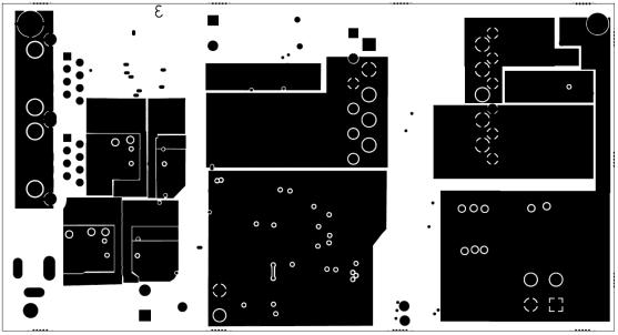
Figure 16: PD70201EVB60F12 EVB PCB Layer 3
