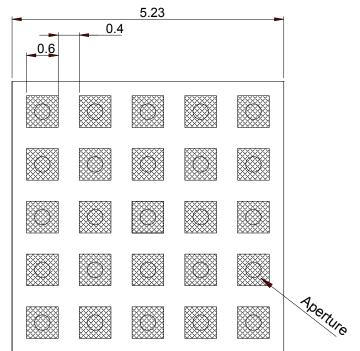
Figure 12: LX23214ILQ Recommended PCB Layout for Thermal Pad Array Footprint (PS)
