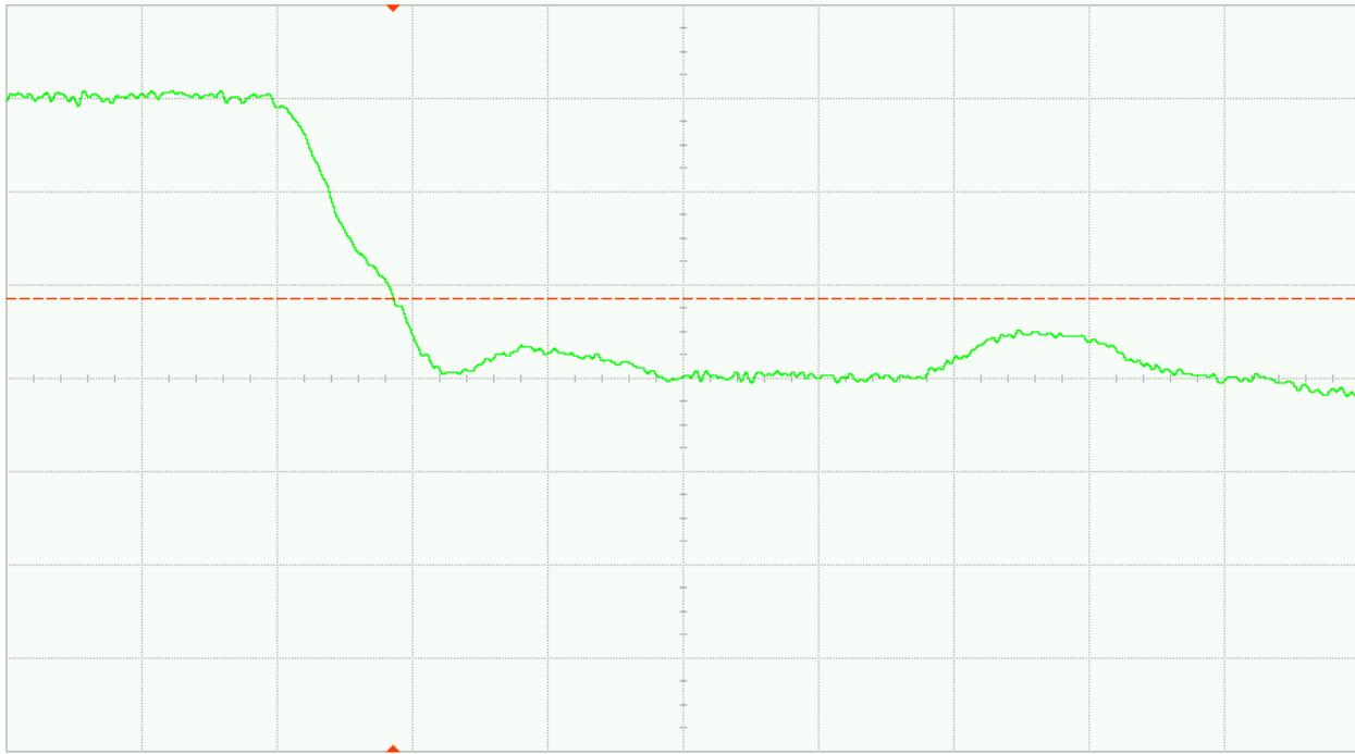
Fig. 34 (a). DUT 07596 pre-irradiation falling edge, abscissa scale is 1V/div and ordinate scale is 2ns/div
