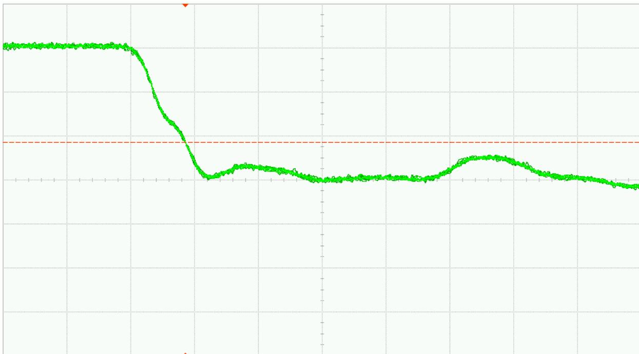
Fig. 32 (b). DUT 07573 post-annealing falling edge, abscissa scale is 1V/div and ordinate scale is 2ns/div
