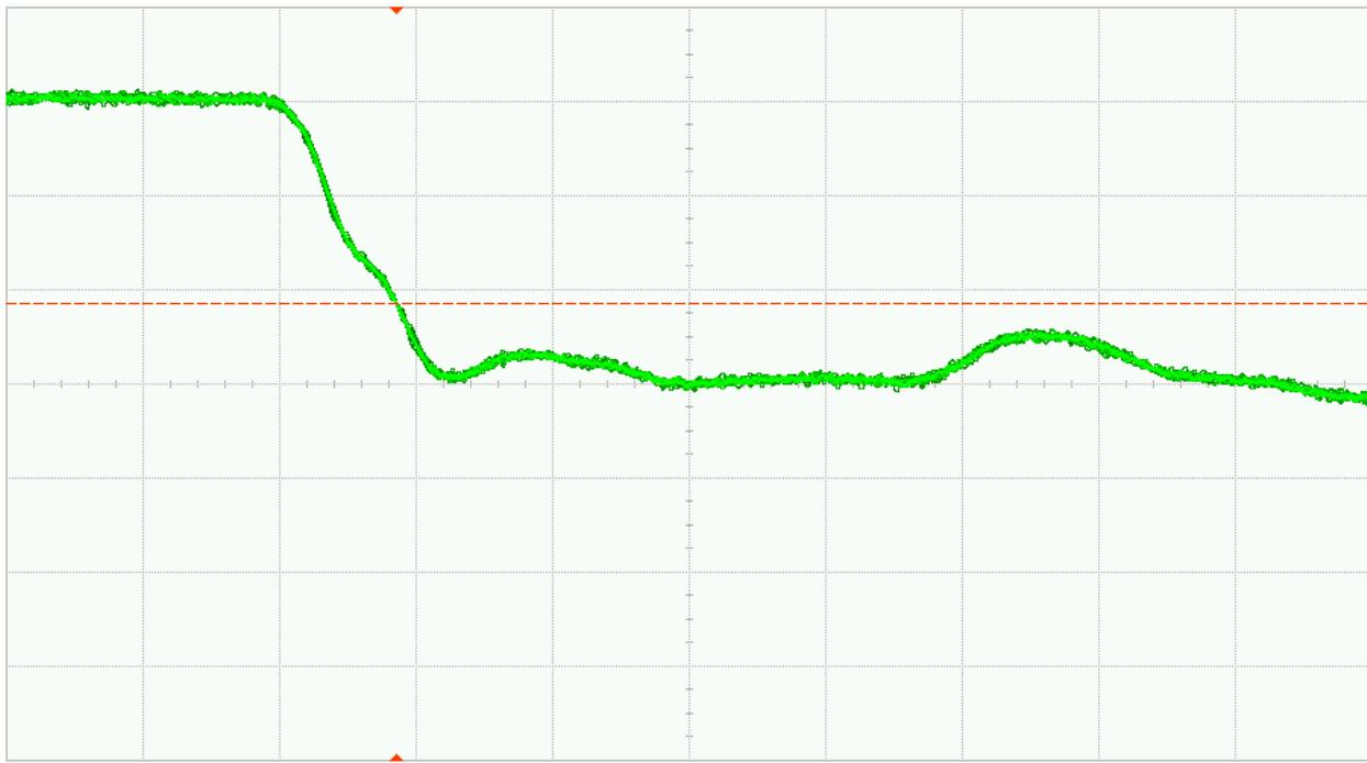
Fig. 33 (a). DUT 07585 pre-irradiation falling edge, abscissa scale is 1V/div and ordinate scale is 2ns/div
