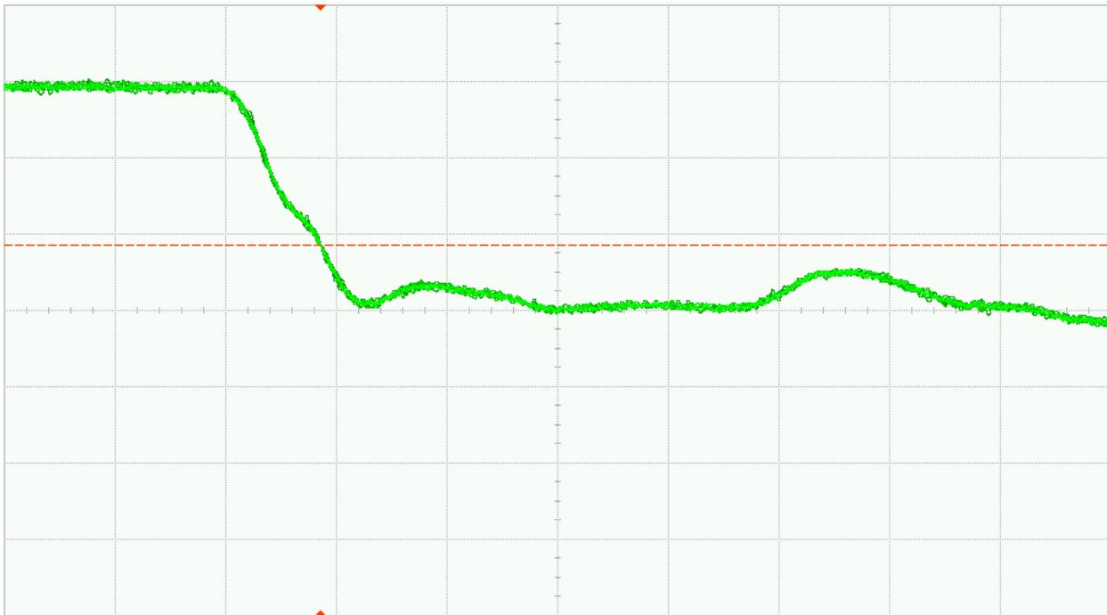
Fig. 33 (b). DUT 01027 post-annealing falling edge, abscissa scale is 1V/div and ordinate scale is 2ns/div
