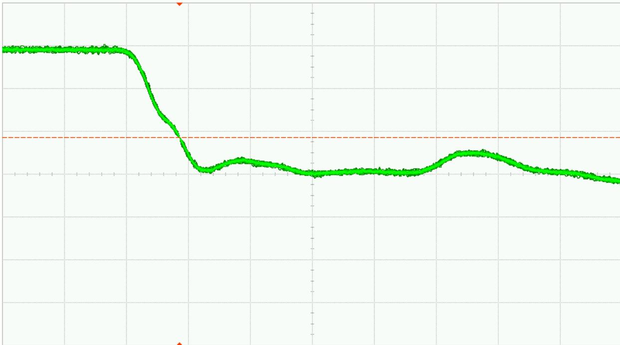
Fig. 32 (b). DUT 01020 post-annealing falling edge, abscissa scale is 1V/div and ordinate scale is 2ns/div
