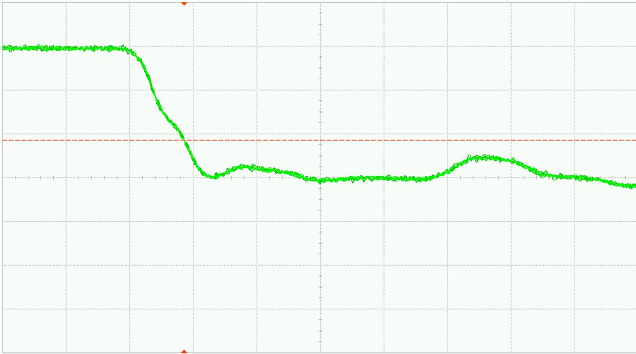
Fig. 33 (a). DUT 01027 pre-irradiation falling edge, abscissa scale is 1V/div and ordinate scale is 2ns/div
