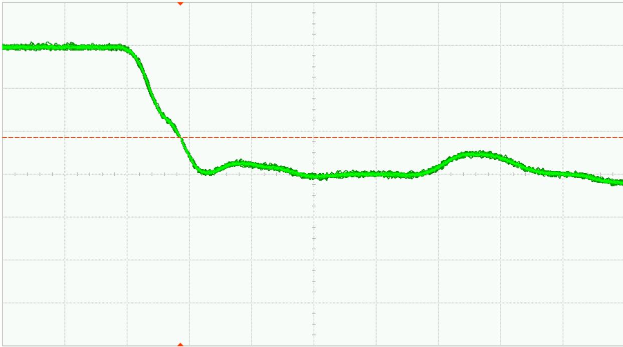
Fig. 36 (a). DUT 01153 pre-irradiation falling edge, abscissa scale is 1V/div and ordinate scale is 2ns/div
