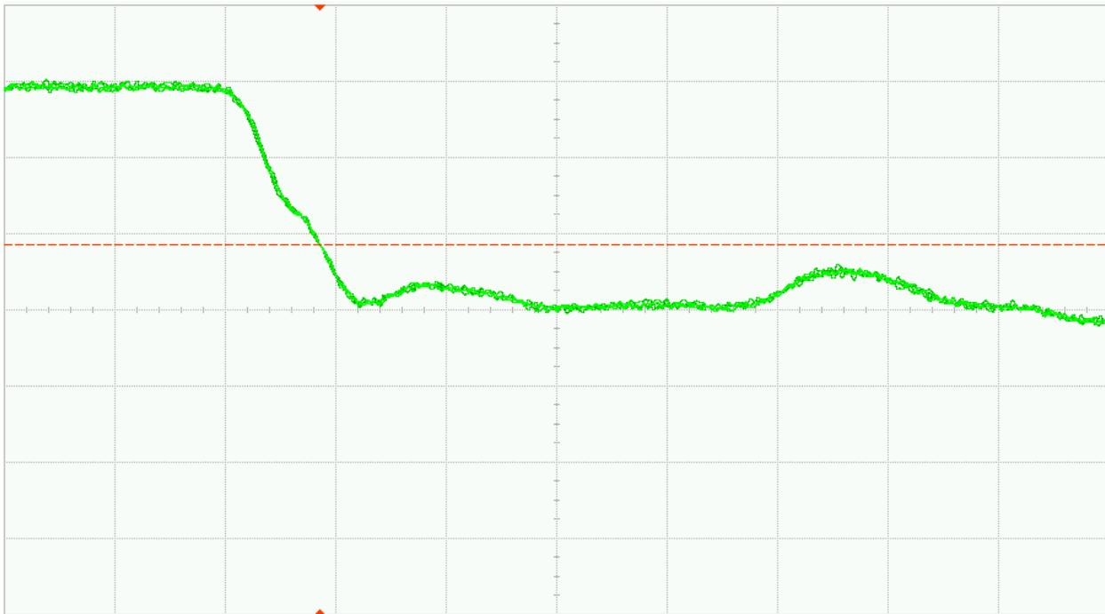
Fig. 37 (b). DUT 01167 post-annealing falling edge, abscissa scale is 1V/div and ordinate scale is 2ns/div
