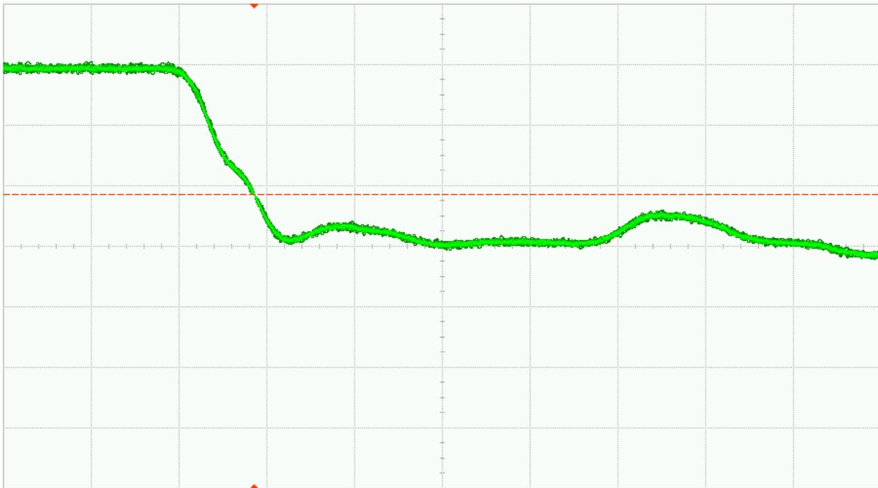
Fig. 36 (b). DUT 01153 post-annealing falling edge, abscissa scale is 1V/div and ordinate scale is 2ns/div
