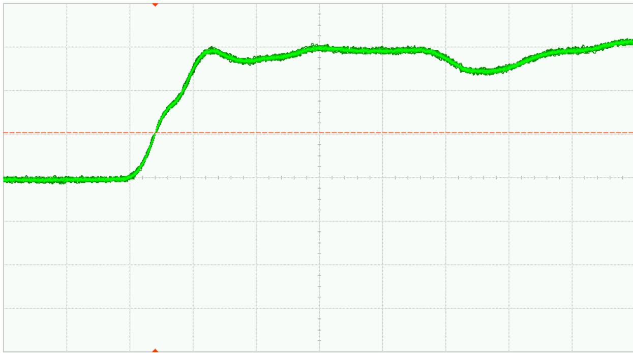
Fig. 28 (a). DUT 01033 pre-irradiation rising edge, abscissa scale is 1V/div and ordinate scale is 2ns/div
