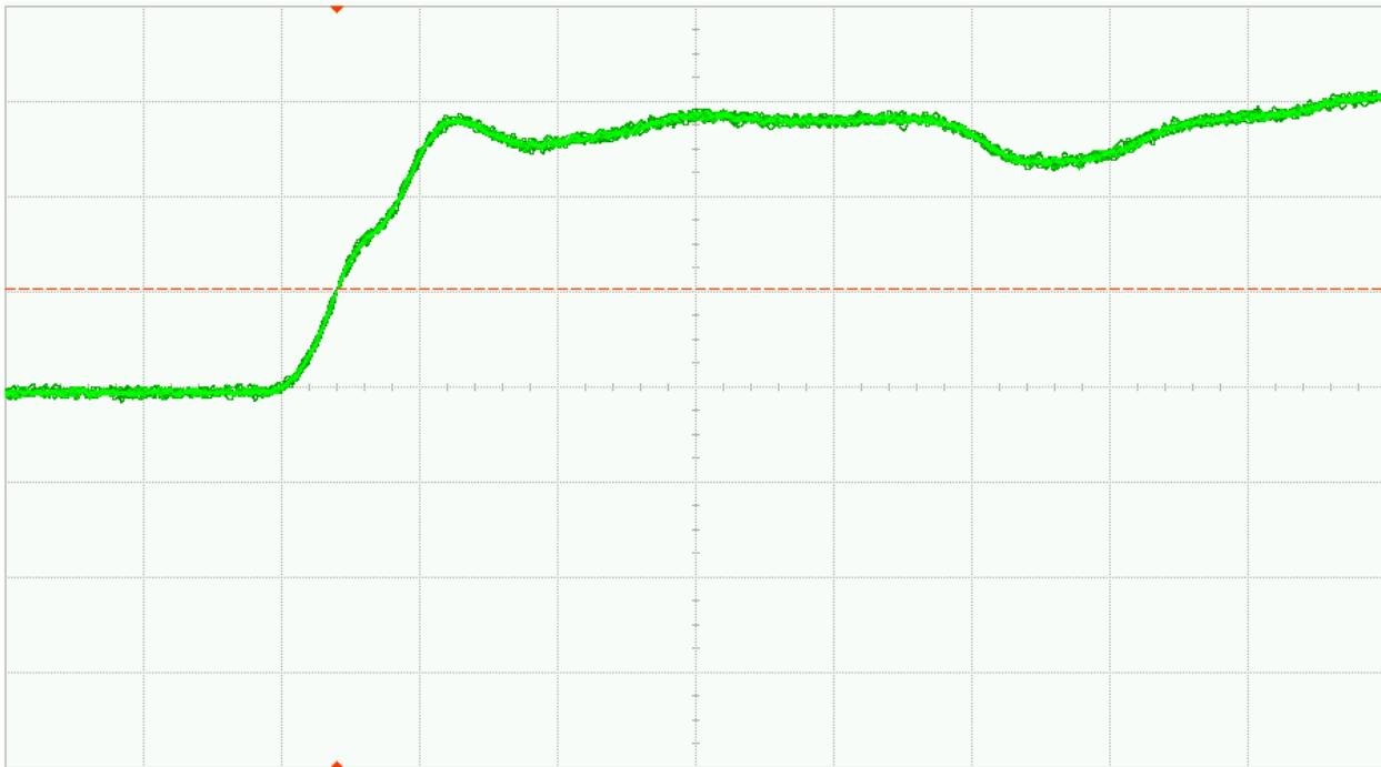
Fig. 30 (b). DUT 01153 post-annealing rising edge, abscissa scale is 1V/div and ordinate scale is 2ns/div
