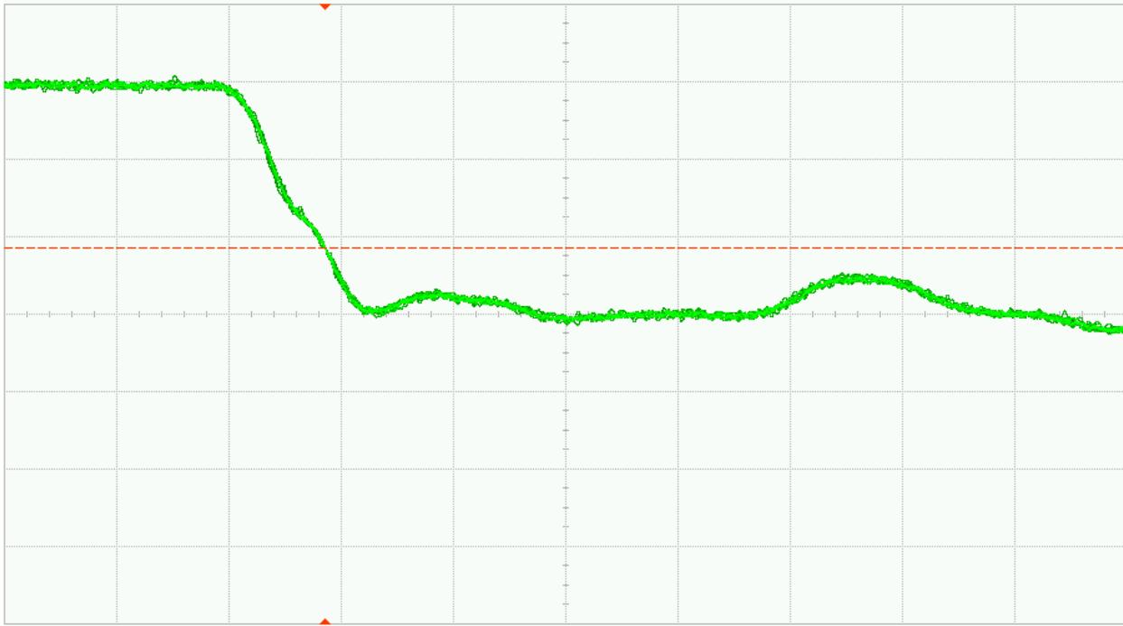
Fig. 37 (a). DUT 01167 pre-irradiation falling edge, abscissa scale is 1V/div and ordinate scale is 2ns/div
