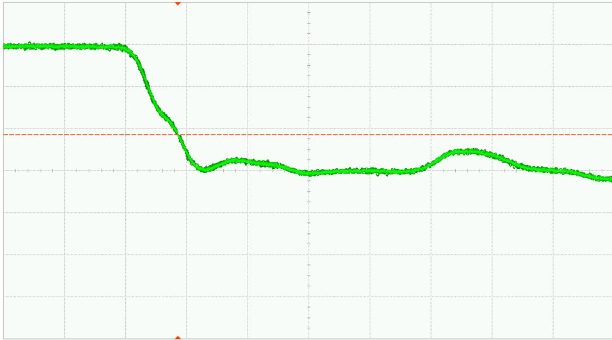
Fig. 35 (a). DUT 01042 pre-irradiation falling edge, abscissa scale is 1V/div and ordinate scale is 2ns/div
