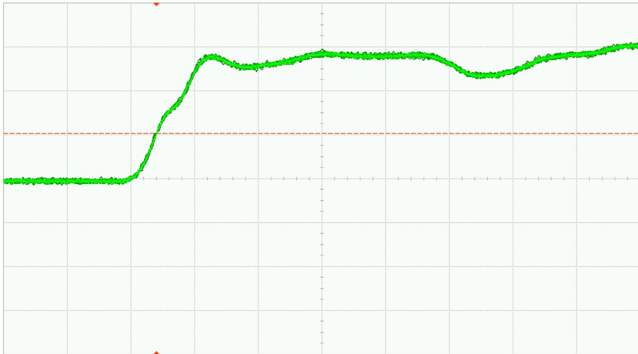
Fig. 31 (b). DUT 01167 post-annealing rising edge, abscissa scale is 1V/div and ordinate scale is 2ns/div
