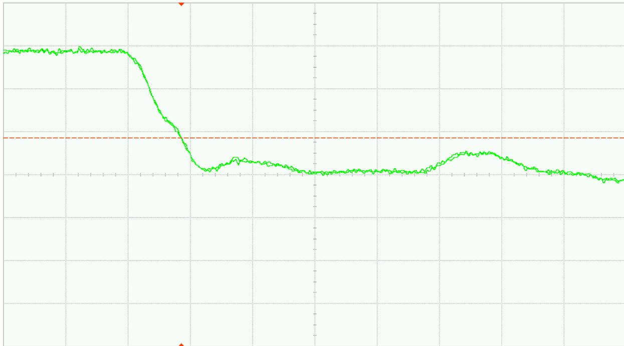
Fig. 34 (b). DUT 01033 post-annealing falling edge, abscissa scale is 1V/div and ordinate scale is 2ns/div
