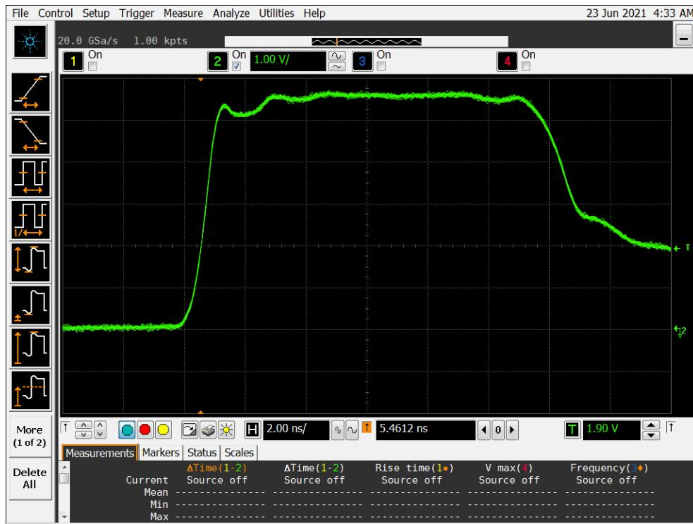
Figure 9a DUT 17070 Pre-Irradiation Rising Edge
