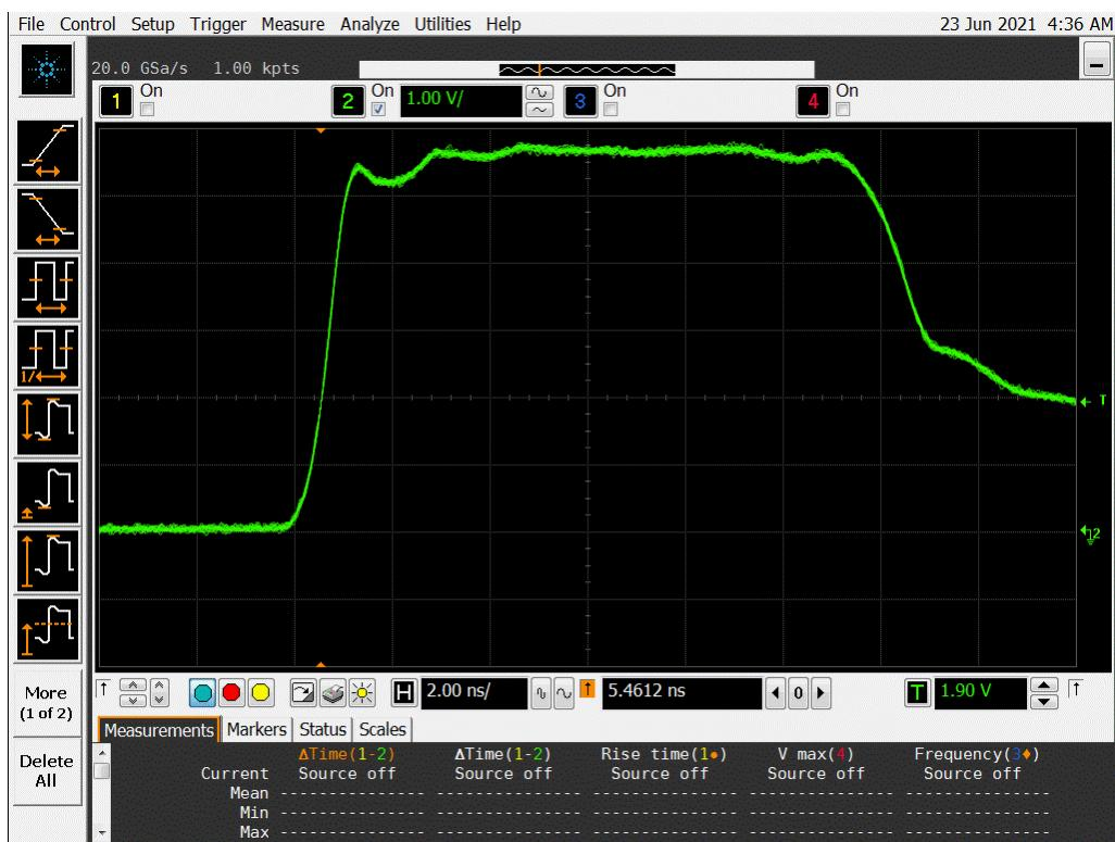
**Figure 10a DUT 17097 Pre-Irradiation Rising Edge**
