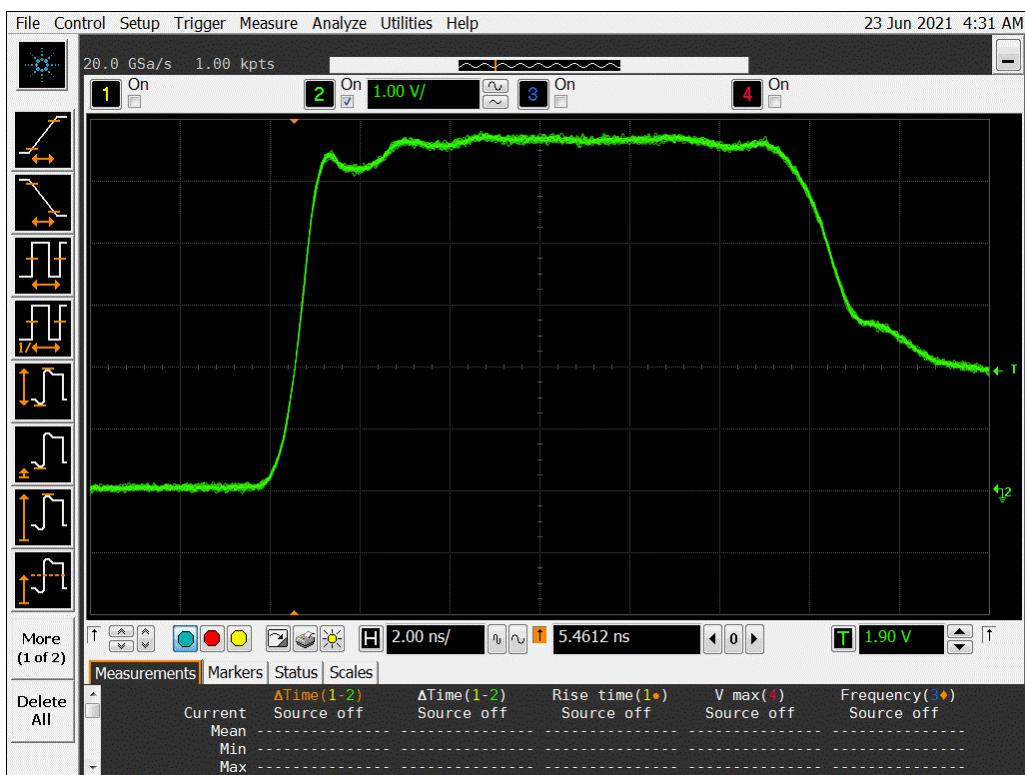
**Figure 12a DUT 17069 Pre-Irradiation Rising Edge**
