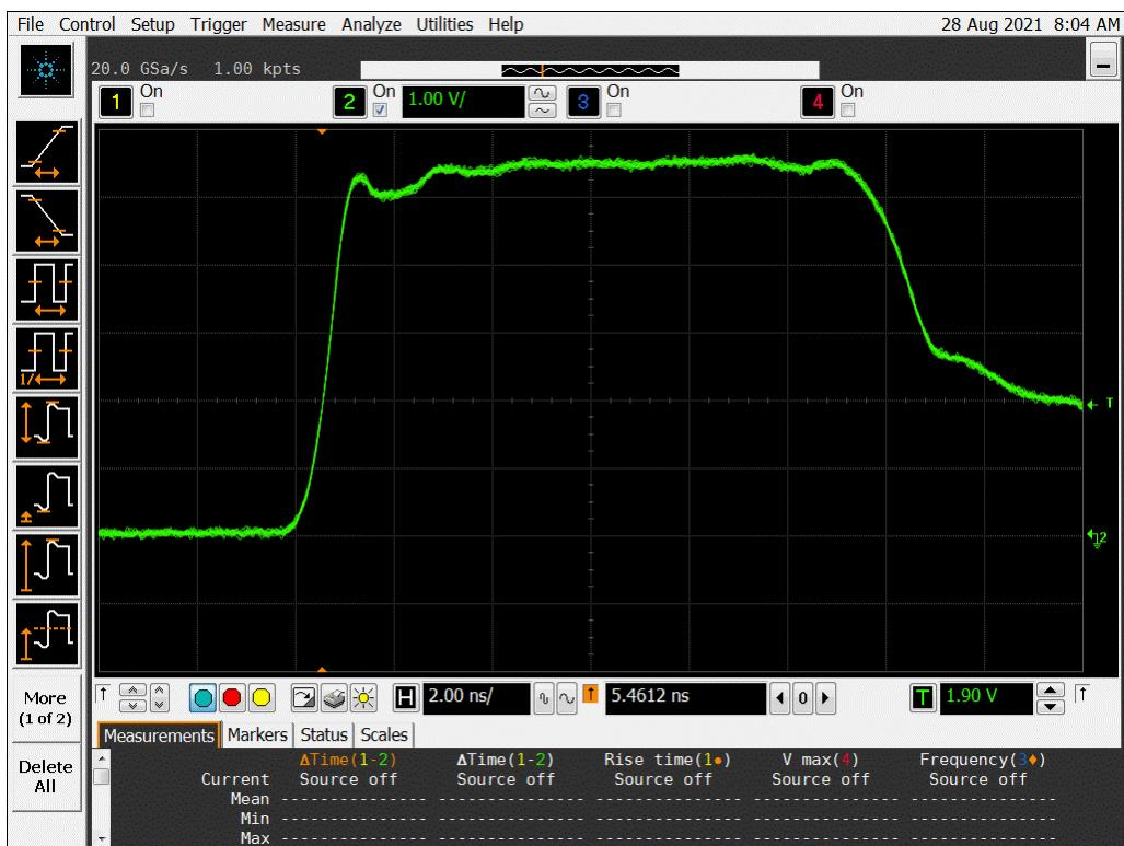
Figure 14b DUT 17056 Post-Annealing Rising Edge
