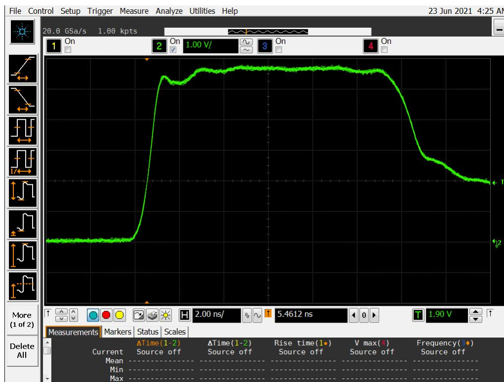
**Figure 13a DUT 17055 Pre-Irradiation Rising Edge**
