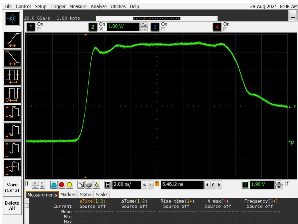
**Figure 12b DUT 17069 Post-Annealing Rising Edge**
