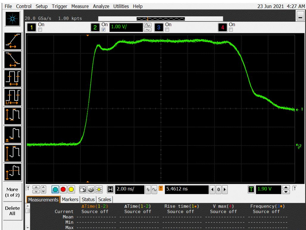
Figure 14a DUT 17056 Pre-Irradiation Rising Edge
