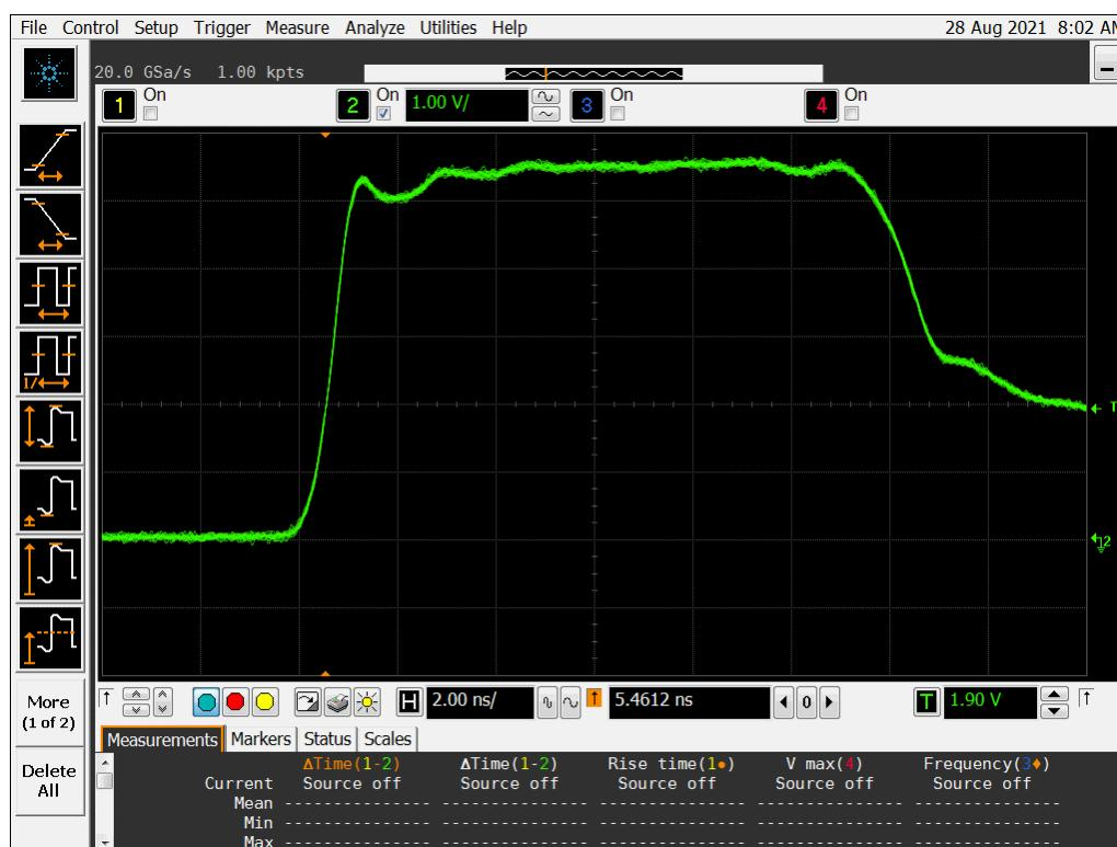
**Figure 13b DUT 17055 Post-Annealing Rising Edge**
