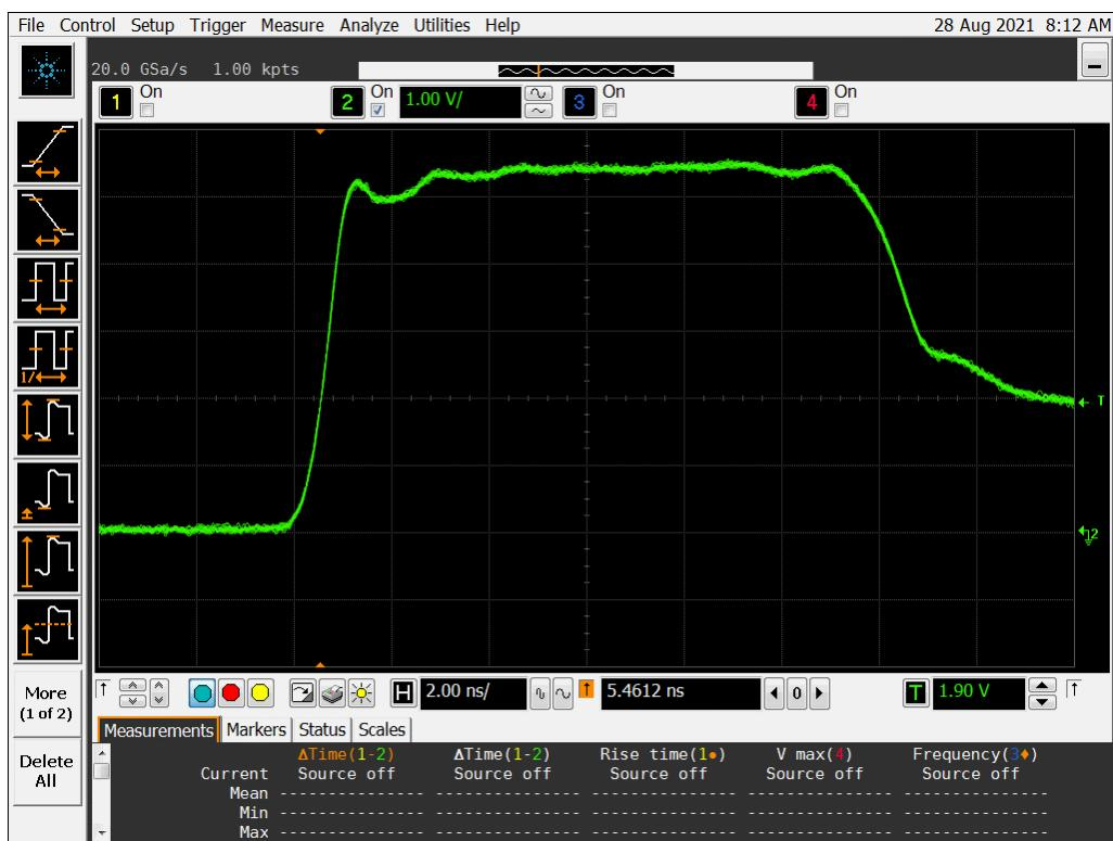
**Figure 10b DUT 17097 Post-Annealing Rising Edge**
