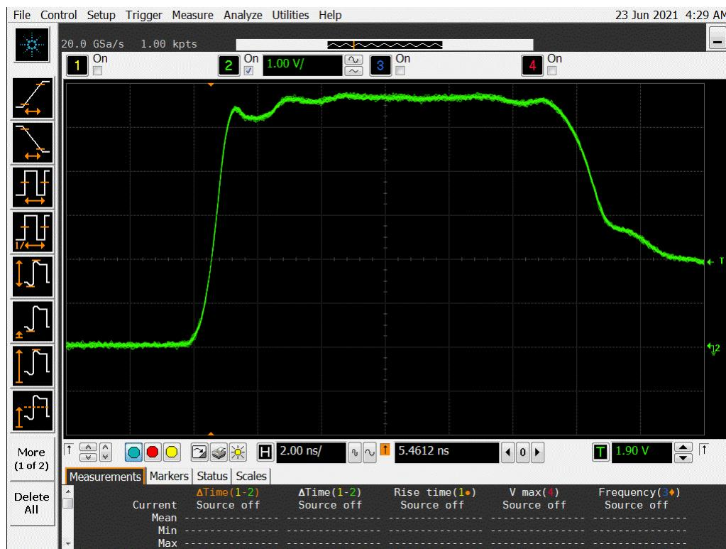
**Figure 11a DUT 17068 Pre-Radiation Rising Edge**
