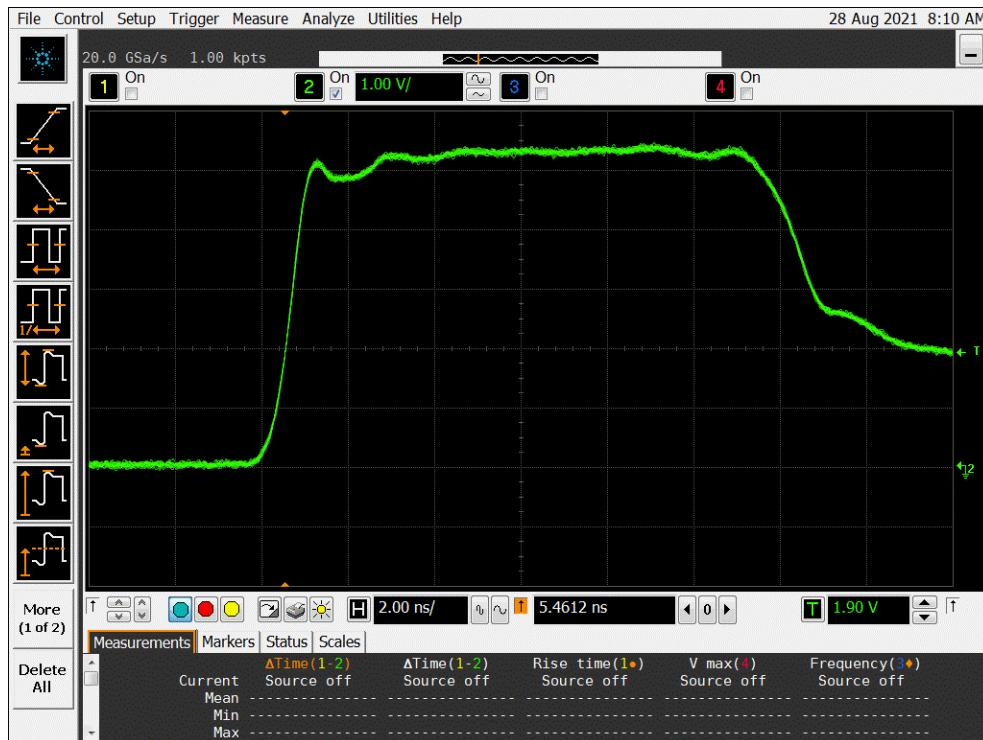
Figure 9b DUT 17070 Post-Annealing Rising Edge
