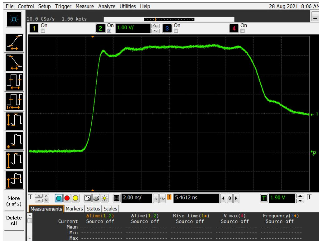
**Figure 11b DUT 17068 Post-Annealing Rising edge**
