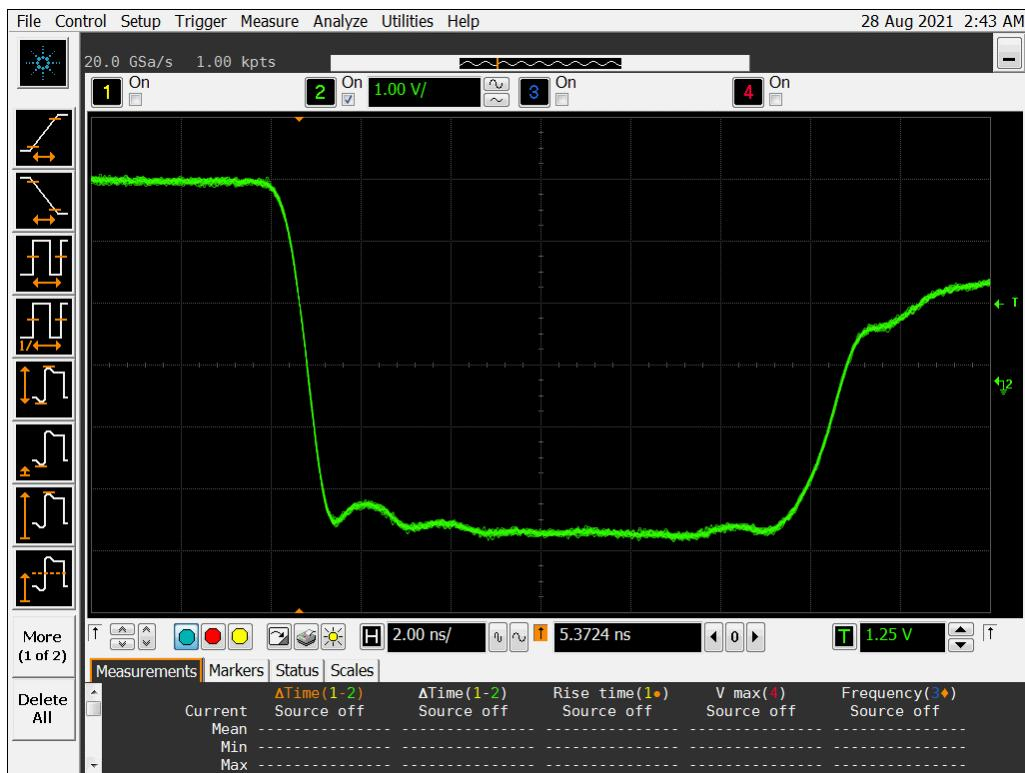
**Figure 20b DUT 4221 Post-Annealing Falling Edge**
