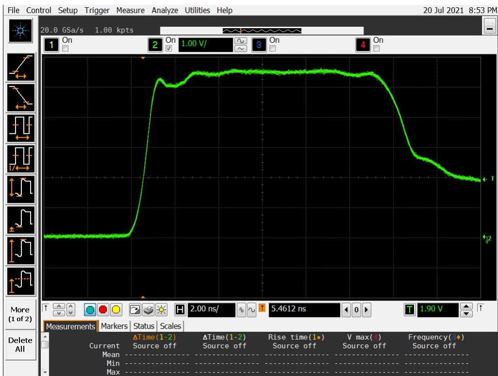
Figure 14a DUT 4221 Pre-Irradiation Rising Edge
