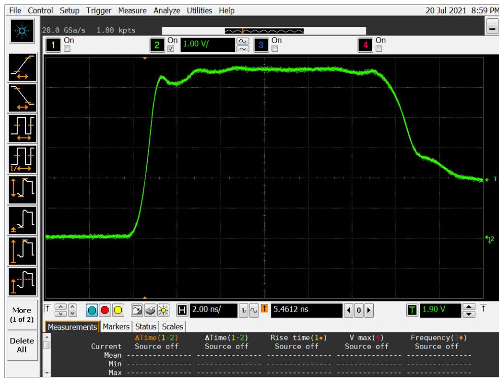
Figure 9a DUT 4252 Pre-Irradiation Rising Edge
