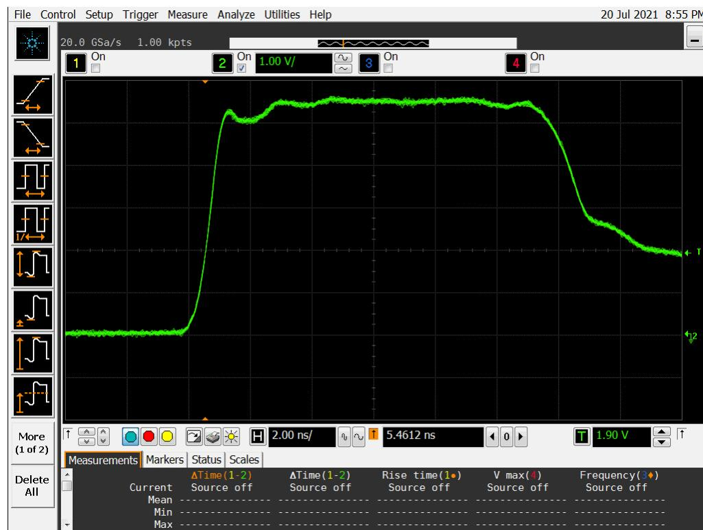
**Figure 11a DUT 4235 Pre-Radiation Rising Edge**
