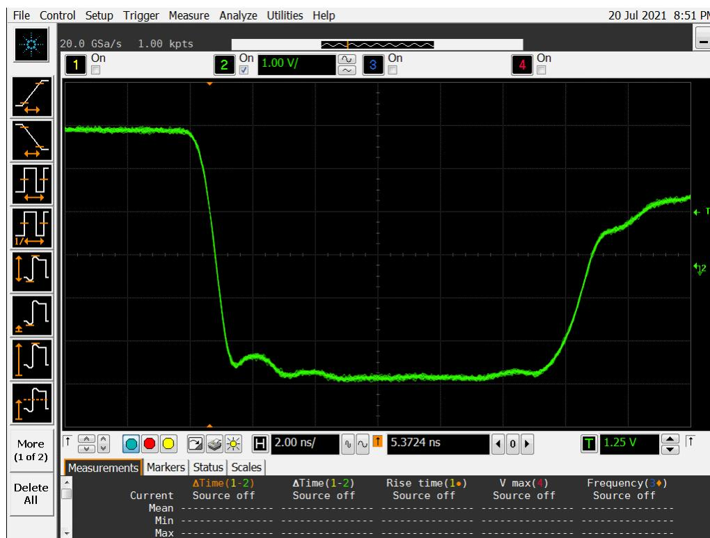
**Figure 19a DUT 4219 Pre-Irradiation Falling Edge**
