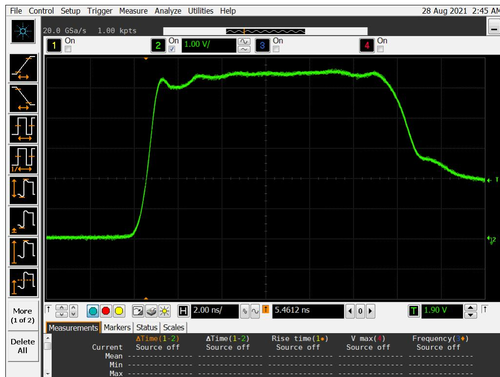
**Figure 11b DUT 4235 Post-Annealing Rising edge**
