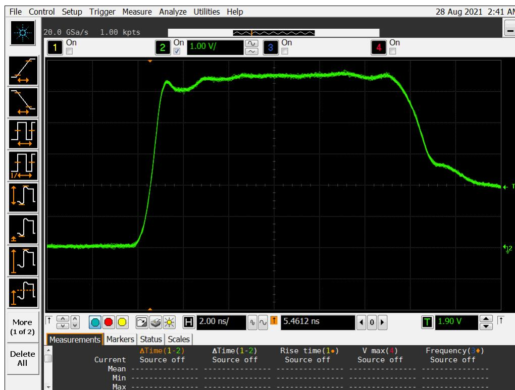
**Figure 13b DUT 4219 Post-Annealing Rising Edge**
