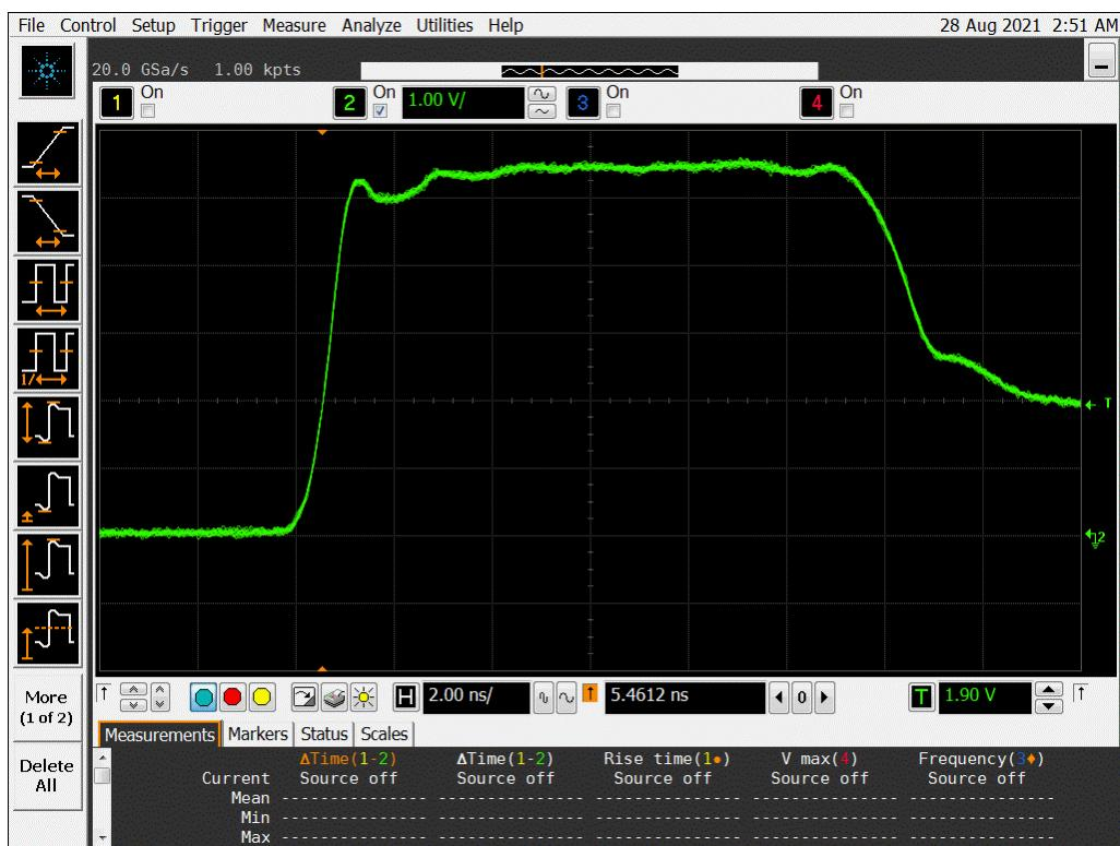
**Figure 10b DUT 4268 Post-Annealing Rising Edge**
