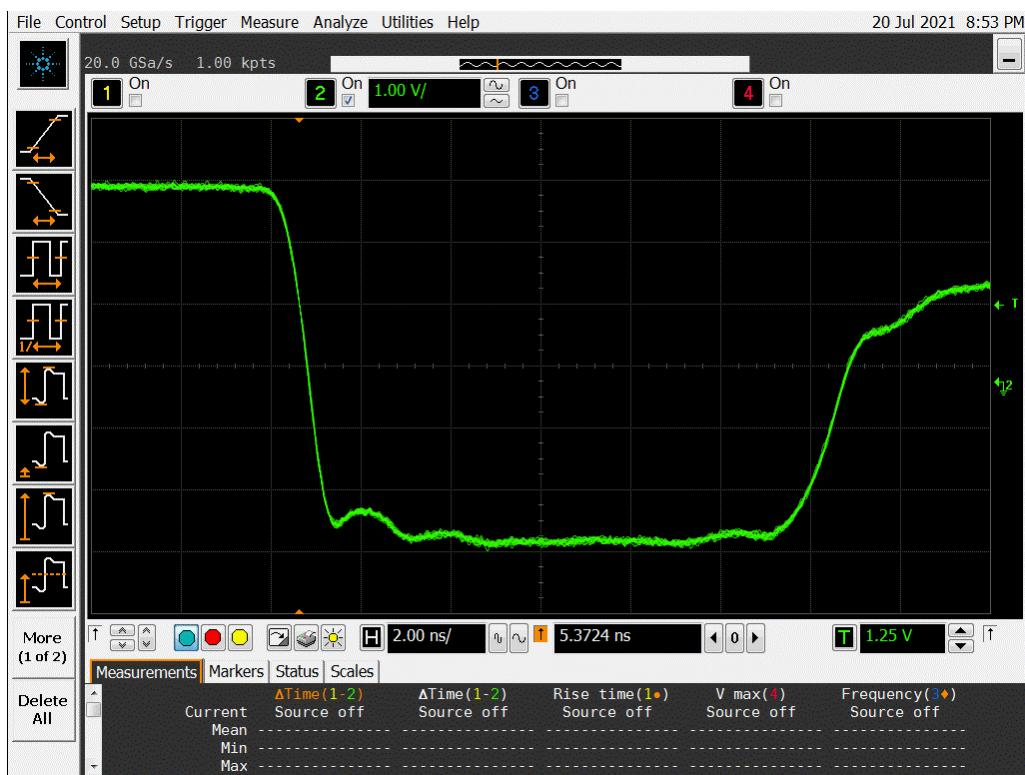
**Figure 20a DUT 4221 Pre-Irradiation Falling Edge**
