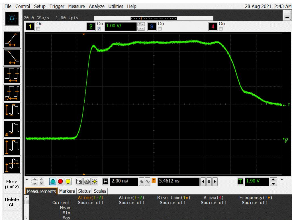
Figure 14b DUT 4221 Post-Annealing Rising Edge
