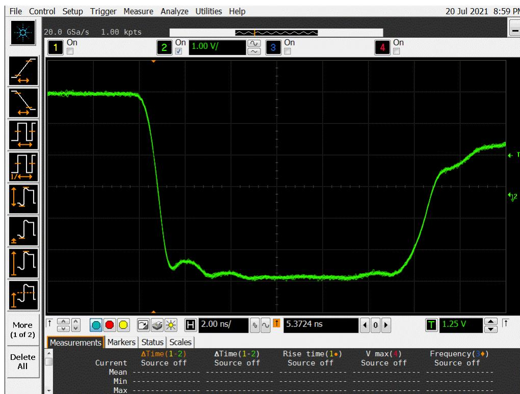
**Figure 15a DUT 4252 Pre-Radiation Falling Edge**
