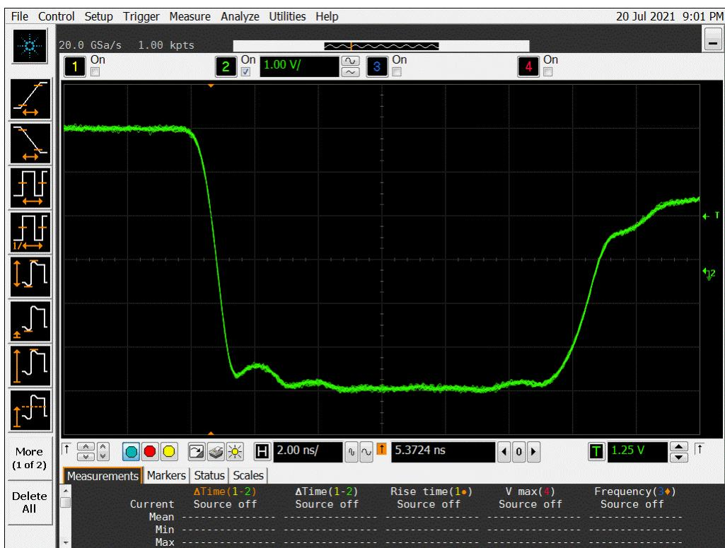
Figure 16a DUT 4268 Pre-Irradiation Falling Edge
