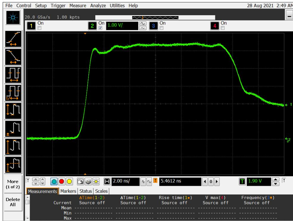
Figure 9b DUT 4252 Post-Annealing Rising Edge
