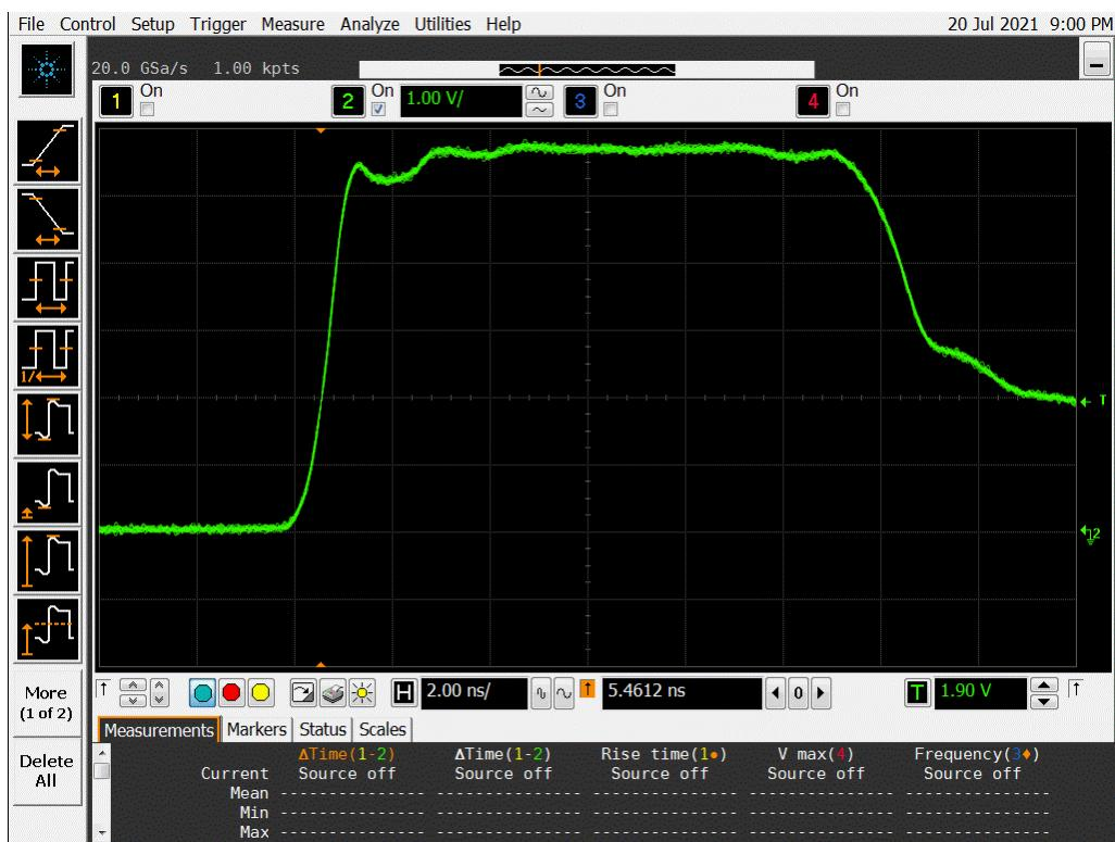
**Figure 10a DUT 4268 Pre-Irradiation Rising Edge**
