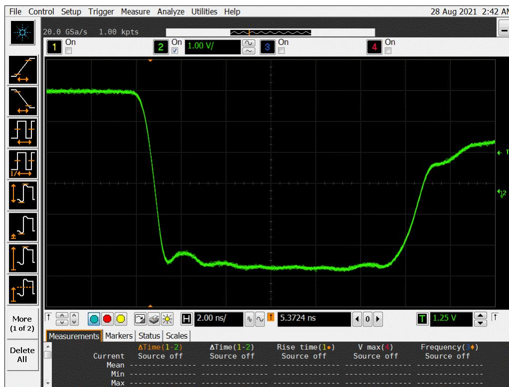
**Figure 19b DUT 4219 Post-Annealing Falling Edge**
