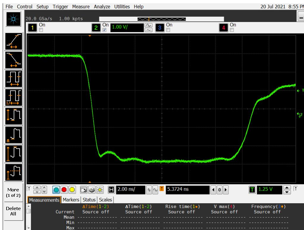
**Figure 17a DUT 4235 Pre-Irradiation Falling Edge**
