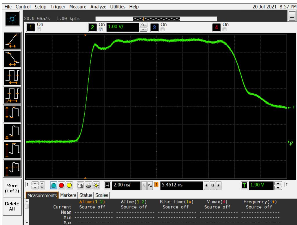
Figure 12a DUT 4251 Pre-Irradiation Rising Edge
