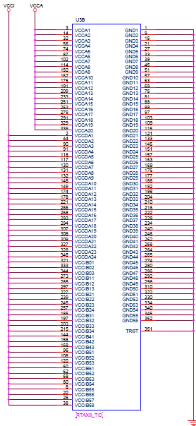
Figure A2 Power Supply, Ground and Special Pins Bias During Irradiation
