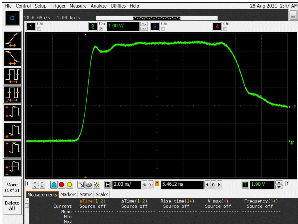
Figure 12b DUT 4251 Post-Annealing Rising Edge
