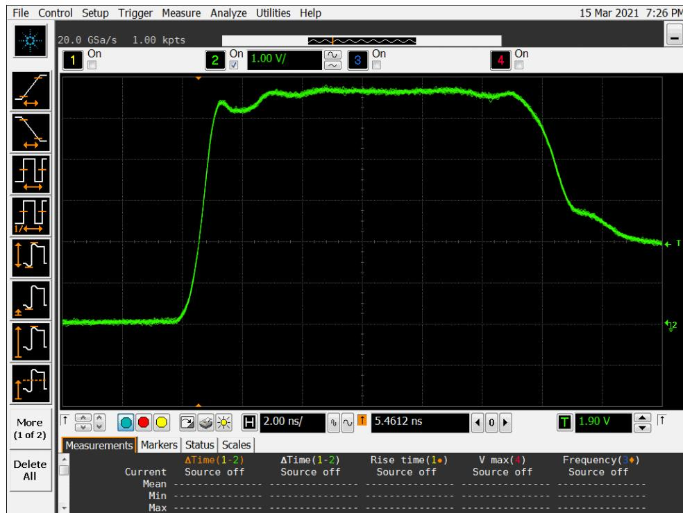
Figure 9b DUT 15412 Post-Annealing Rising Edge
