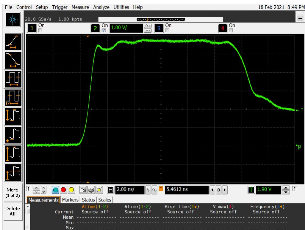
Figure 10a DUT 15415 Pre-Irradiation Rising Edge
