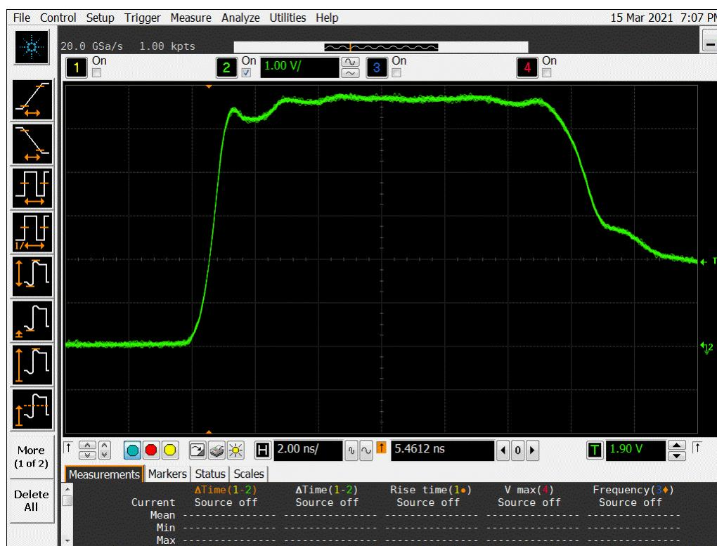
**Figure 13b DUT 15397 Post-Annealing Rising Edge**
