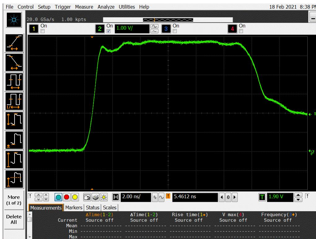
**Figure 13a DUT 15397 Pre-Irradiation Rising Edge**
