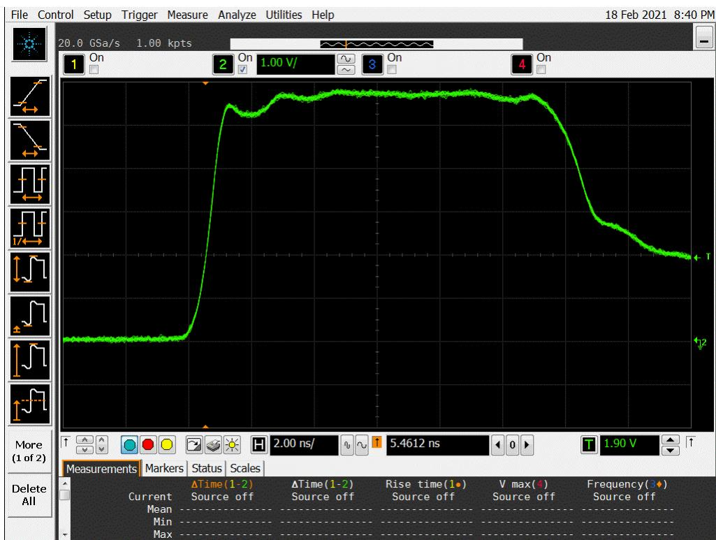
**Figure 14a DUT 15401 Pre-Irradiation Rising Edge**
