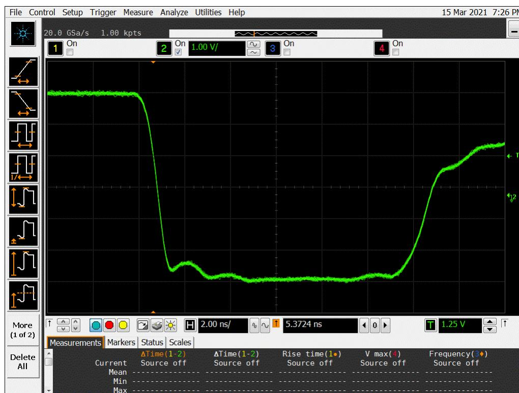
**Figure 15b DUT 15412 Post-Annealing Falling Edge**
