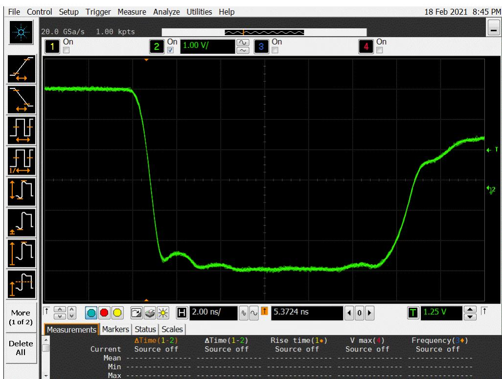
Figure 18a DUT 15411 Pre-Irradiation Falling Edge
