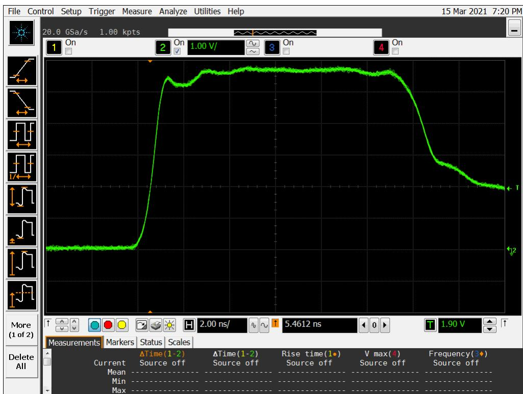
**Figure 14b DUT 15401 Post-Annealing Rising Edge**
