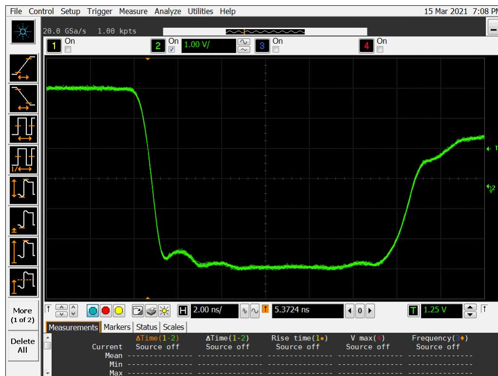
**Figure 19b DUT 15397 Post-Annealing Falling Edge**
