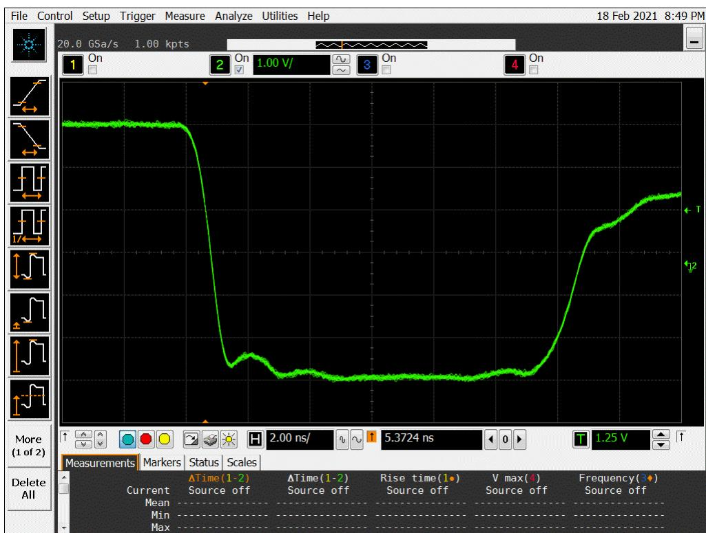
**Figure 16a DUT 15415 Pre-Irradiation Falling Edge**
