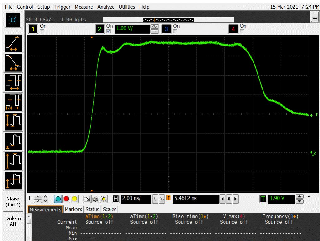
Figure 12b DUT 15411 Post-Annealing Rising Edge
