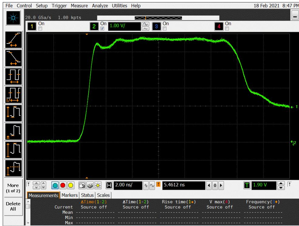
Figure 9a DUT 15412 Pre-Irradiation Rising Edge
