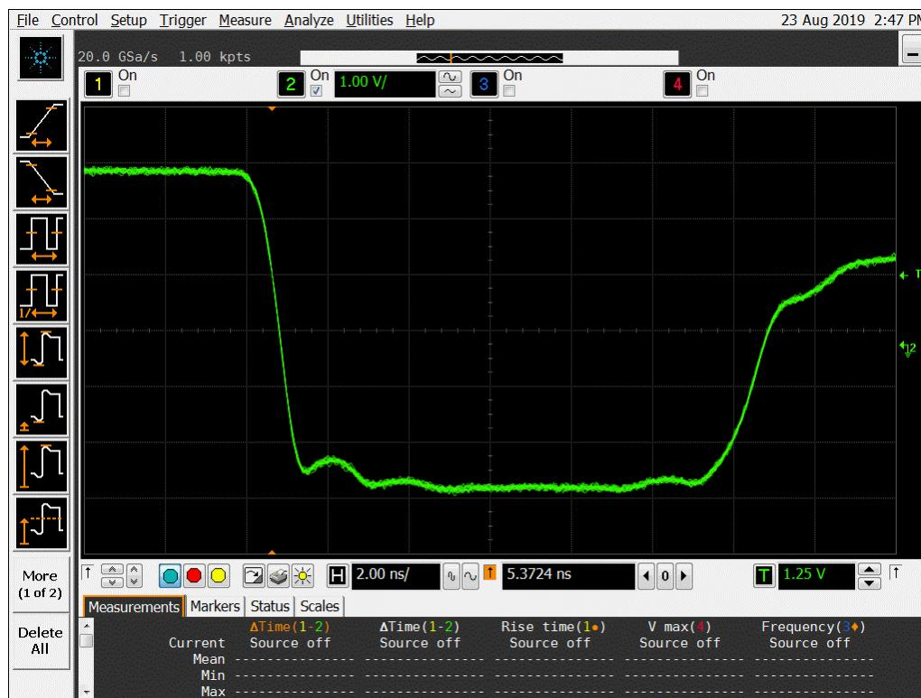
**Figure 15b DUT 5444 Post-Annealing Falling Edge**
