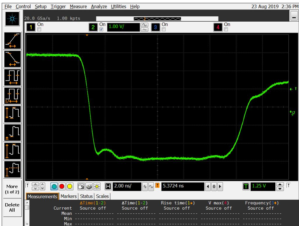
**Figure 16b DUT 5447 Post-Annealing Falling Edge**
