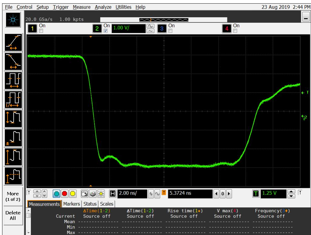
**Figure 20b DUT 5405 Post-Annealing Falling Edge**
