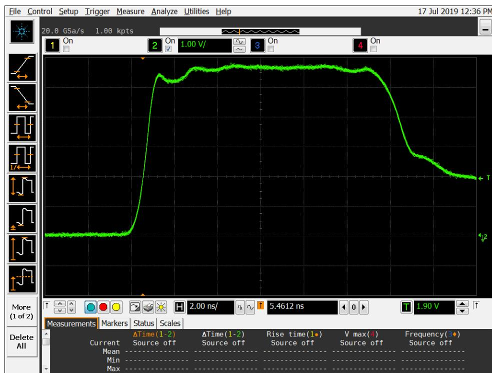
Figure 9a DUT 5444 Pre-Irradiation Rising Edge
