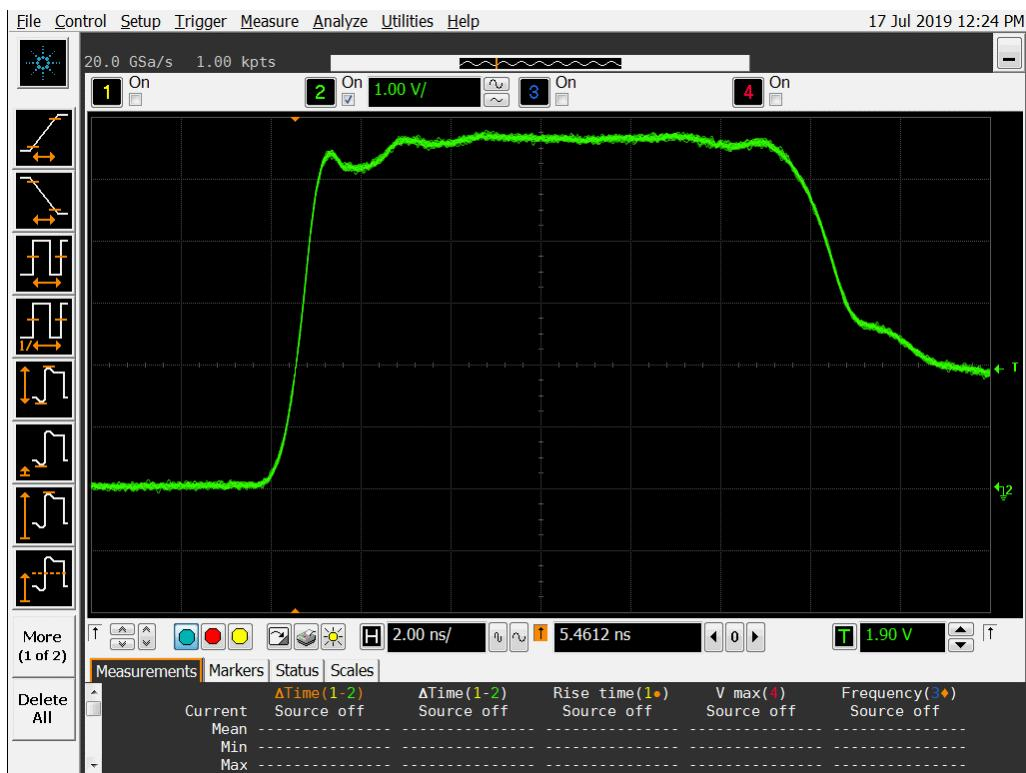
**Figure 14a DUT 5405 Pre-Irradiation Rising Edge**
