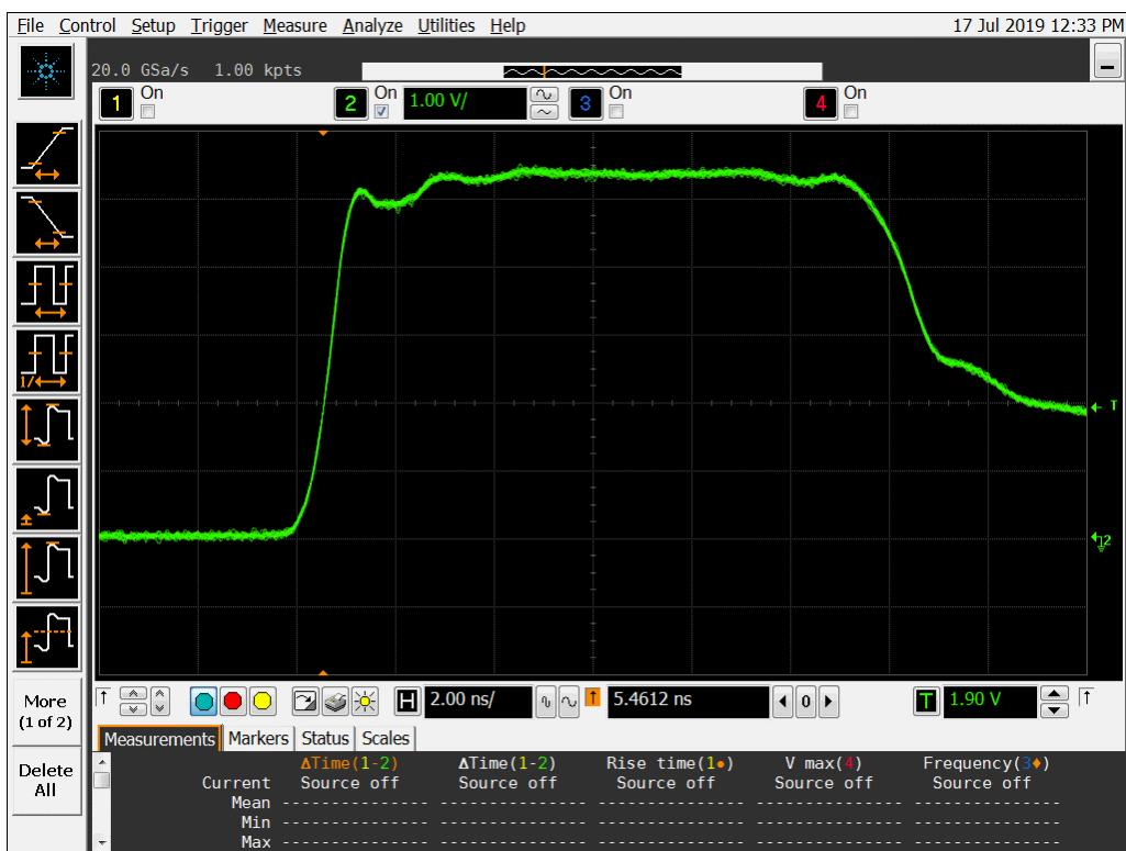
**Figure 12a DUT 5420 Pre-Irradiation Rising Edge**
