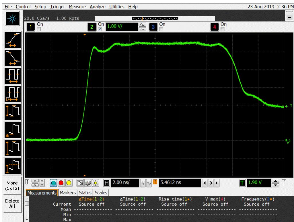
**Figure 10b DUT 5447 Post-Annealing Rising Edge**
