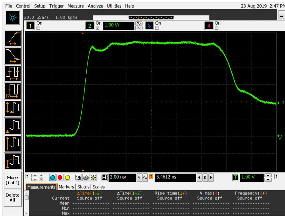
Figure 9b DUT 5444 Post-Annealing Rising Edge
