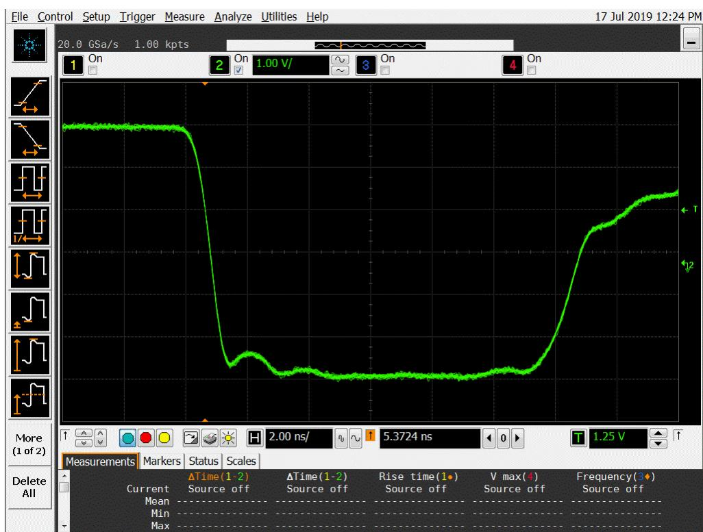
**Figure 20a DUT 5405 Pre-Irradiation Falling Edge**
