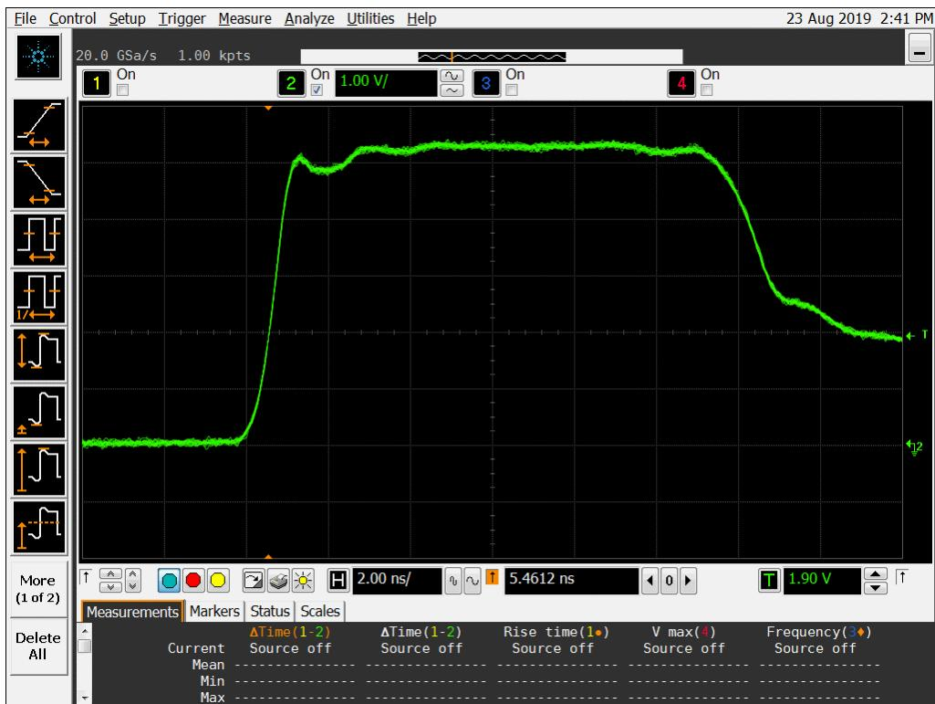
**Figure 12b DUT 5420 Post-Annealing Rising Edge**
