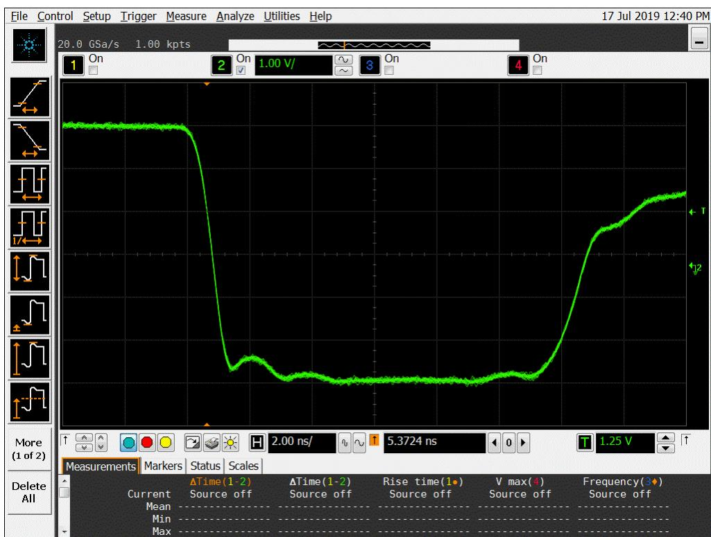
**Figure 16a DUT 5447 Pre-Irradiation Falling Edge**
