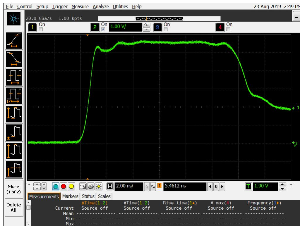
**Figure 11b DUT 5410 Post-Annealing Rising edge**
