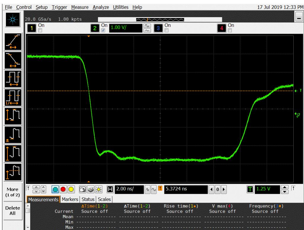
**Figure 18a DUT 5420 Pre-Irradiation Falling Edge**
