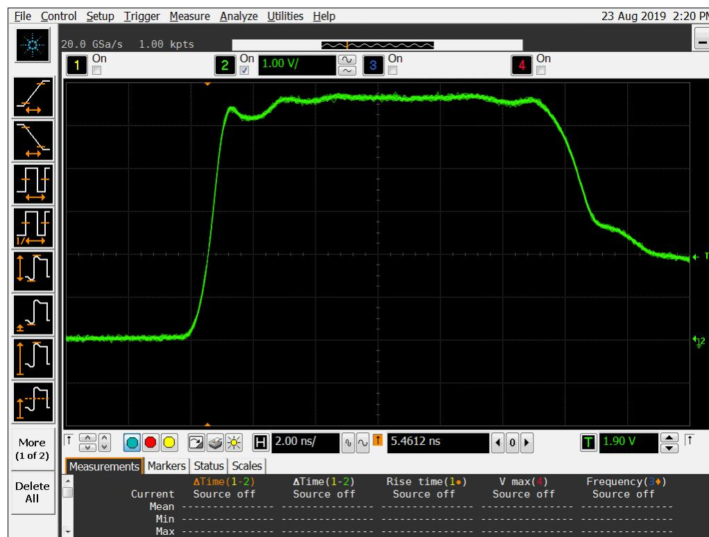
**Figure 13b DUT 5400 Post-Annealing Rising Edge**
