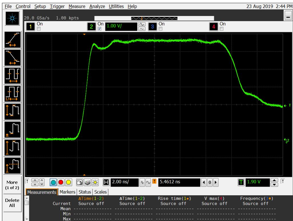
**Figure 14b DUT 5405 Post-Annealing Rising Edge**
