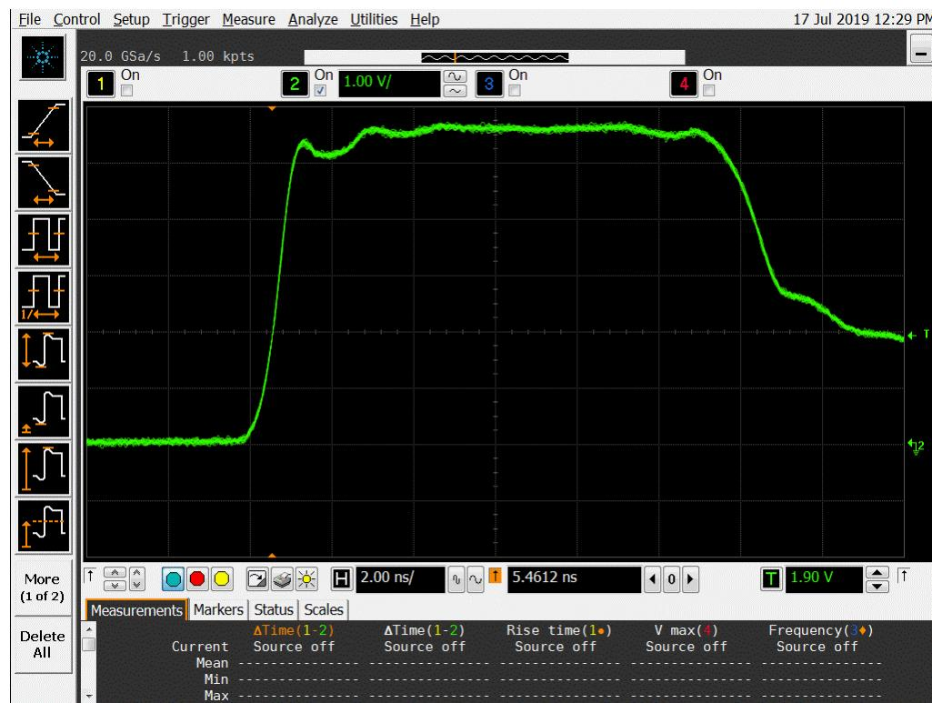
**Figure 11a DUT 5410 Pre-Radiation Rising Edge**
