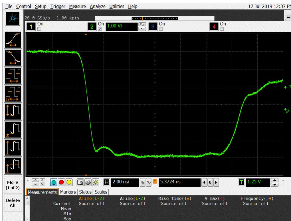
**Figure 15a DUT 5444 Pre-Radiation Falling Edge**
