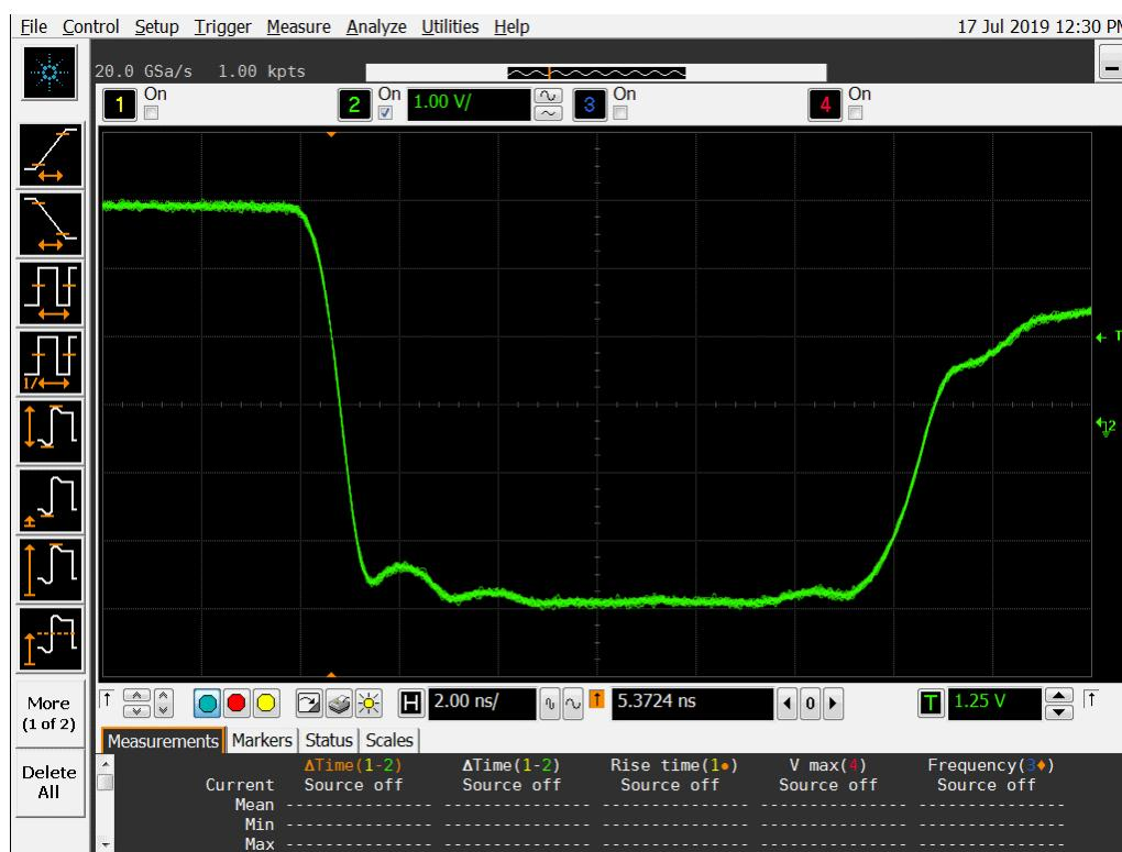
**Figure 17a DUT 5410 Pre-Irradiation Falling Edge**
