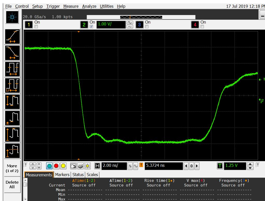
**Figure 19a DUT 5400 Pre-Irradiation Falling Edge**
