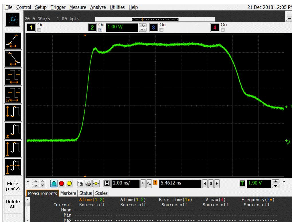
**Figure 13b DUT 8676 Post-Annealing Rising Edge**
