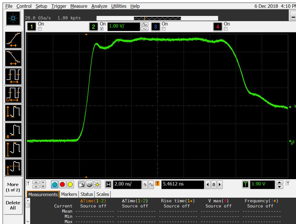
**Figure 11a DUT 8680 Pre-Radiation Rising Edge**
