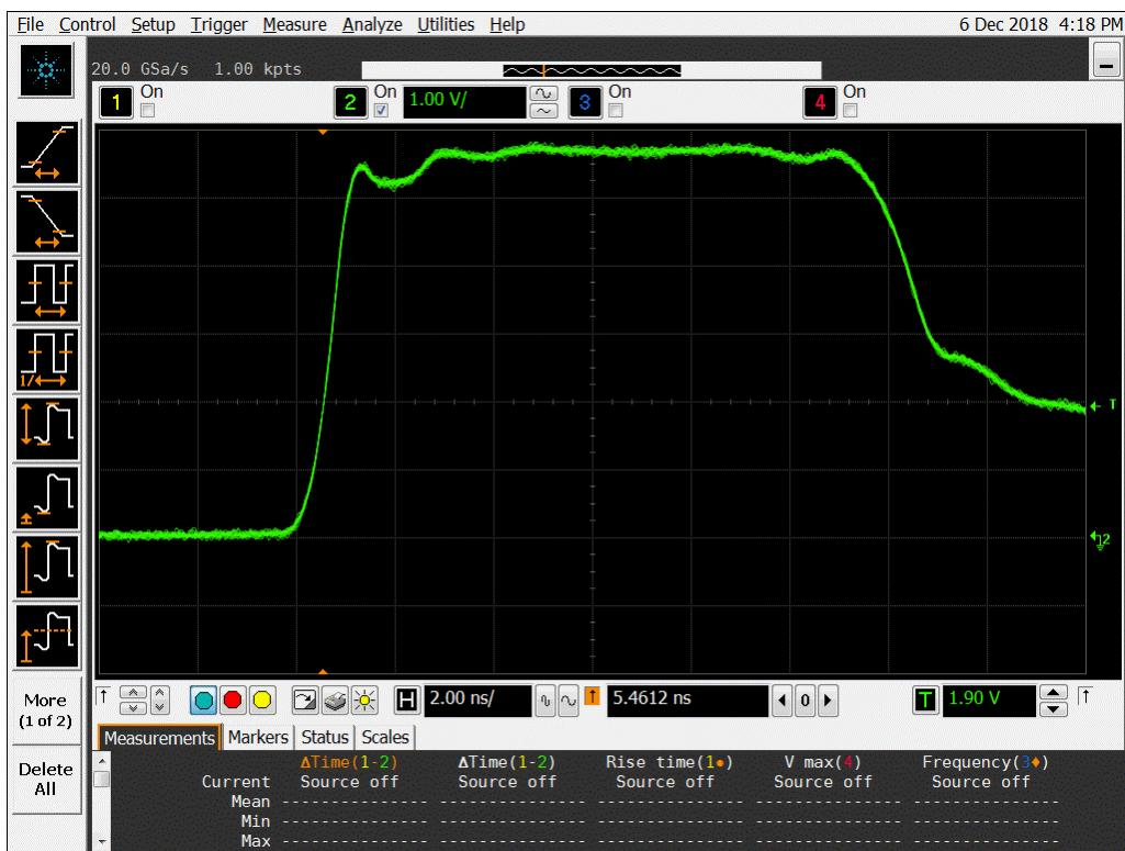
**Figure 10a DUT 8686 Pre-Irradiation Rising Edge**
