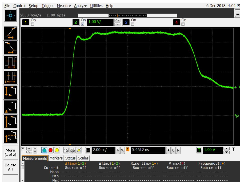
**Figure 13a DUT 8676 Pre-Irradiation Rising Edge**
