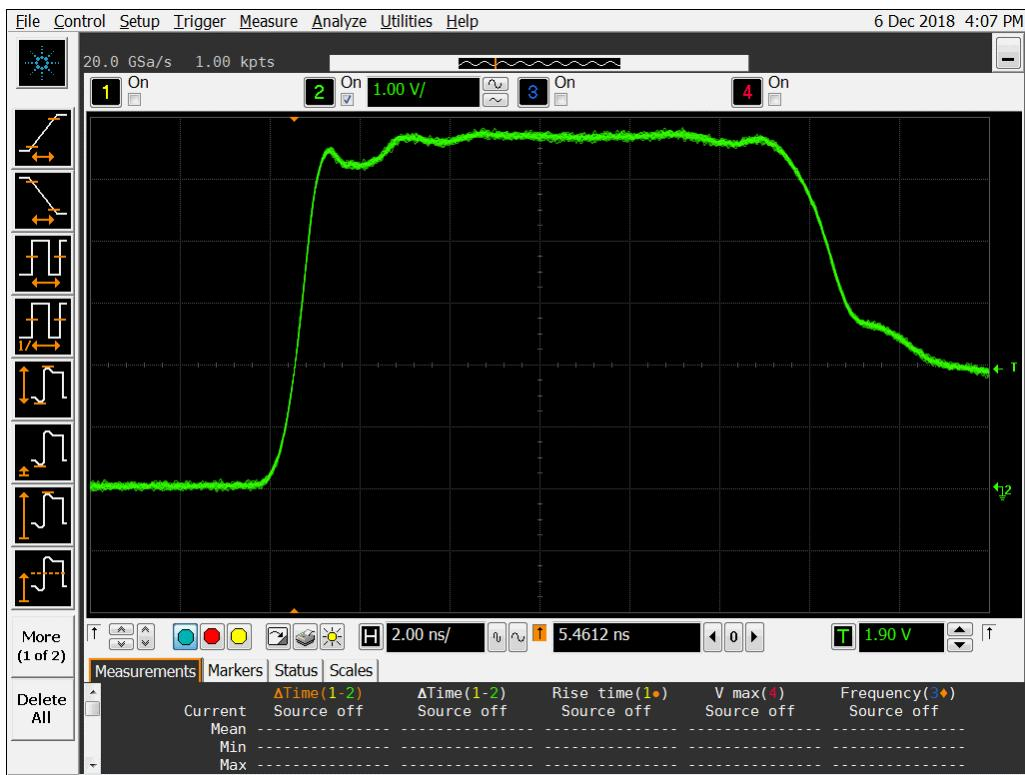
Figure 14a DUT 8679 Pre-Irradiation Rising Edge
