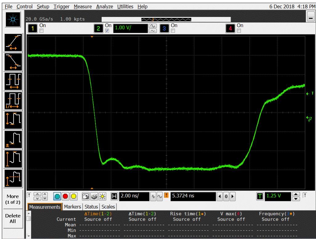
Figure 16a DUT 8686 Pre-Irradiation Falling Edge
