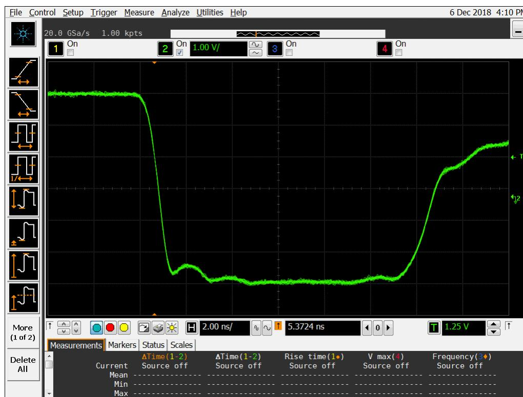
**Figure 17a DUT 8680 Pre-Irradiation Falling Edge**
