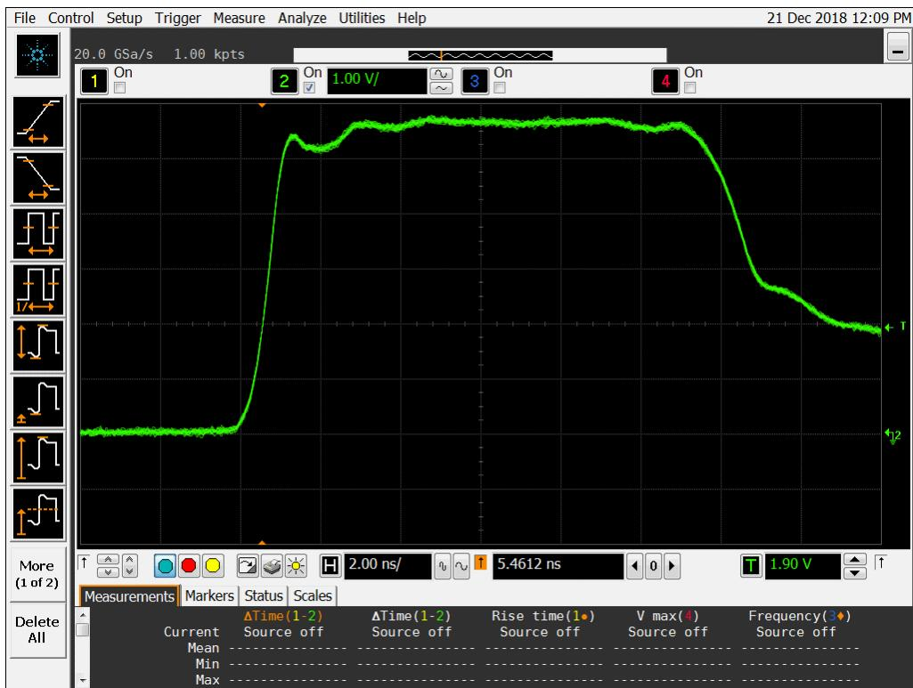
Figure 14b DUT 8679 Post-Annealing Rising Edge
