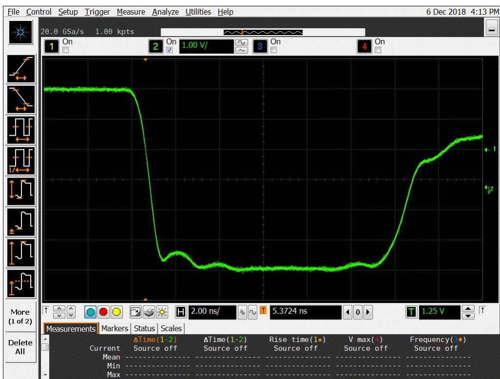
**Figure 18a DUT 8682 Pre-Irradiation Falling Edge**
