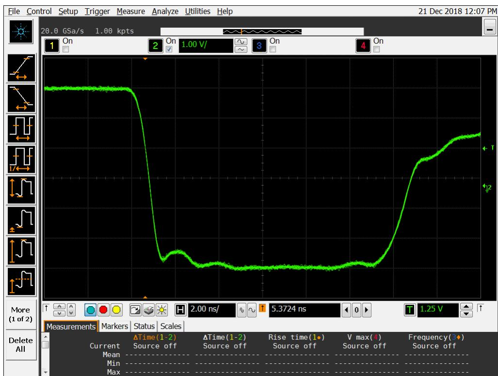
**Figure 20b DUT 8679 Post-Annealing Falling Edge**
