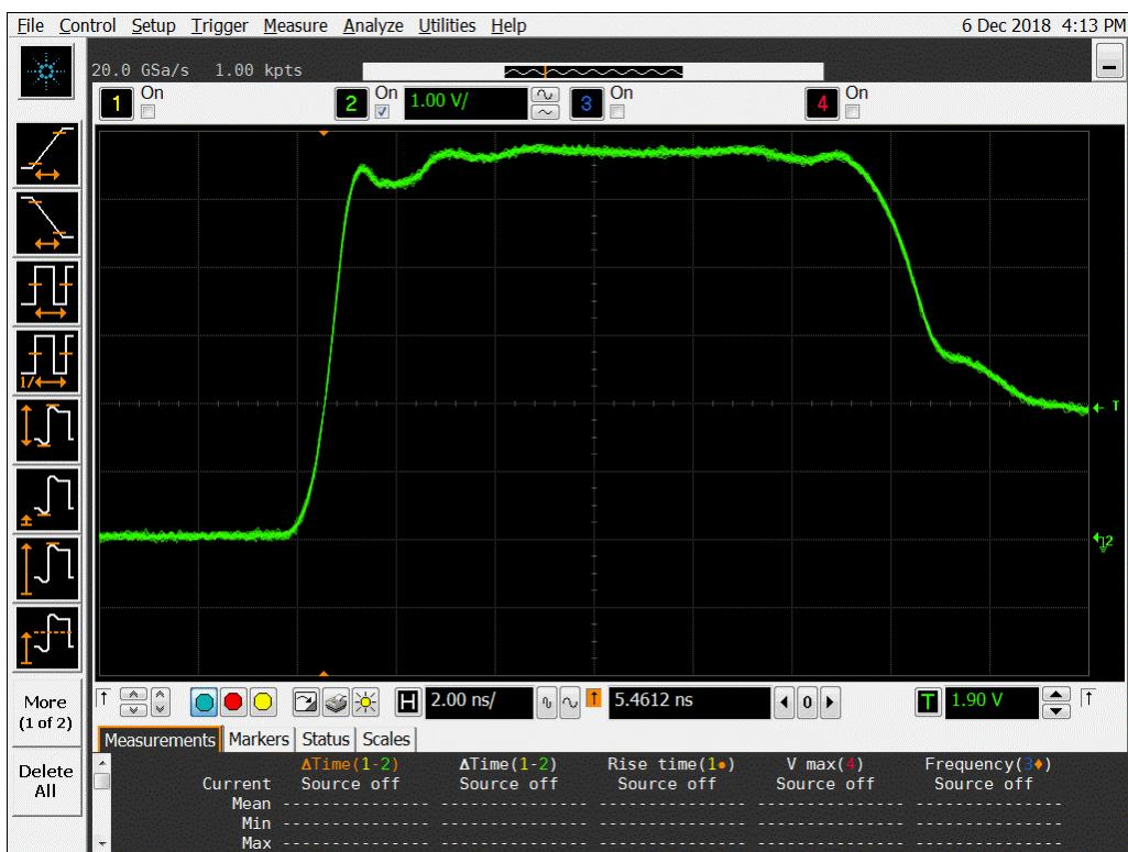
Figure 12a DUT 8682 Pre-Irradiation Rising Edge
