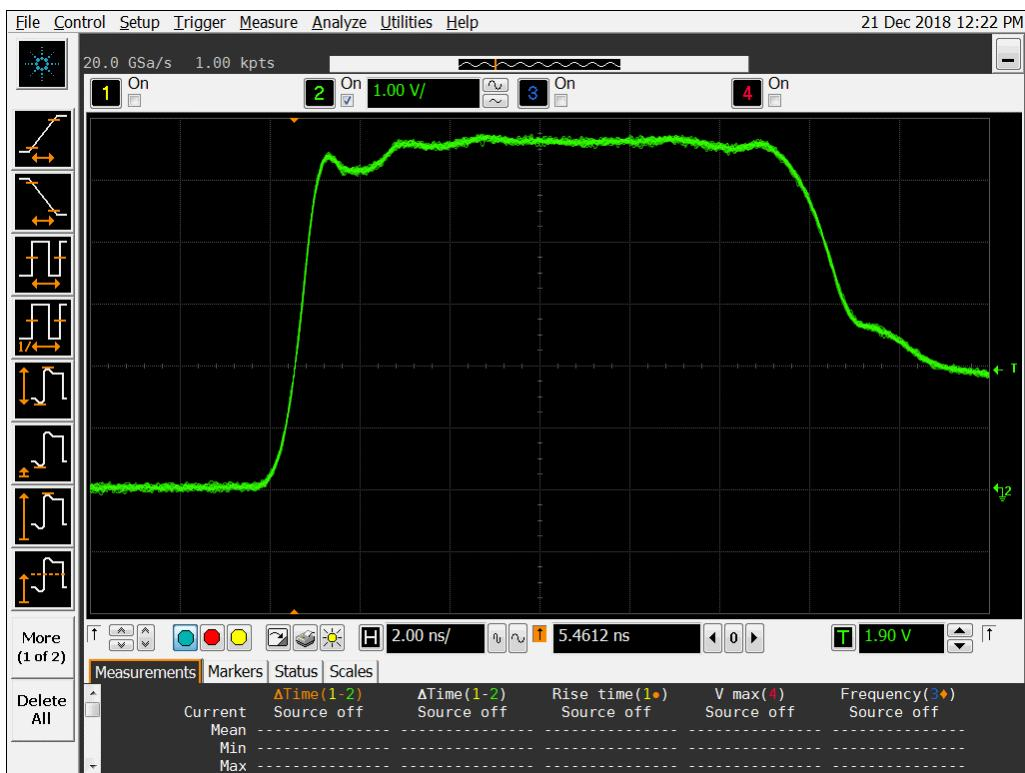
Figure 12b DUT 8682 Post-Annealing Rising Edge
