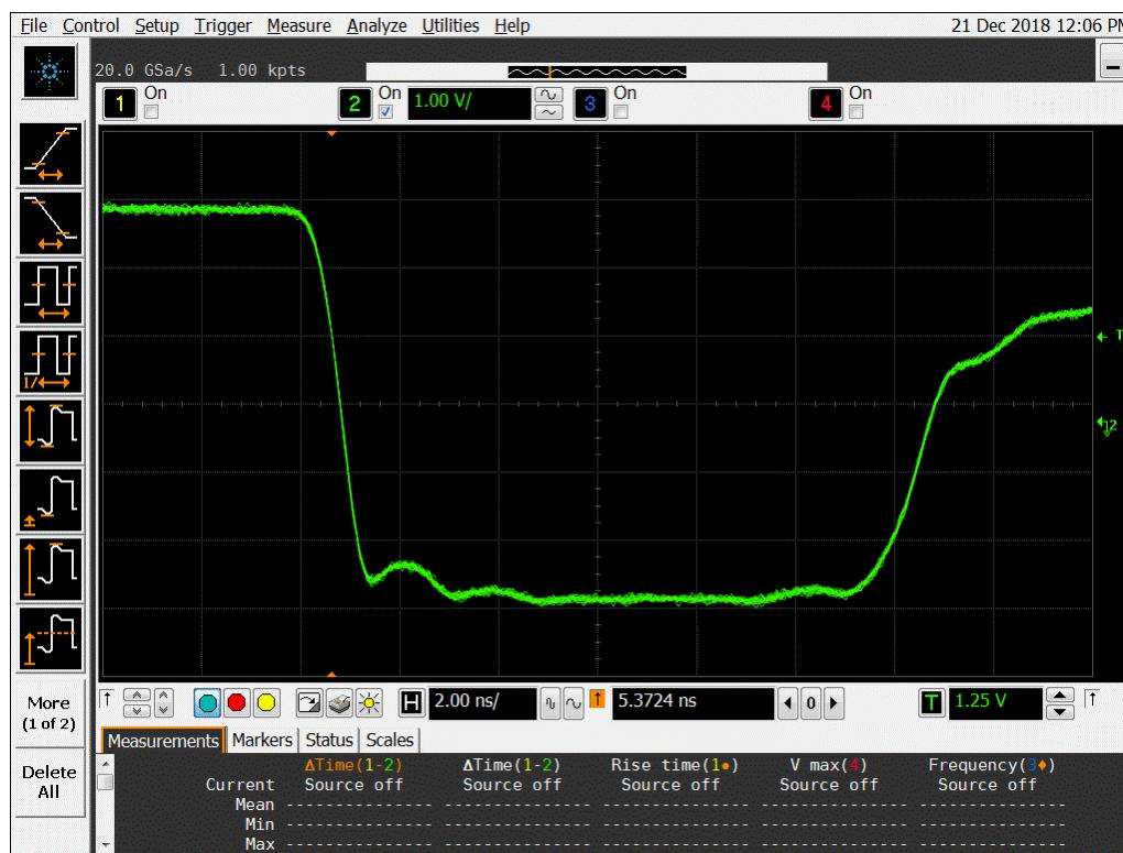
**Figure 19b DUT 8676 Post-Annealing Falling Edge**
