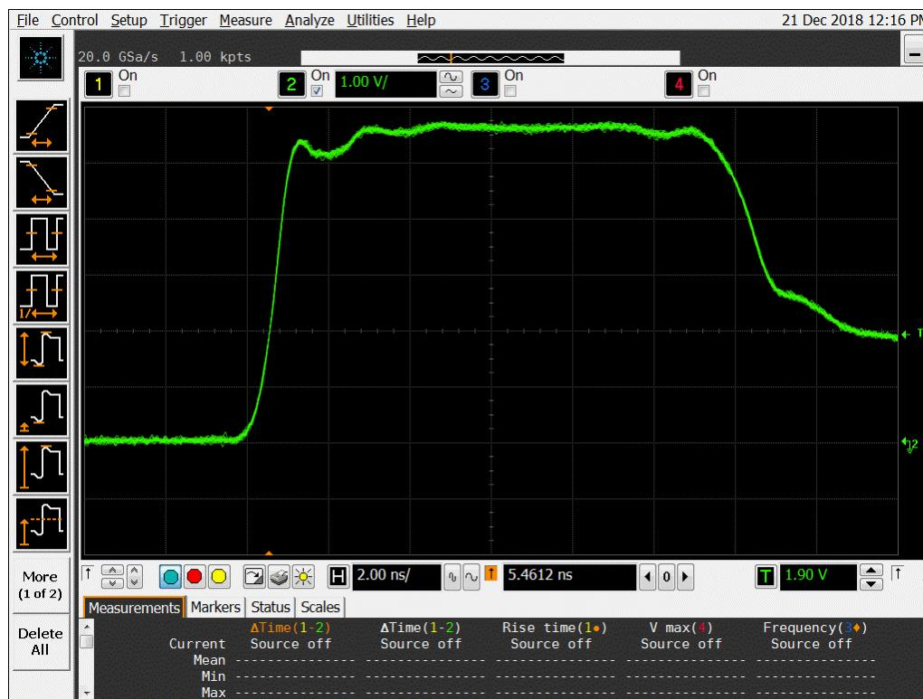
**Figure 11b DUT 8680 Post-Annealing Rising edge**
