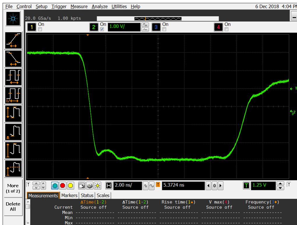
**Figure 19a DUT 8676 Pre-Irradiation Falling Edge**
