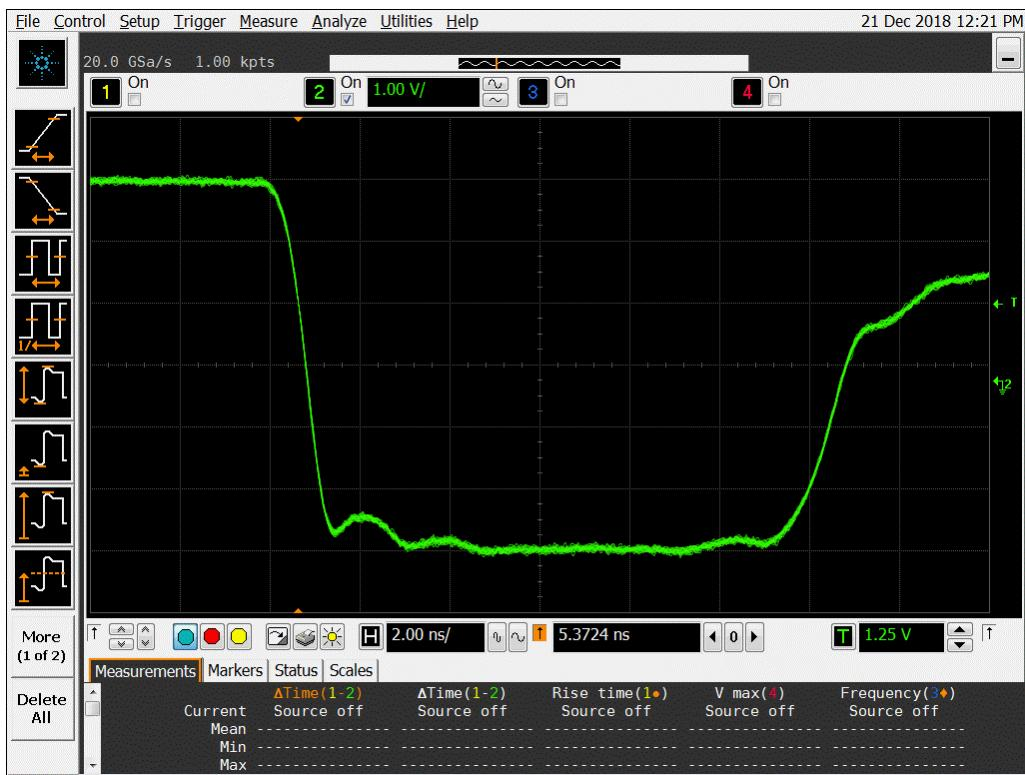
**Figure 18b DUT 8682 Post-Annealing Falling Edge**
