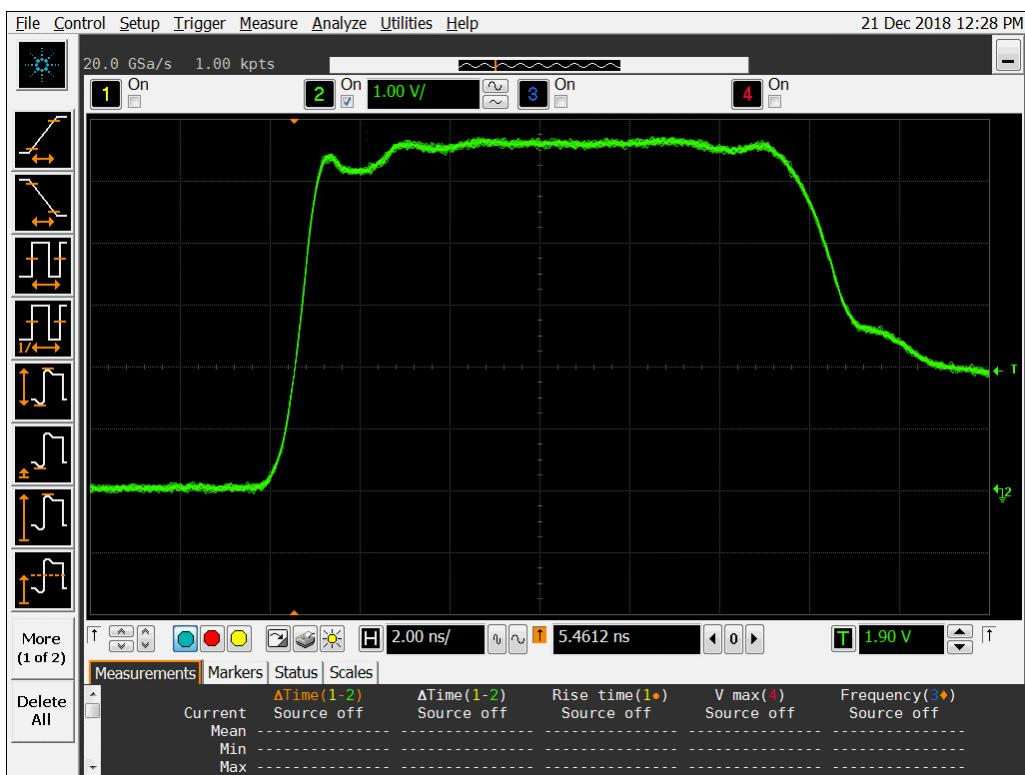
**Figure 10b DUT 8686 Post-Annealing Rising Edge**
