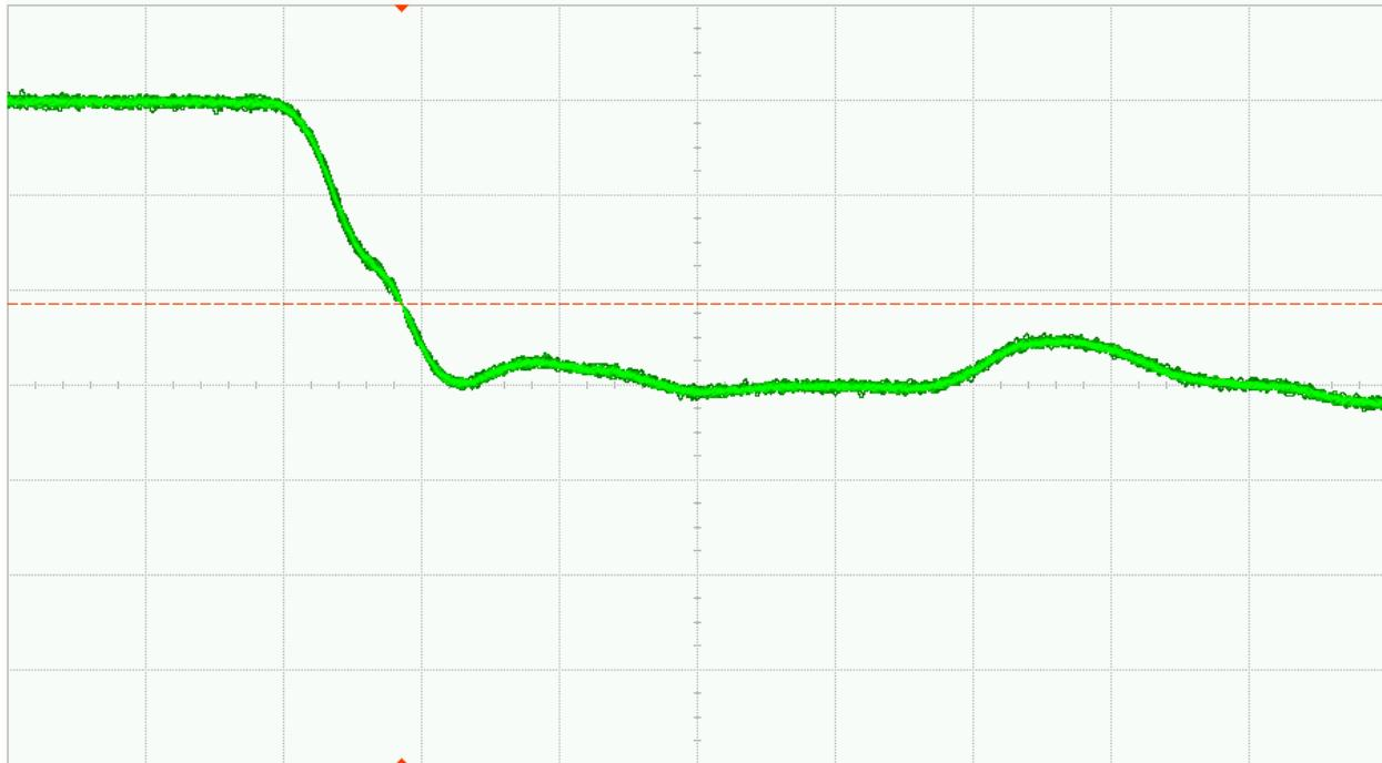
Fig. 32 (a). DUT 9782 pre-irradiation falling edge, abscissa scale is 1V/div and ordinate scale is 2ns/div
