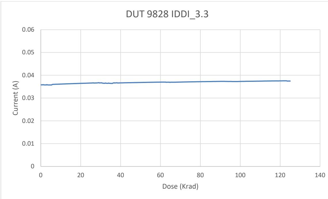
Fig. 19. DUT 9828 I/O bank 3.3V power supply current ( $I_{DDI\_3.3}$ ) versus TID
