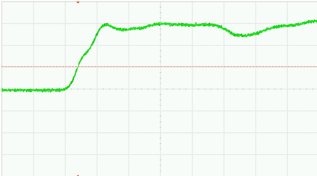
Fig. 29 (a). DUT 9823 pre-irradiation rising edge, abscissa scale is 1V/div and ordinate scale is 2ns/div
