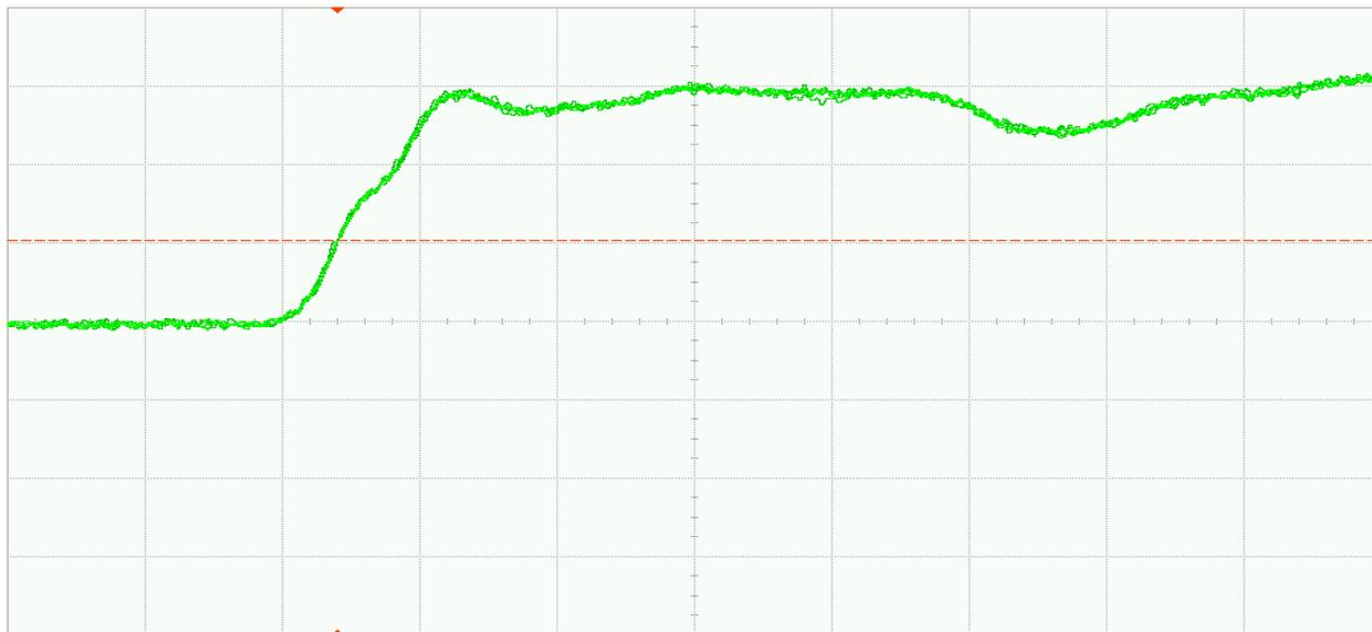
Fig. 26 (b). DUT 9782 post-annealing rising edge, abscissa scale is 1V/div and ordinate scale is 2ns/div
