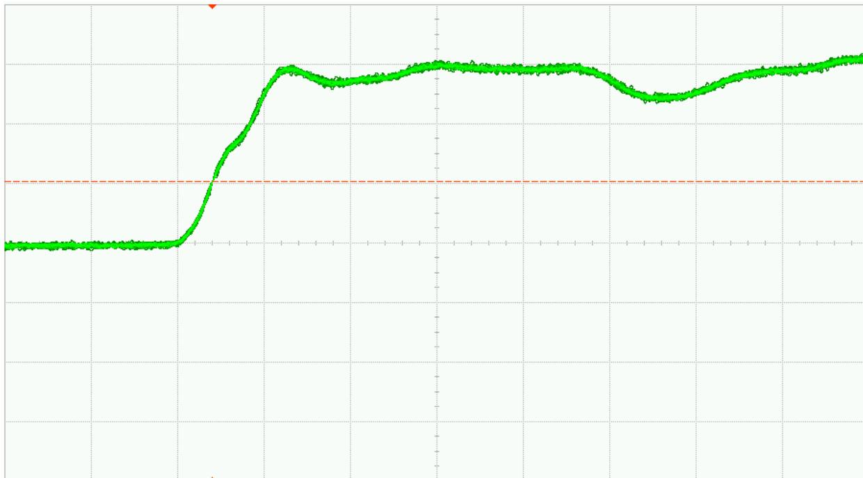
Fig. 29 (b). DUT 9823 post-annealing rising edge, abscissa scale is 1V/div and ordinate scale is 2ns/div
