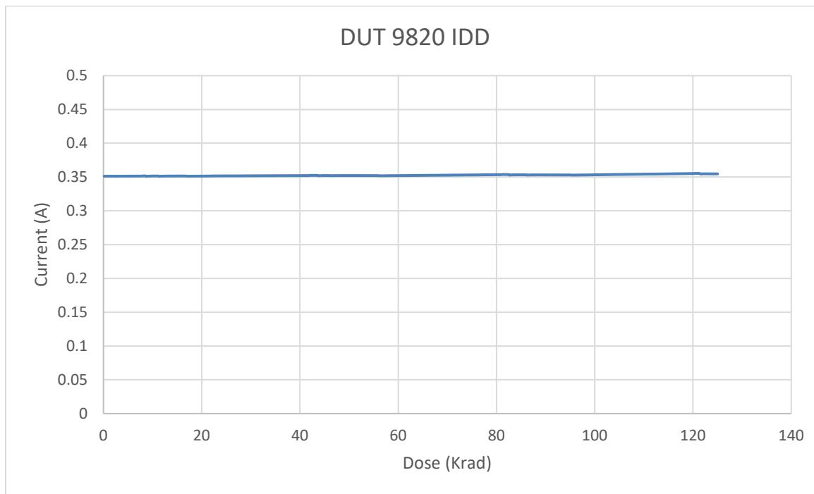
Fig. 4. DUT 9820 core power supply current ( $I_{DD}$ ) versus TID
