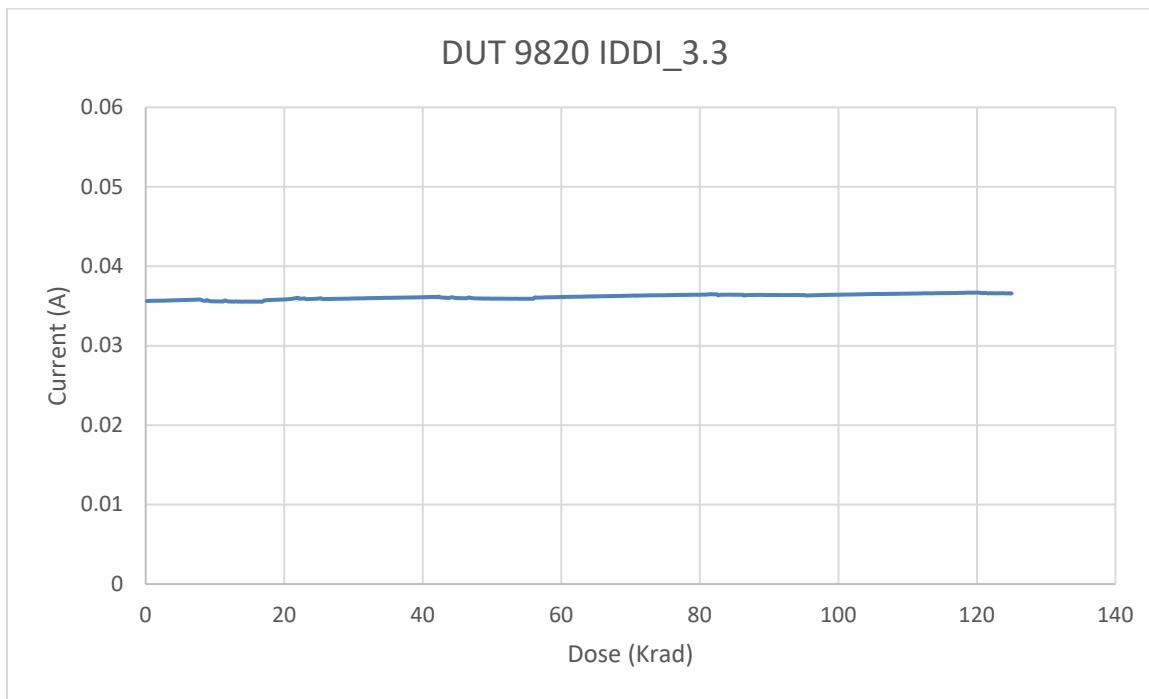
Fig. 16. DUT 9820 I/O bank 3.3V power supply current ( $I_{DDI\_3.3}$ ) versus TID
