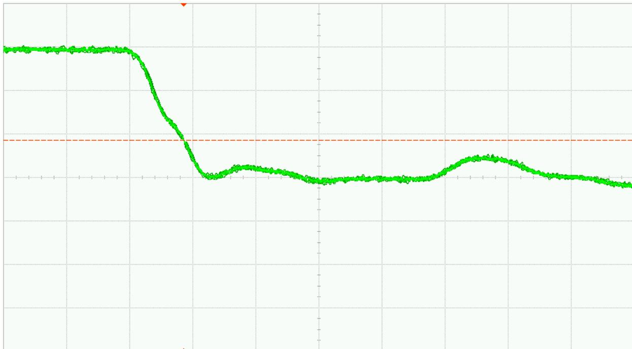
Fig. 36 (b). DUT 9826 post-annealing falling edge, abscissa scale is 1V/div and ordinate scale is 2ns/div
