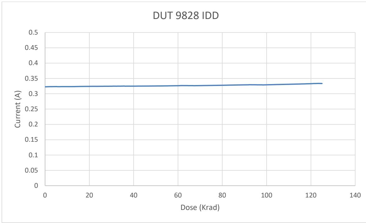
Fig. 7. DUT 9828 core power supply current ( $I_{DD}$ ) versus TID
