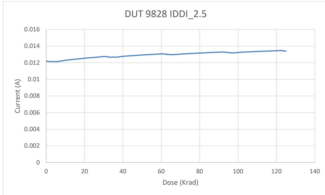
Fig. 13. DUT 9828 I/O bank 2.5V power supply current ( $I_{DDI\_2.5}$ ) versus TID
