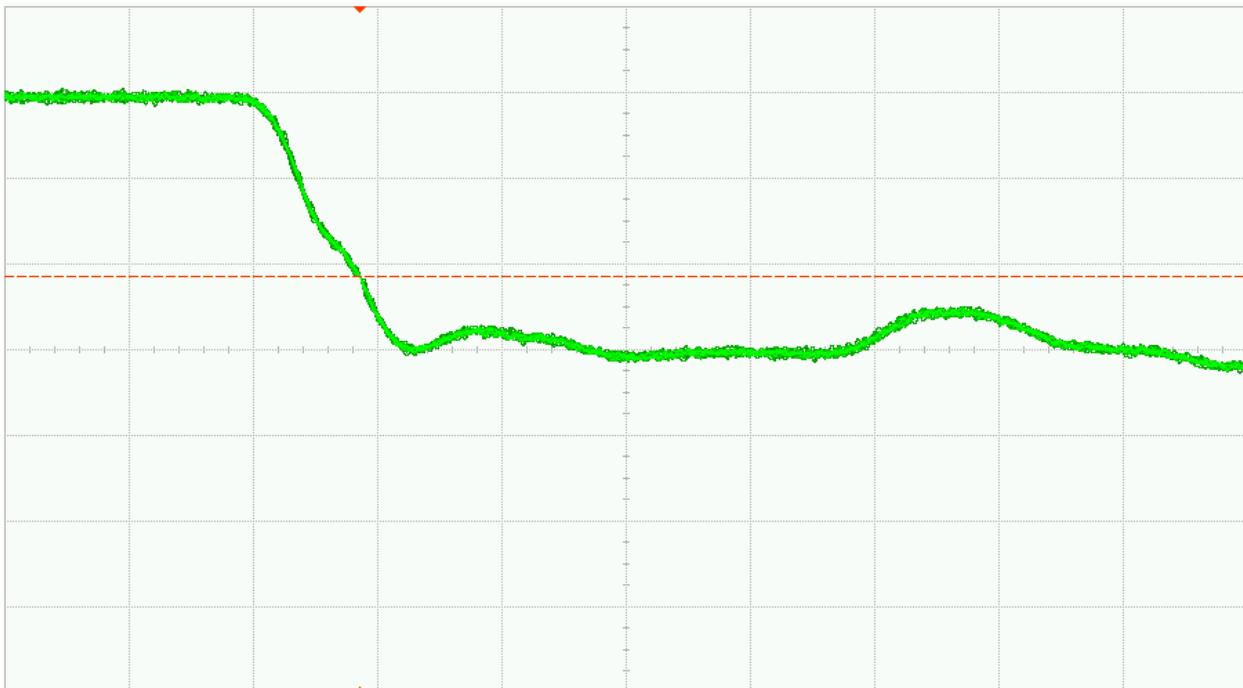
Fig. 37 (b). DUT 9828 post-annealing falling edge, abscissa scale is 1V/div and ordinate scale is 2ns/div
