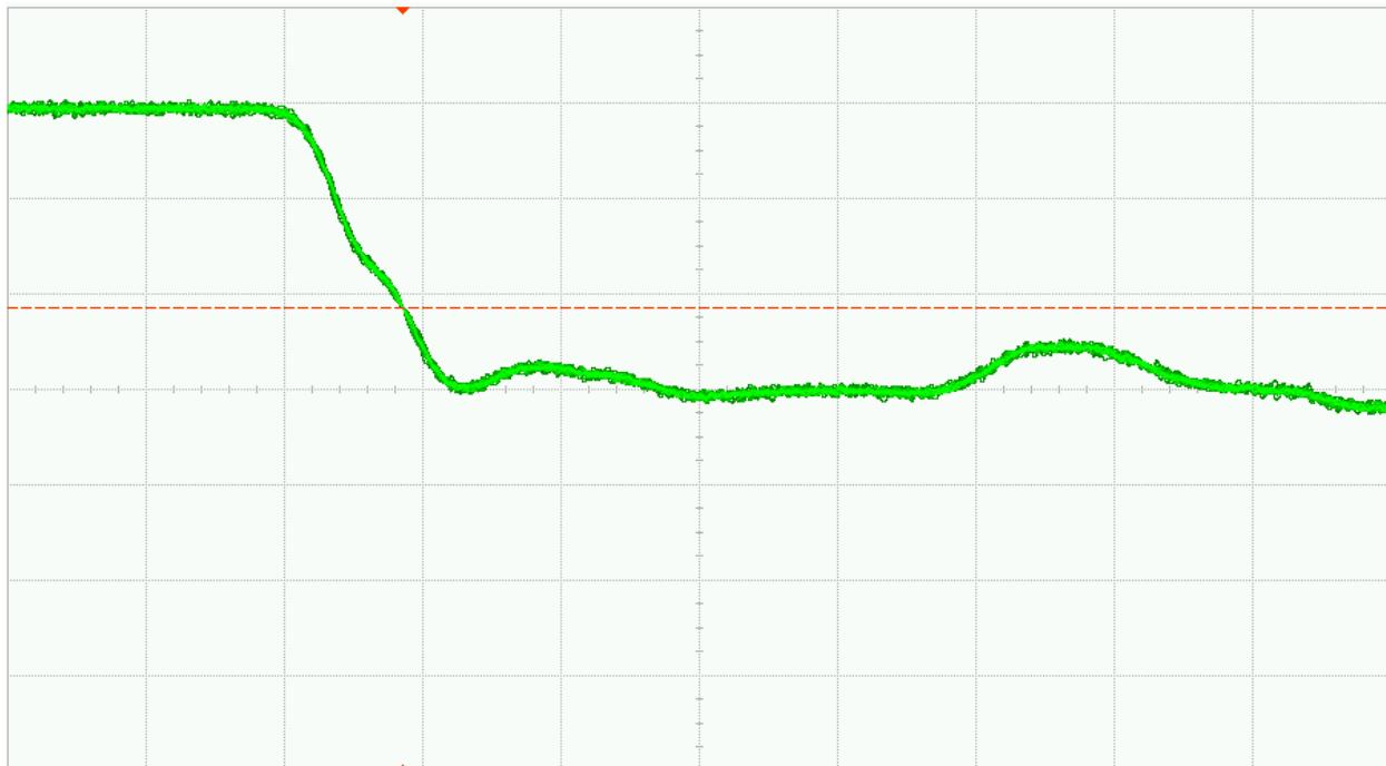
Fig. 35 (b). DUT 9823 post-annealing falling edge, abscissa scale is 1V/div and ordinate scale is 2ns/div
