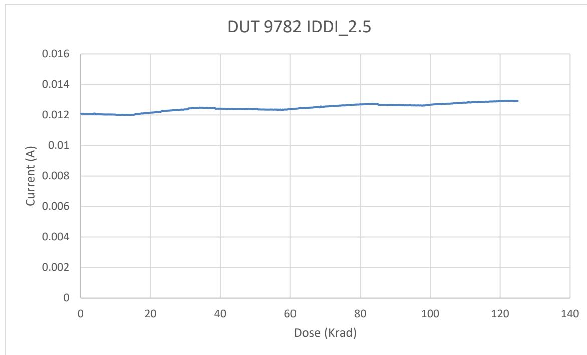
Fig. 8. DUT 9782 I/O bank 2.5V power supply current ( $I_{DDI\_2.5}$ ) versus TID
