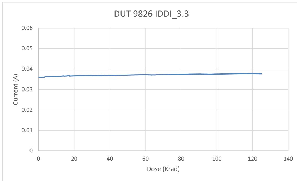
Fig. 18. DUT 9826 I/O bank 3.3V power supply current ( $I_{DDI\_3.3}$ ) versus TID
