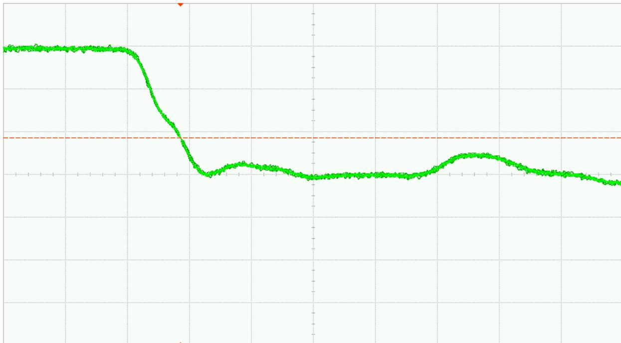
Fig. 32 (b). DUT 9782 post-annealing falling edge, abscissa scale is 1V/div and ordinate scale is 2ns/div
