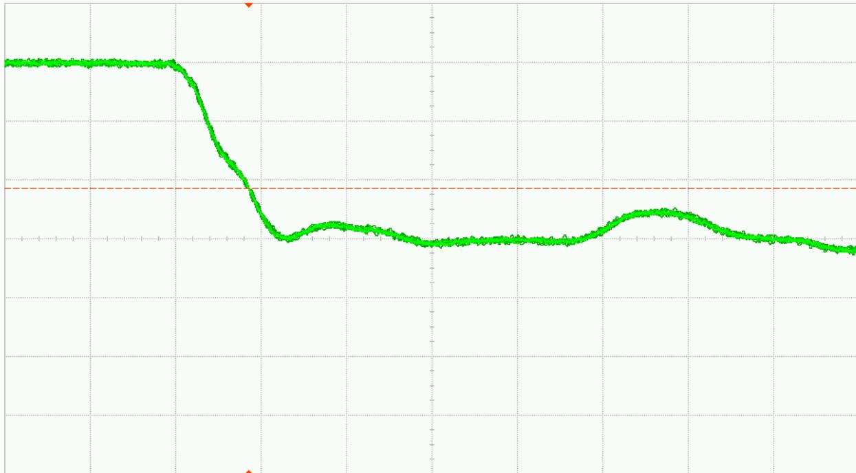
Fig. 36 (a). DUT 9826 pre-irradiation falling edge, abscissa scale is 1V/div and ordinate scale is 2ns/div
