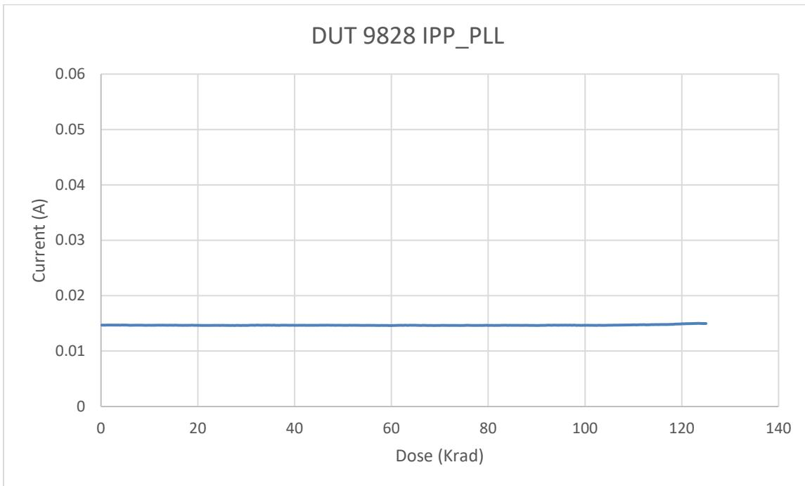
Fig. 25. DUT 9828 charge pump and PLL power supply current ( $I_{PP\_PLL}$ ) versus TID
