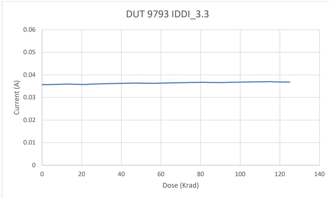
Fig. 15. DUT 9793 I/O bank 3.3V power supply current ( $I_{DDI\_3.3}$ ) versus TID
