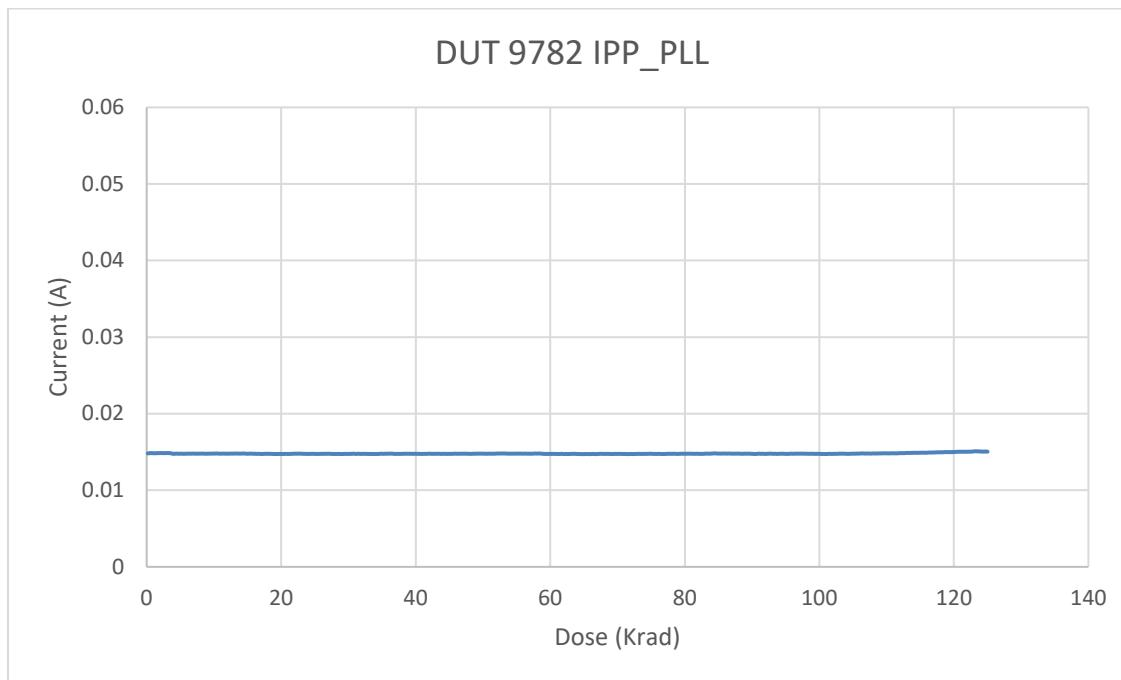
Fig. 20. DUT 9782 charge pump and PLL power supply current ( $I_{PP\_PLL}$ ) versus TID
