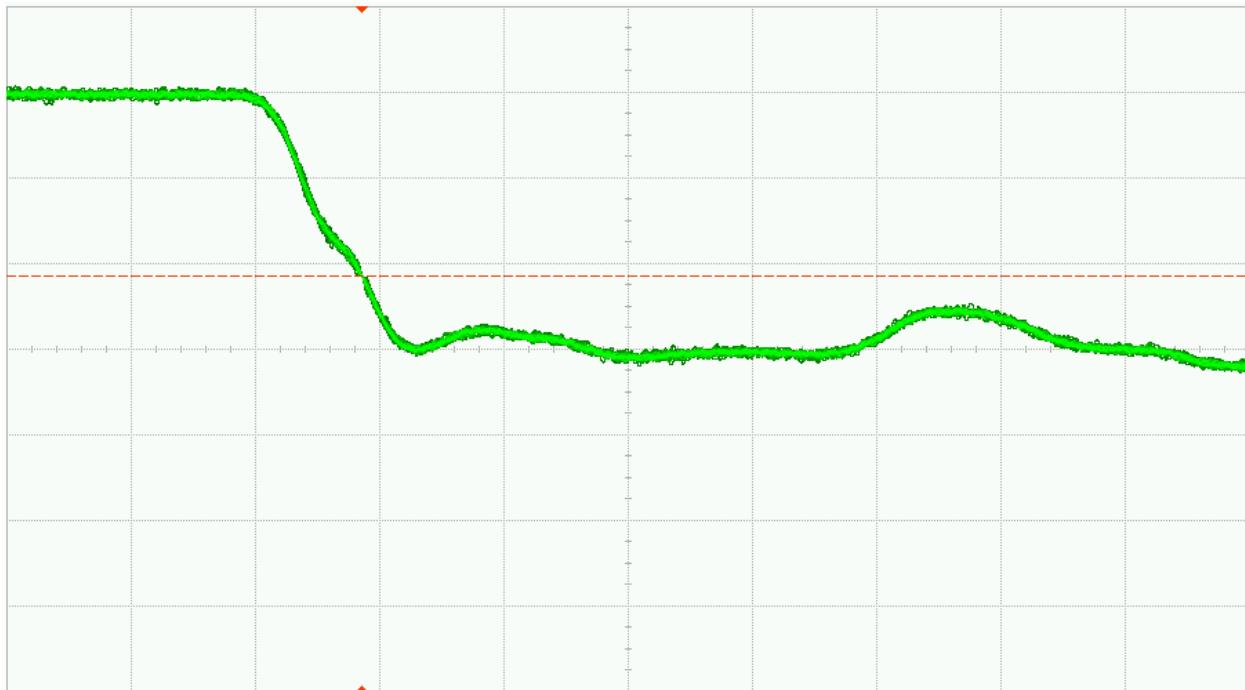
Fig. 33 (a). DUT 9793 pre-irradiation falling edge, abscissa scale is 1V/div and ordinate scale is 2ns/div
