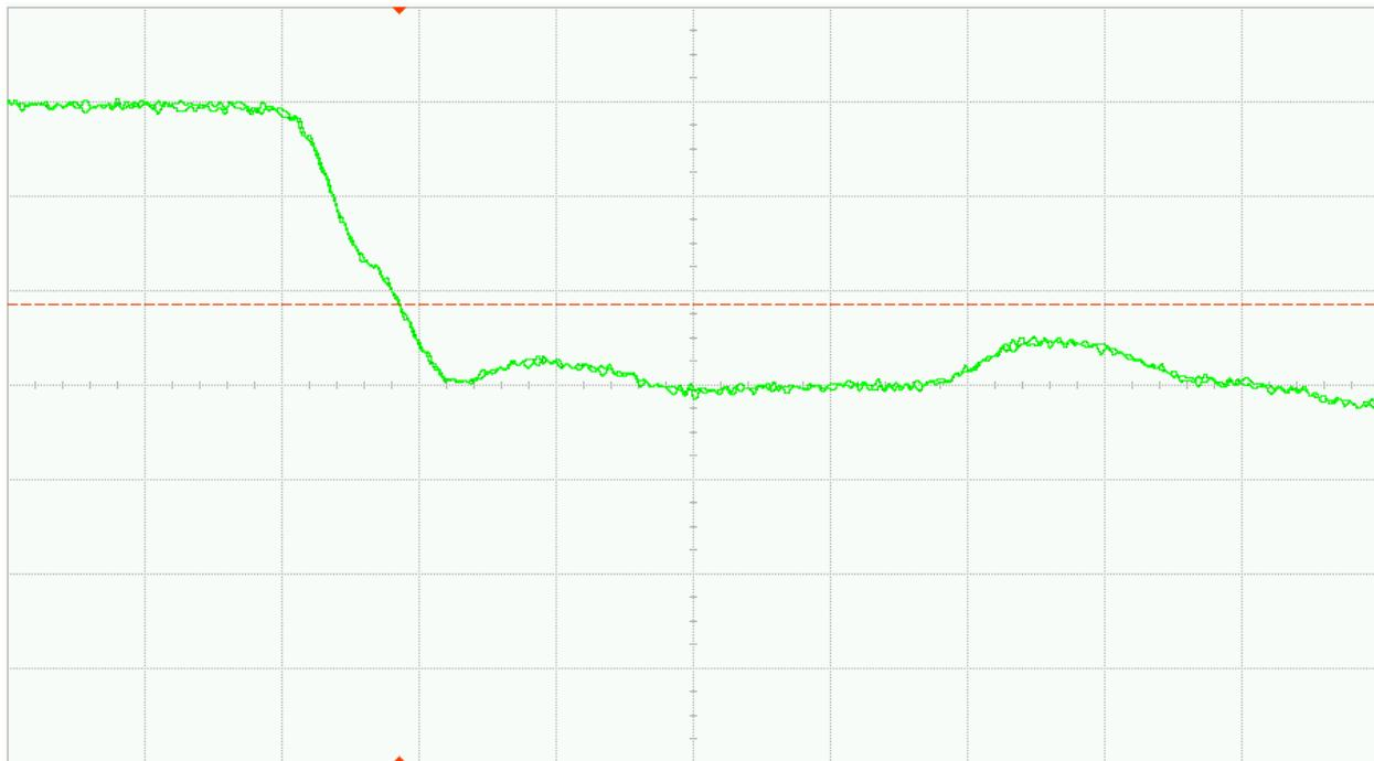
Fig. 35 (a). DUT 9823 pre-irradiation falling edge, abscissa scale is 1V/div and ordinate scale is 2ns/div
