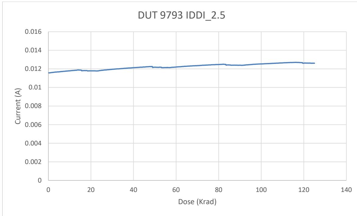
Fig. 9. DUT 9793 I/O bank 2.5V power supply current ( $I_{DDI\_2.5}$ ) versus TID
