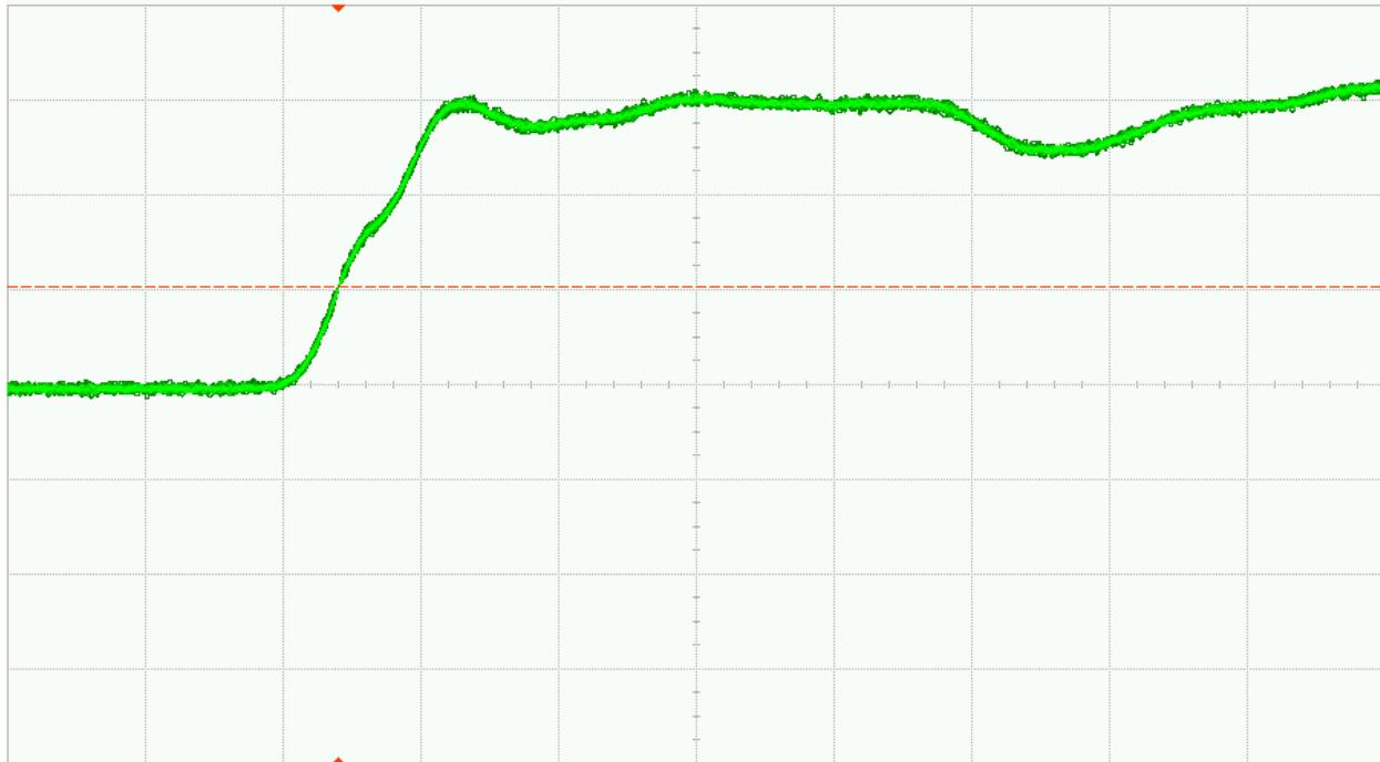
Fig. 31 (a). DUT 9828 pre-irradiation rising edge, abscissa scale is 1V/div and ordinate scale is 2ns/div
