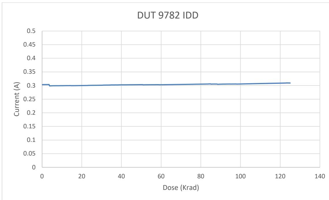
Fig. 2. DUT 9782 core power supply current ( $I_{DD}$ ) versus TID
