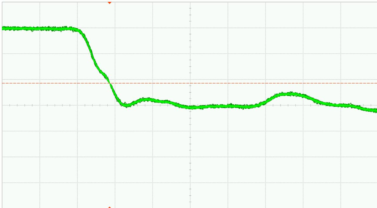
Fig. 34 (a). DUT 9820 pre-irradiation falling edge, abscissa scale is 1V/div and ordinate scale is 2ns/div
