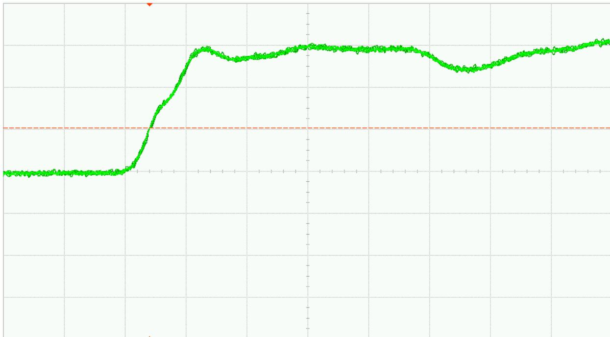
Fig. 28 (b). DUT 9820 post-annealing rising edge, abscissa scale is 1V/div and ordinate scale is 2ns/div
