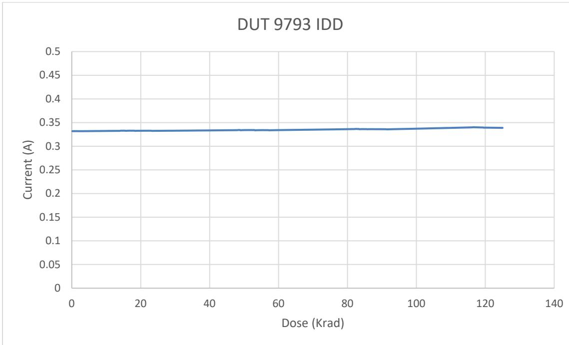
Fig. 3. DUT 9793 core power supply current ( $I_{DD}$ ) versus TID
