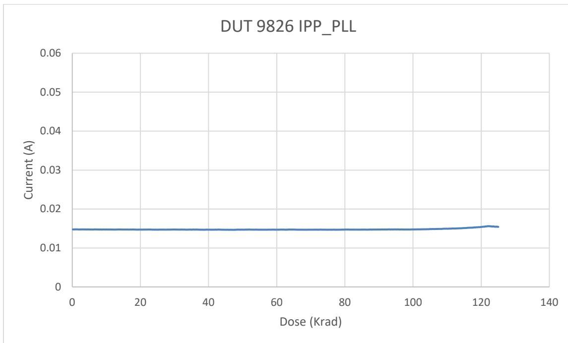
Fig. 24. DUT 9826 charge pump and PLL power supply current ( $I_{PP\_PLL}$ ) versus TID
