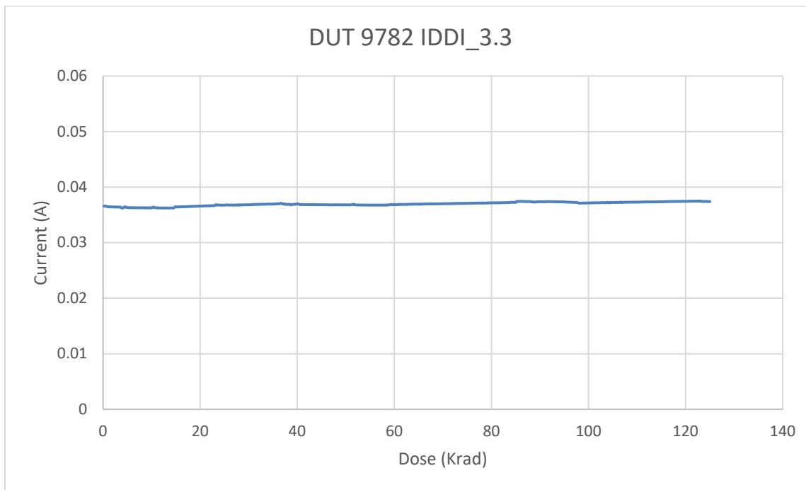
Fig. 14. DUT 9782 I/O bank 3.3V power supply current ( $I_{DDI\_3.3}$ ) versus TID
