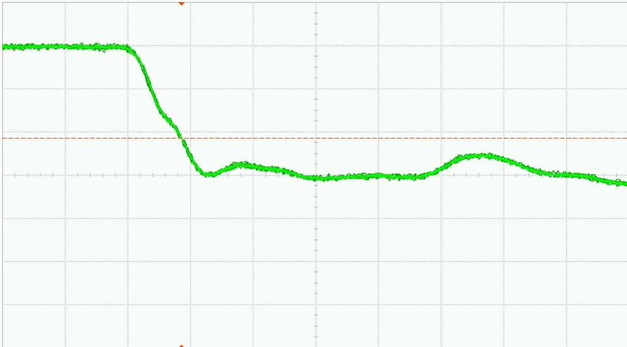
Fig. 37 (a). DUT 9828 pre-irradiation falling edge, abscissa scale is 1V/div and ordinate scale is 2ns/div
