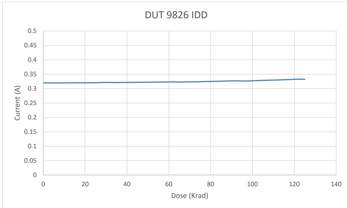
Fig. 6. DUT 9826 core power supply current ( $I_{DD}$ ) versus TID
