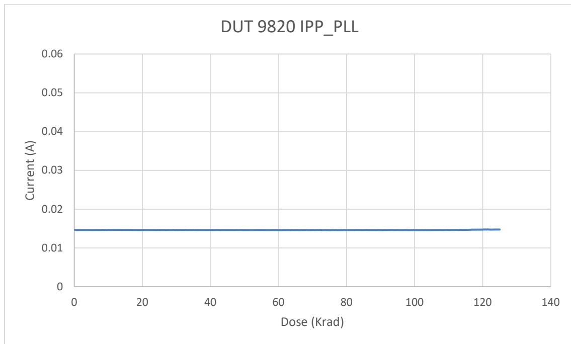
Fig. 22. DUT 9820 charge pump and PLL power supply current ( $I_{PP\_PLL}$ ) versus TID
