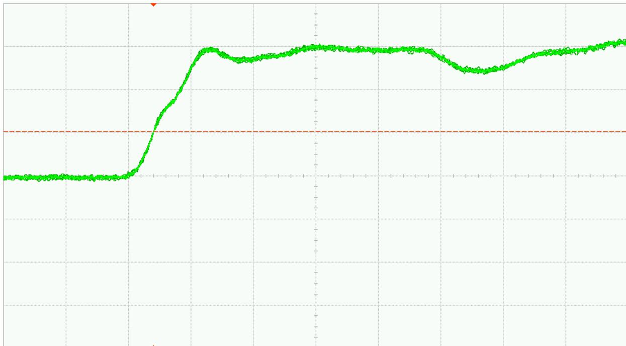
Fig. 30 (b). DUT 9826 post-annealing rising edge, abscissa scale is 1V/div and ordinate scale is 2ns/div
