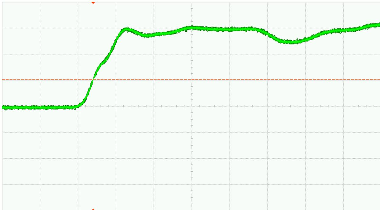
Fig. 28 (a). DUT 9820 pre-irradiation rising edge, abscissa scale is 1V/div and ordinate scale is 2ns/div
