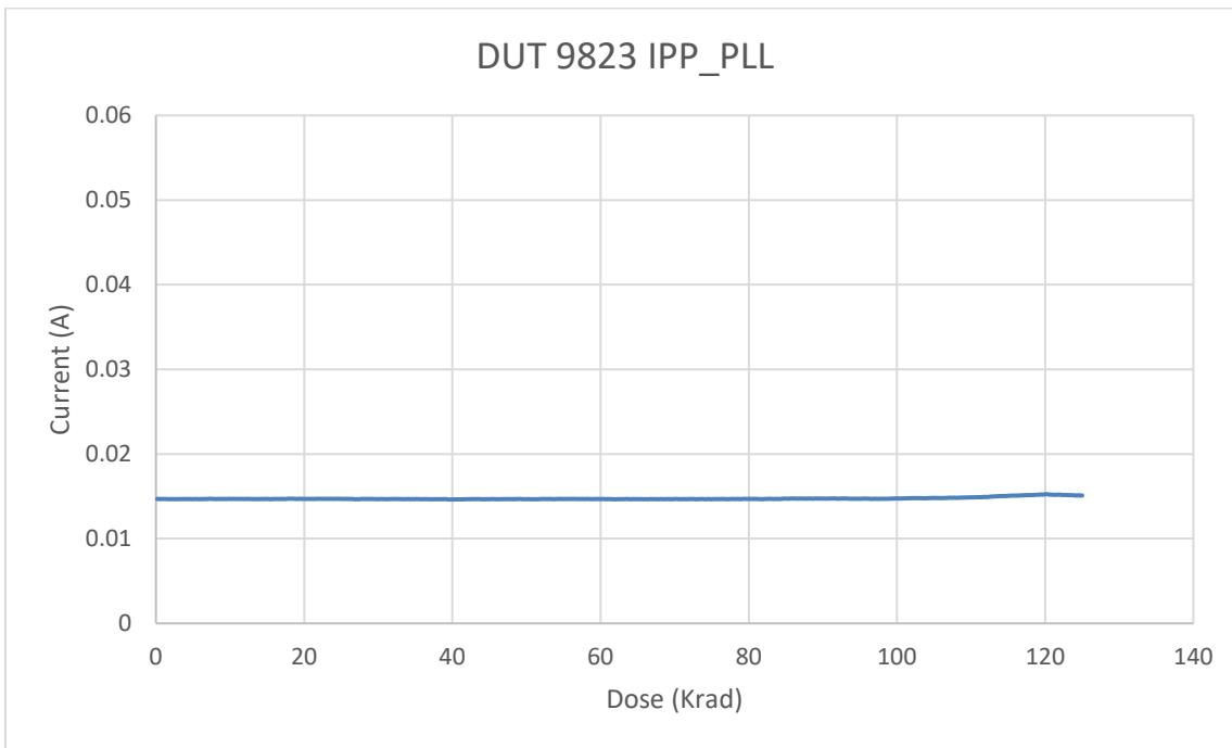
Fig. 23. DUT 9823 charge pump and PLL power supply current ( $I_{PP\_PLL}$ ) versus TID
