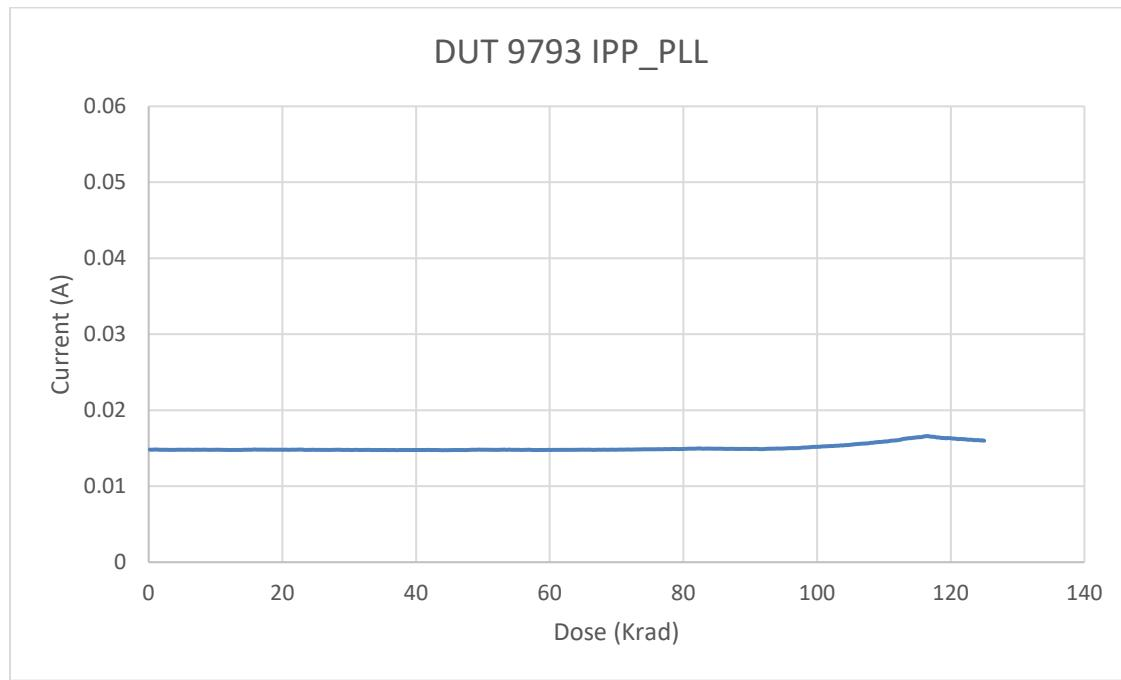
Fig. 21. DUT 9793 charge pump and PLL power supply current ( $I_{PP\_PLL}$ ) versus TID
