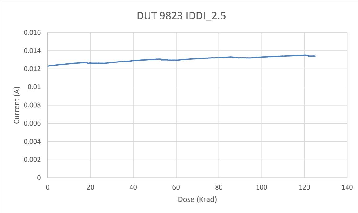
Fig. 11. DUT 9823 I/O bank 2.5V power supply current ( $I_{DDI\_2.5}$ ) versus TID
