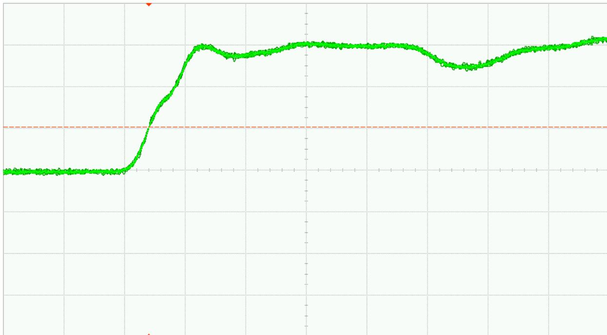
Fig. 27 (a). DUT 9793 pre-irradiation rising edge, abscissa scale is 1V/div and ordinate scale is 2ns/div
