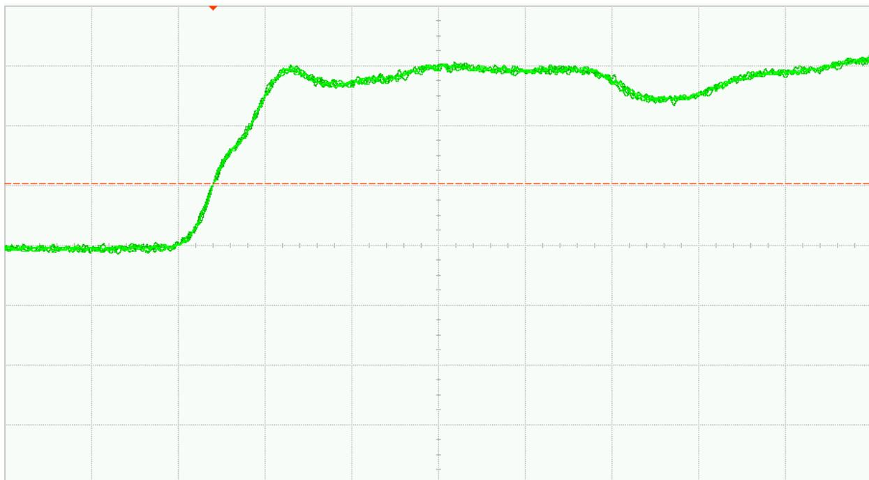
Fig. 27 (b). DUT 9793 post-annealing rising edge, abscissa scale is 1V/div and ordinate scale is 2ns/div
