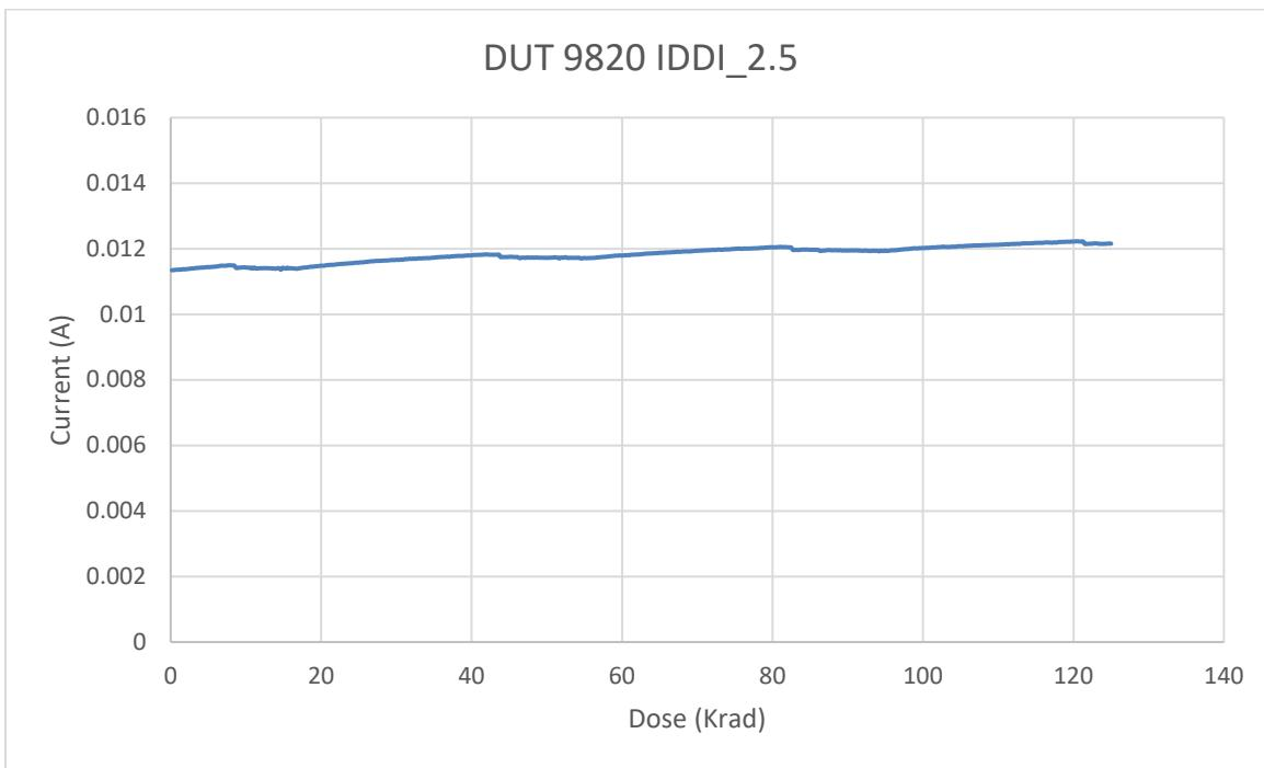
Fig. 10. DUT 9820 I/O bank 2.5V power supply current ( $I_{DDI\_2.5}$ ) versus TID
