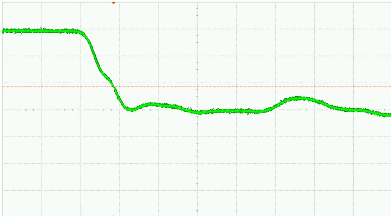
Fig. 34 (b). DUT 9820 post-annealing falling edge, abscissa scale is 1V/div and ordinate scale is 2ns/div
