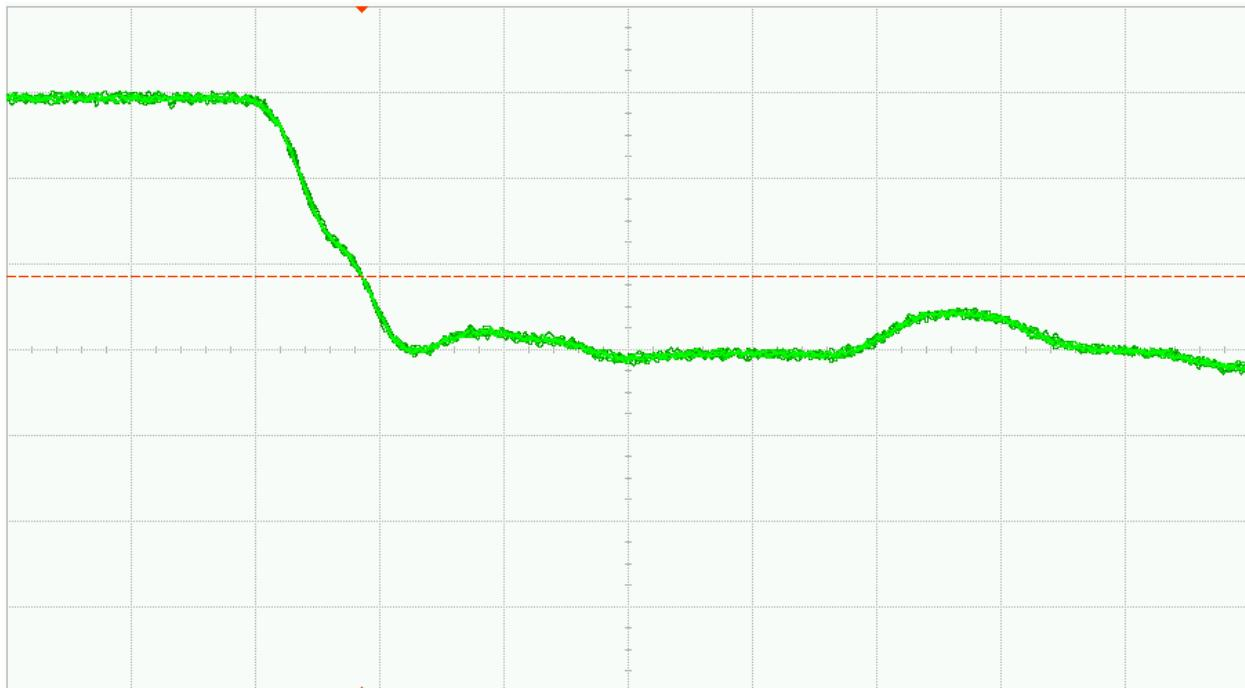
Fig. 33 (b). DUT 9793 post-annealing falling edge, abscissa scale is 1V/div and ordinate scale is 2ns/div
