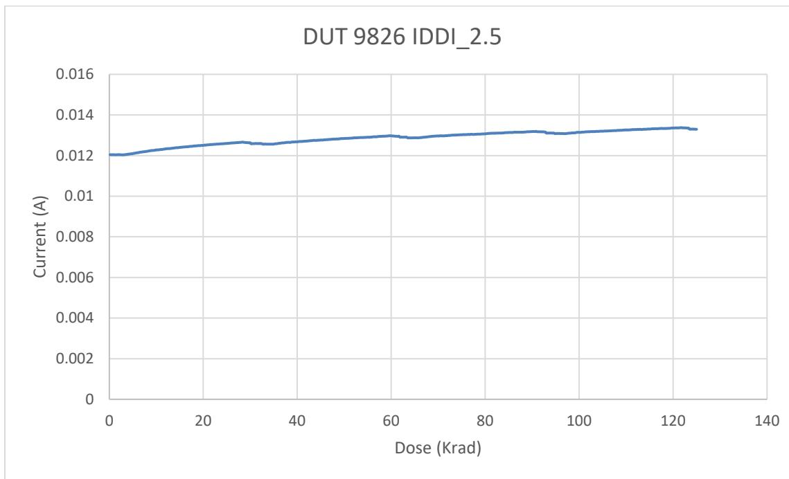
Fig. 12. DUT 9826 I/O bank 2.5V power supply current ( $I_{DDI\_2.5}$ ) versus TID
