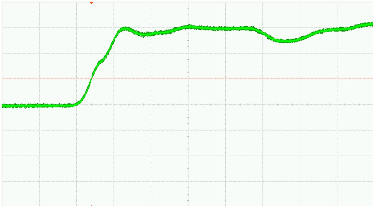
Fig. 30 (a). DUT 9826 pre-irradiation rising edge, abscissa scale is 1V/div and ordinate scale is 2ns/div
