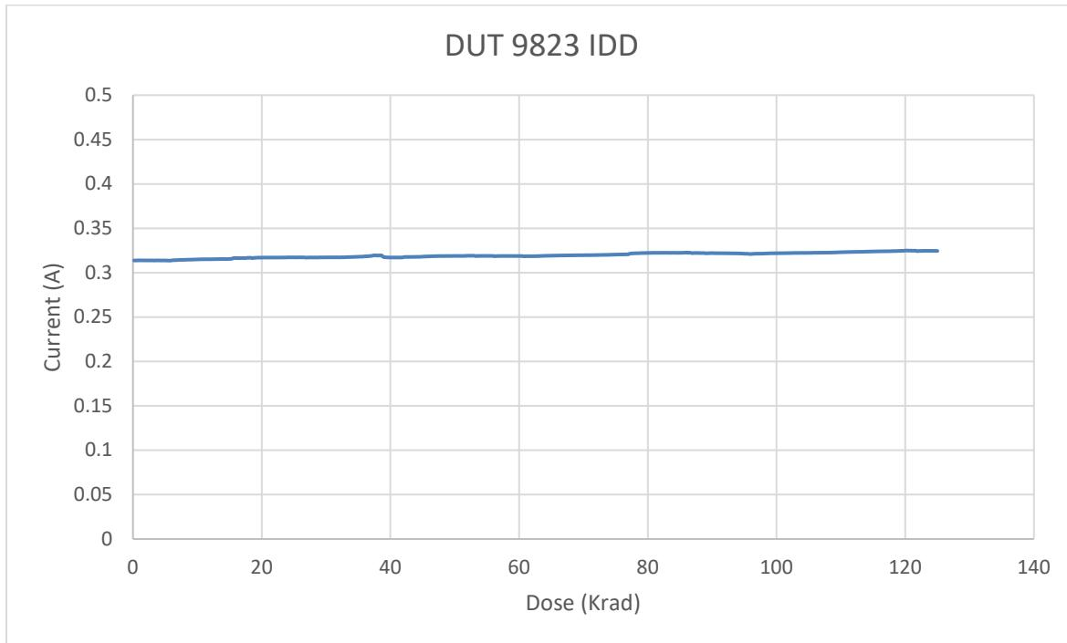
Fig. 5. DUT 9823 core power supply current ( $I_{DD}$ ) versus TID
