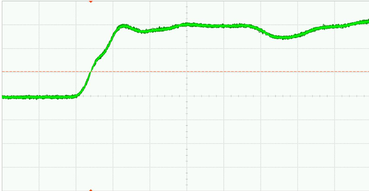
Fig. 26 (a). DUT 9782 pre-irradiation rising edge, abscissa scale is 1V/div and ordinate scale is 2ns/div
