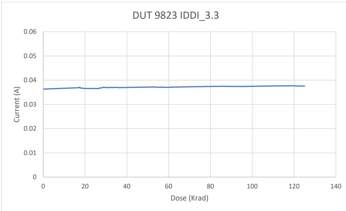
Fig. 17. DUT 9823 I/O bank 3.3V power supply current ( $I_{DDI\_3.3}$ ) versus TID
