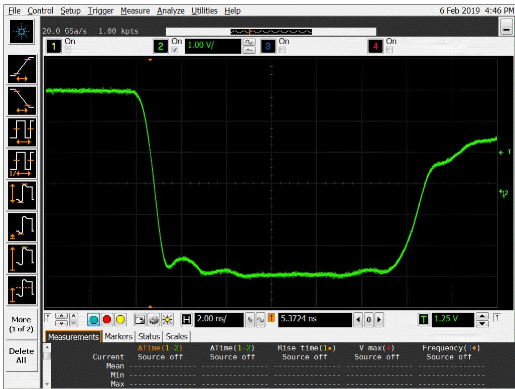
**Figure 20b DUT 8729 Post-Annealing Falling Edge**
