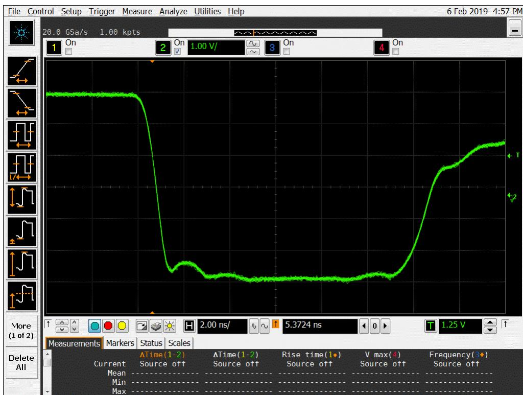
**Figure 16b DUT 8748 Post-Annealing Falling Edge**
