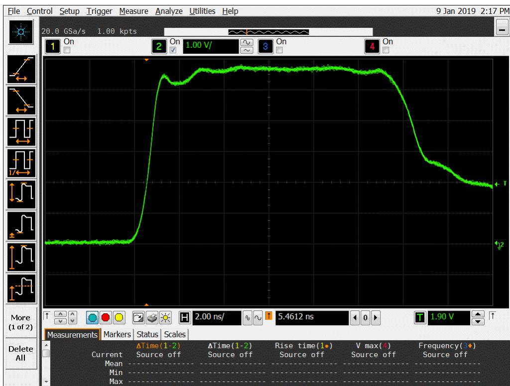
**Figure 10a DUT 8748 Pre-Irradiation Rising Edge**
