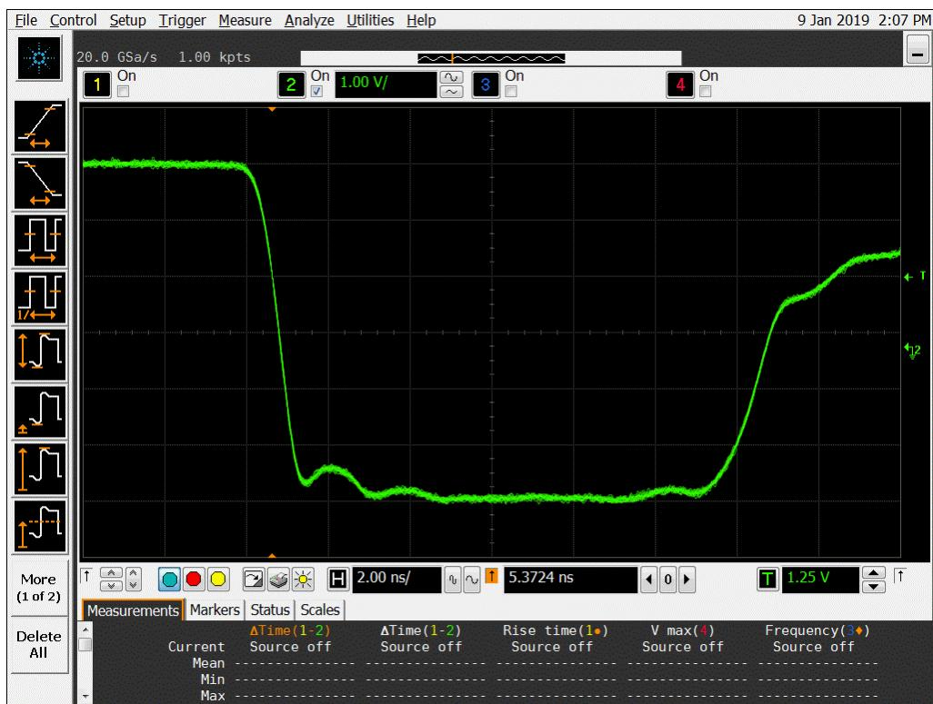
**Figure 20a DUT 8729 Pre-Irradiation Falling Edge**
