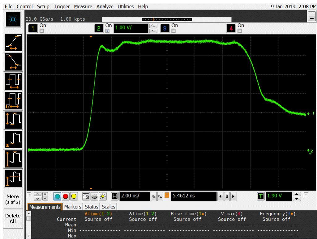
Figure 14a DUT 8729 Pre-Irradiation Rising Edge
