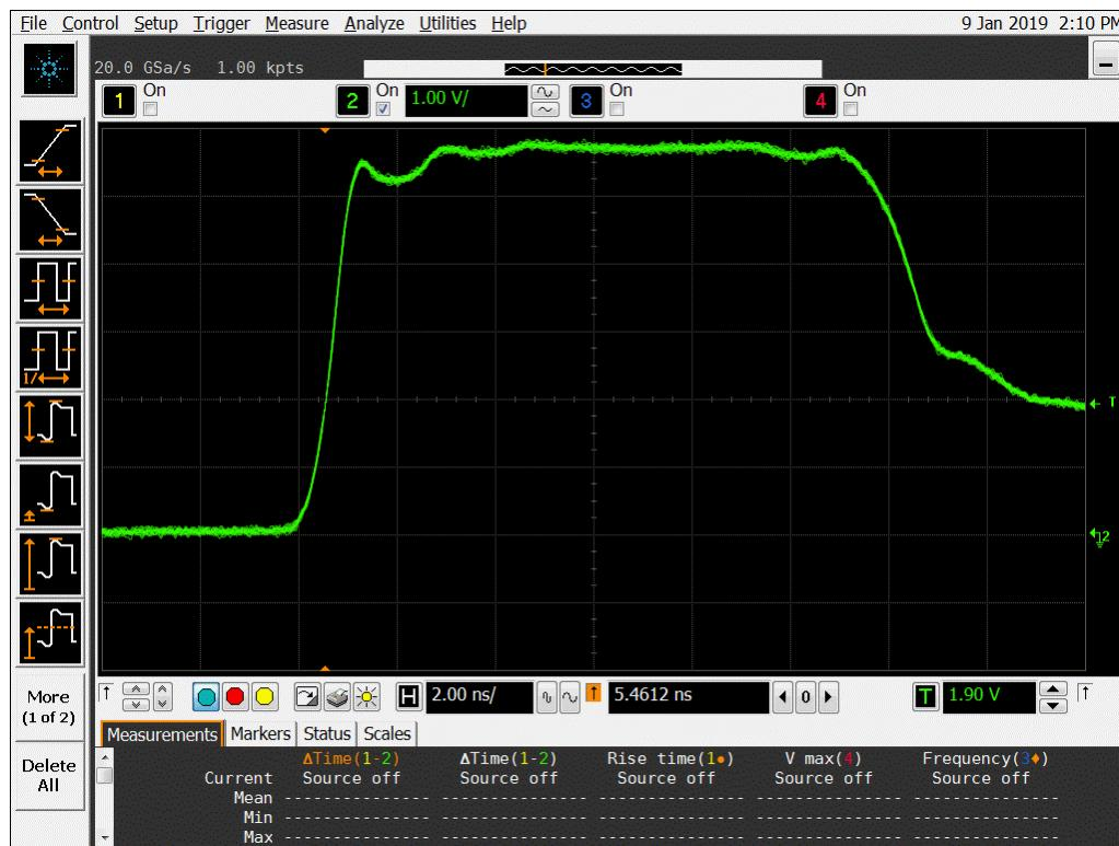
**Figure 11a DUT 8731 Pre-Radiation Rising Edge**
