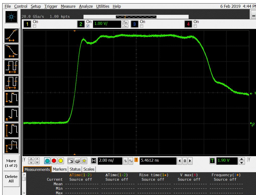
**Figure 13b DUT 8714 Post-Annealing Rising Edge**
