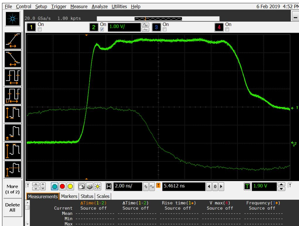
**Figure 12b DUT 8744 Post-Annealing Rising Edge**
