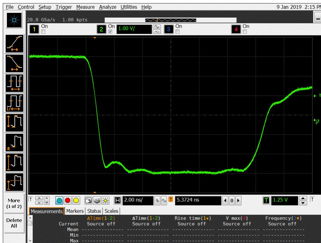
**Figure 15a DUT 8746 Pre-Radiation Falling Edge**
