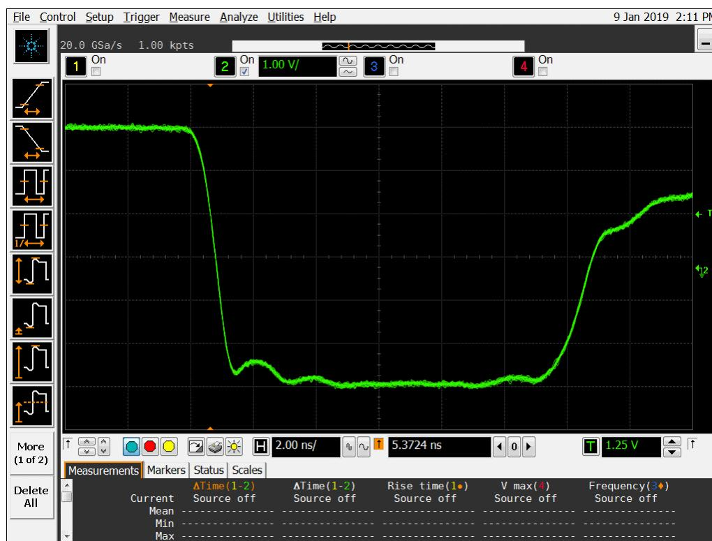
**Figure 17a DUT 8731 Pre-Irradiation Falling Edge**
