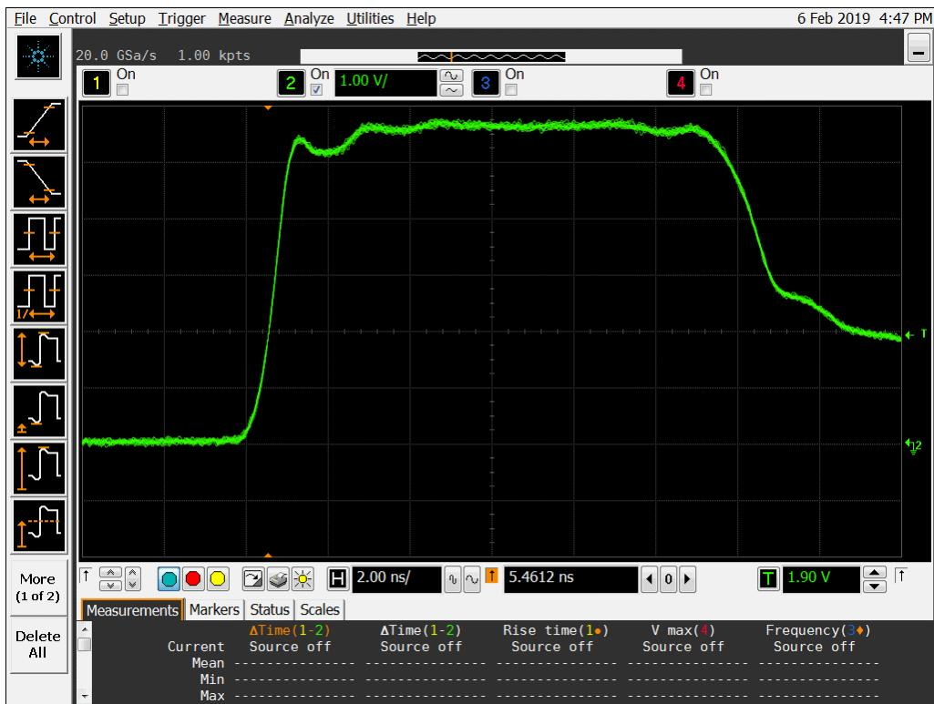
Figure 14b DUT 8729 Post-Annealing Rising Edge
