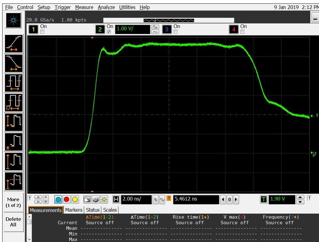
**Figure 12a DUT 8744 Pre-Irradiation Rising Edge**
