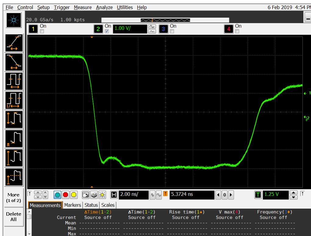
**Figure 15b DUT 8746 Post-Annealing Falling Edge**
