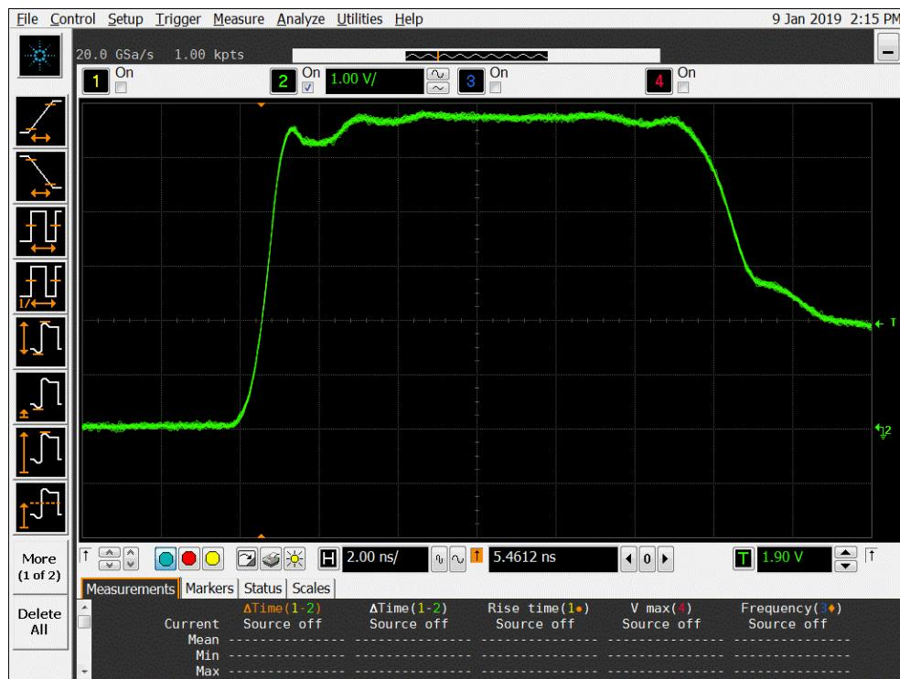
Figure 9a DUT 8746 Pre-Irradiation Rising Edge
