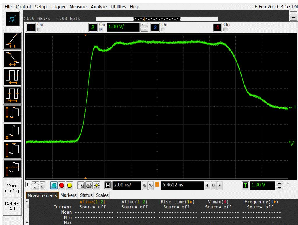
**Figure 10b DUT 8748 Post-Annealing Rising Edge**
