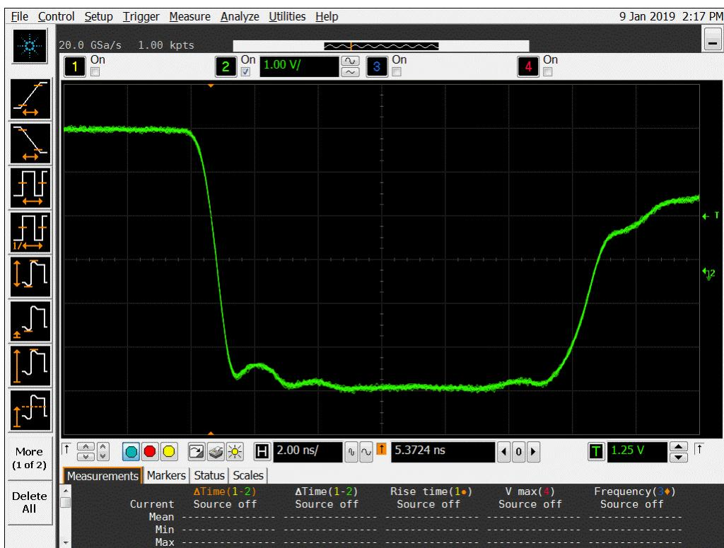
**Figure 16a DUT 8748 Pre-Irradiation Falling Edge**
