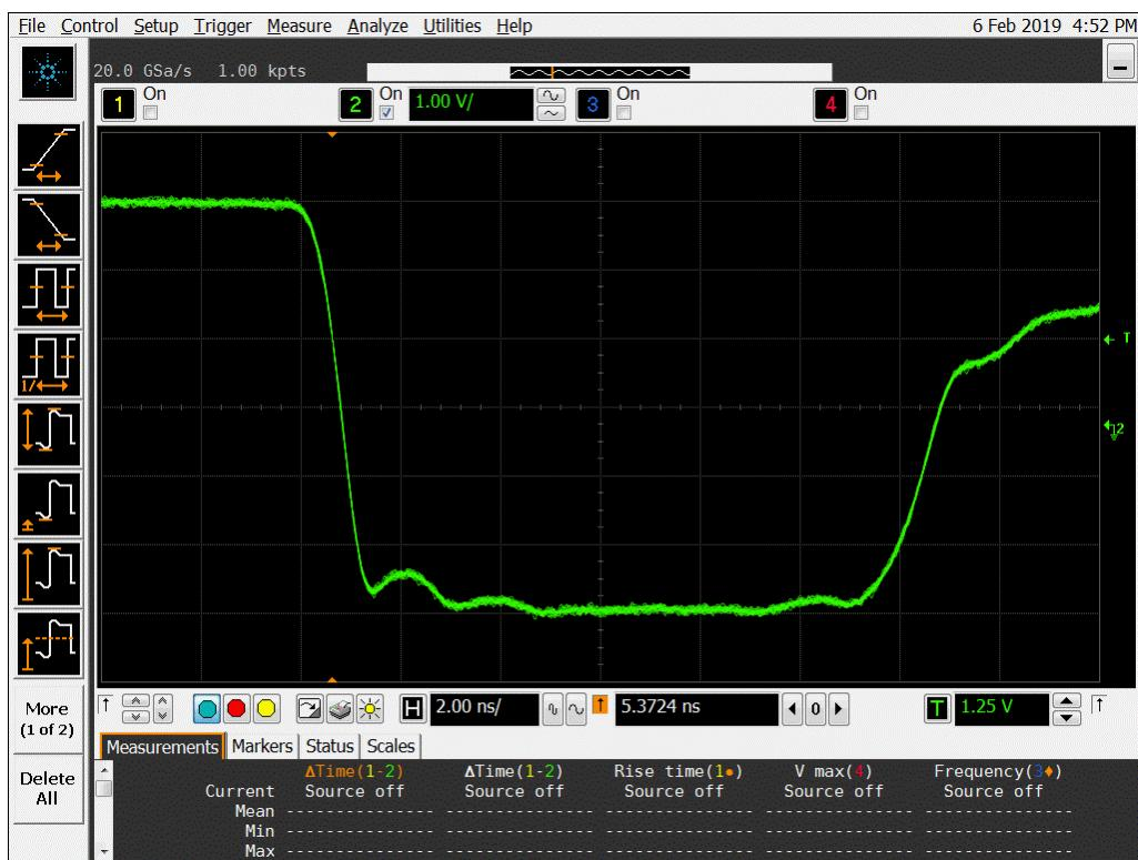
**Figure 18b DUT 8744 Post-Annealing Falling Edge**
