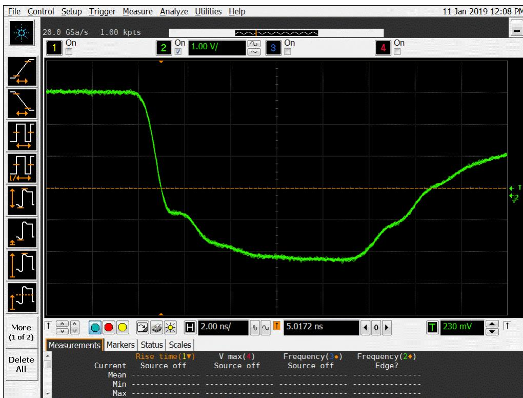
Figure 11a DUT 7967 Pre-Irradiation Falling Edge.
