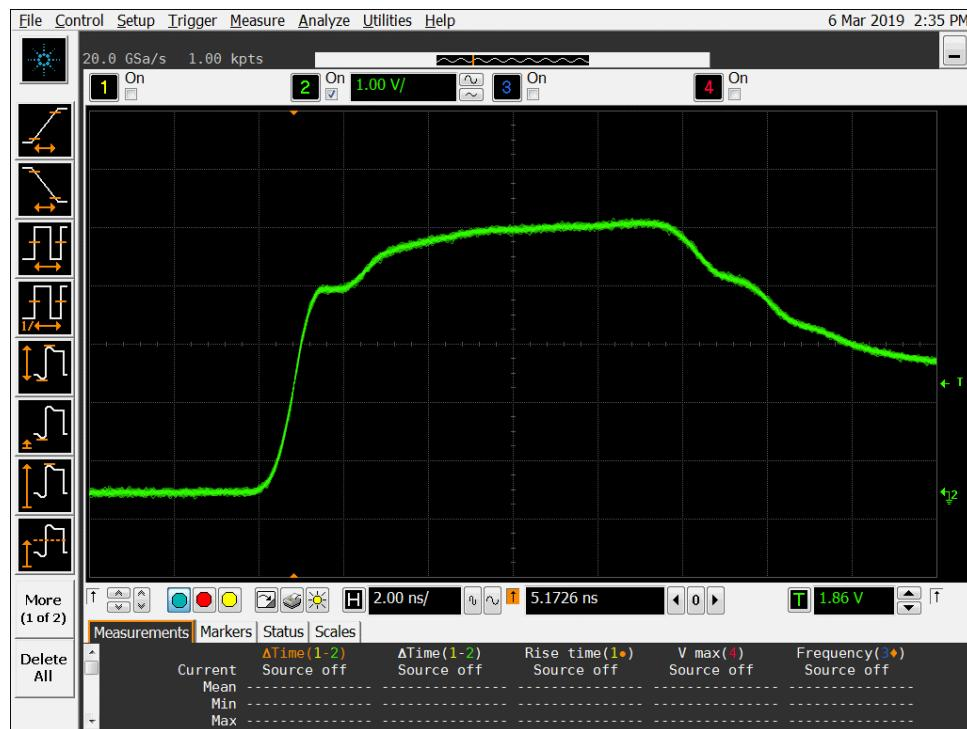
Figure 6b DUT 7950 Post-Annealing Rising Edge.
