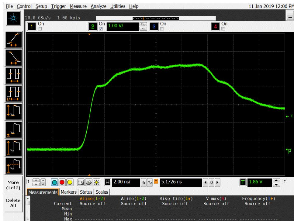
Figure 6a DUT 7950 Pre-Irradiation Rising Edge.
