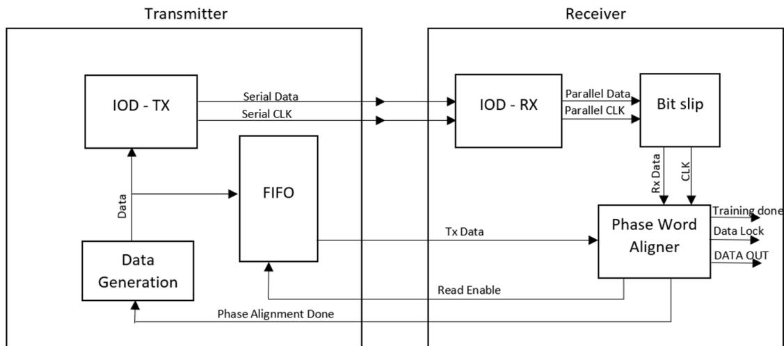
The LVDS 7:1 transmit and receive blocks perform the following functions:
