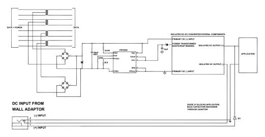
CONFIGURATION #3: SOURCE CONNECTED TO APPLICATION'S SUPPLY RAILS
