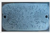
Figure 2-3. Grease on the Module After Disassembling
