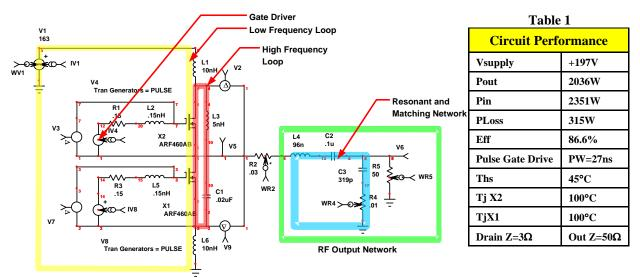
Figure 1. N - N Channel Half Bridge
