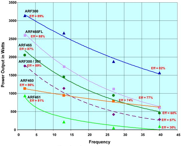
Figure 2. RF Output Power vs. Frequency
